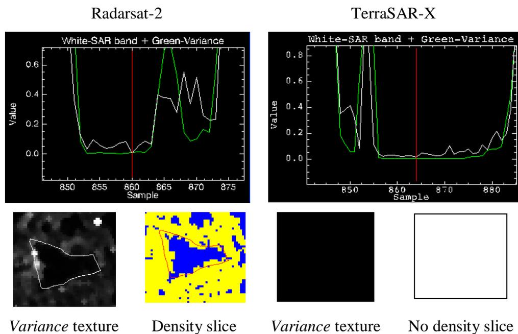
Figure 6.16: Reflectance profiles of occurrence *variance* texture measure with extracted texture scene for Radarsat-2 HH and TerraSAR-X images (note that there is no output texture signature for the TerraSAR-X image and accordingly no density slice).
