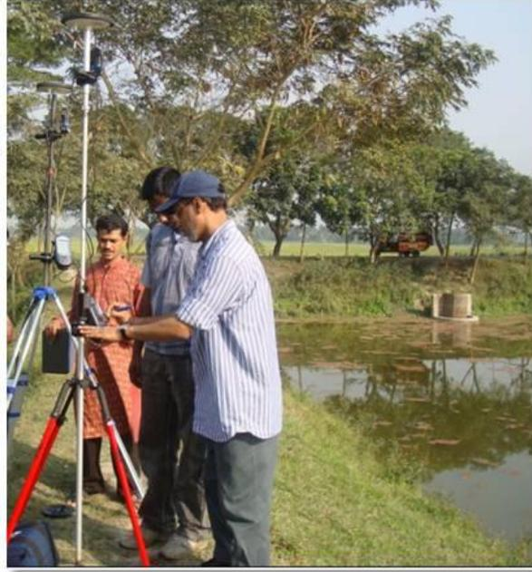
Figure 5.5: Setting up the ProMark3 equipment (base and rover) during fieldwork in Bangladesh.
