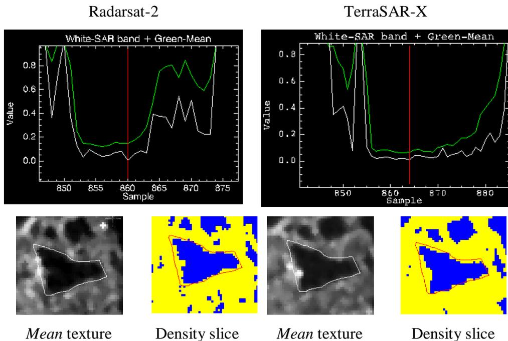
Figure 6.15: Reflectance profiles of occurrence *mean* texture measure for Radarsat-2 and TerraSAR-X HH images with extracted texture scenes smoothed by median  $3 \times 3$  window, along with density slice scenes.
