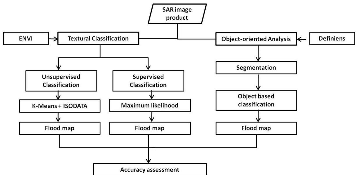
Figure 5.11: General methodology flowchart for mapping flood.
