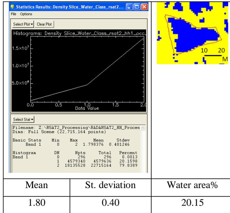
Figure 7.5: Statistical results of density slicing for water class with *occurrence mean* variable - Radarsat-2 HH.
