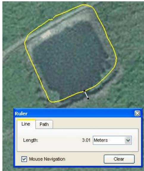
Figure 6.8: Distance of distortion of a water body extracted from Google Earth, 2010, overlaid with dGPS data. Note the distortion measured approximately 3 metres.
