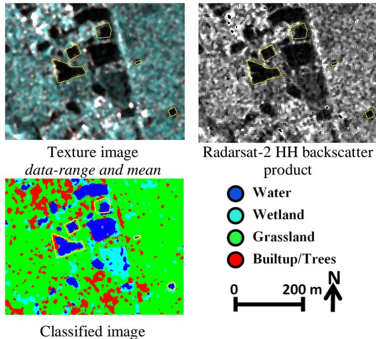
Figure 7.12: Supervised classification of *occurrence data-range and mean* texture image for Radarsat-2 HH overlaid with dGPS data compared to the original SAR product and the texture image; maps shown here and subsequent maps cover a small portion of the study area.
