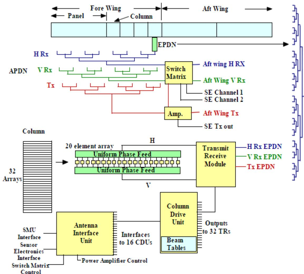
Radarsat-2 antenna subsystem (adapted from Livingstone et al., 2005)
