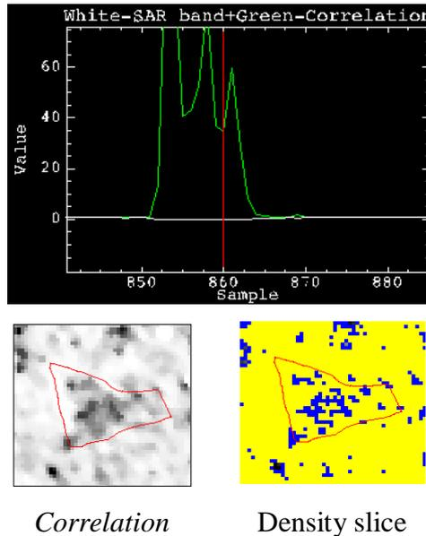
Figure 6.26: Reflectance profile of co-occurrence *correlation* texture measure for the Radarsat-2 HH image with extracted texture scene, and density slice in the ranges  $-25$  to  $-7$  (blue) and  $-7$  to  $4$  (yellow).
