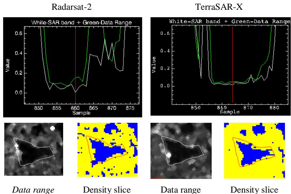
Figure 6.14: Reflectance profiles of occurrence *data range* texture measure with extracted texture scenes smoothed by median  $3 \times 3$  window, along with density sliced scenes for Radarsat-2 and TerraSAR-X HH images.
