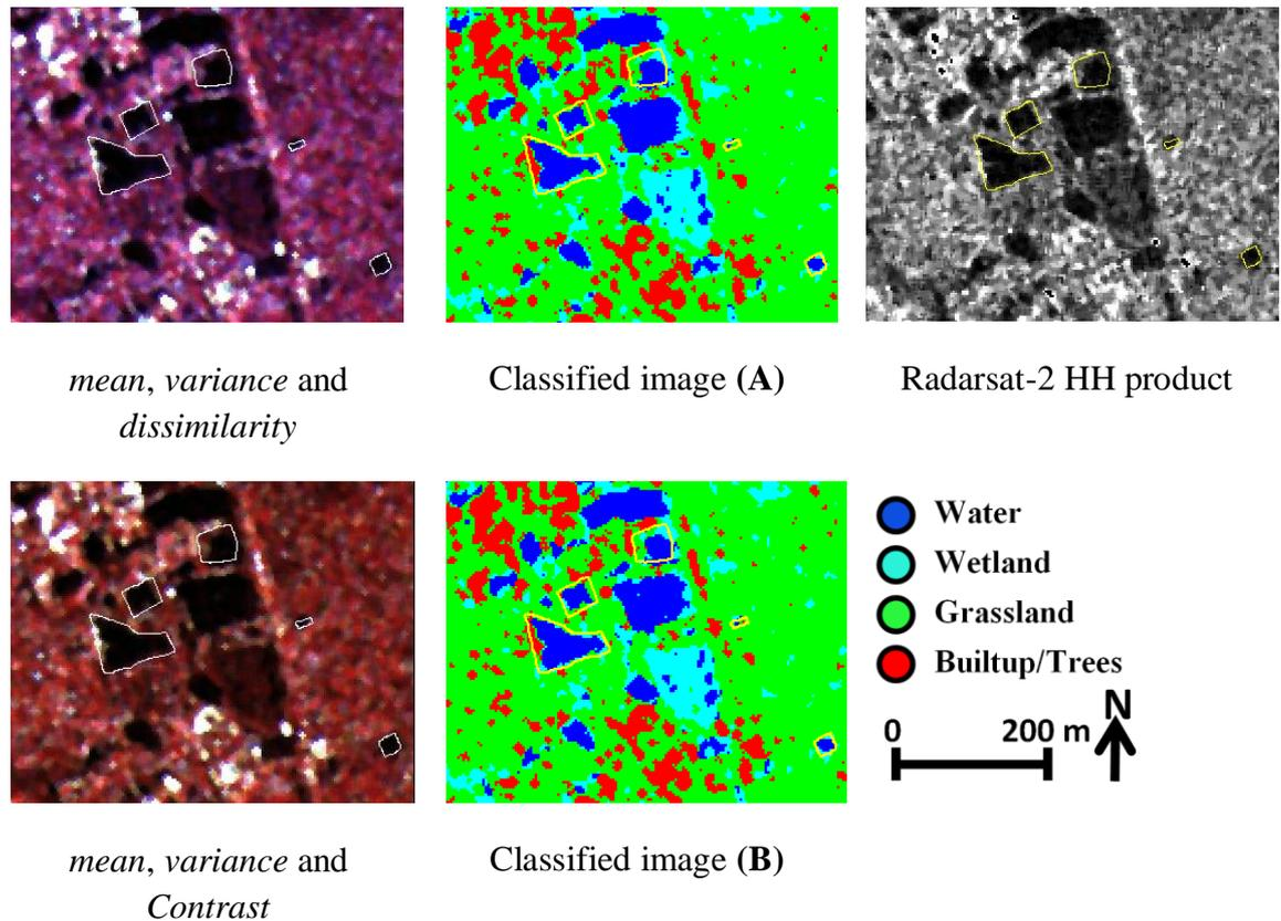
Figure 7.14: Supervised classification of Radarsat-2 HH produced after applying co-occurrence variables of (A) *mean, variance and dissimilarity*, and (B) *mean, variance and contrast* overlaid with dGPS data
