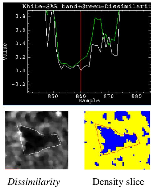
Figure 6.23: Reflectance profile of co-occurrence *dissimilarity* texture measure filter for the Radarsat-2 HH image with extracted texture scene, and density slice in the ranges 0.0–2.5 (blue) and 2.5–39 (yellow).
