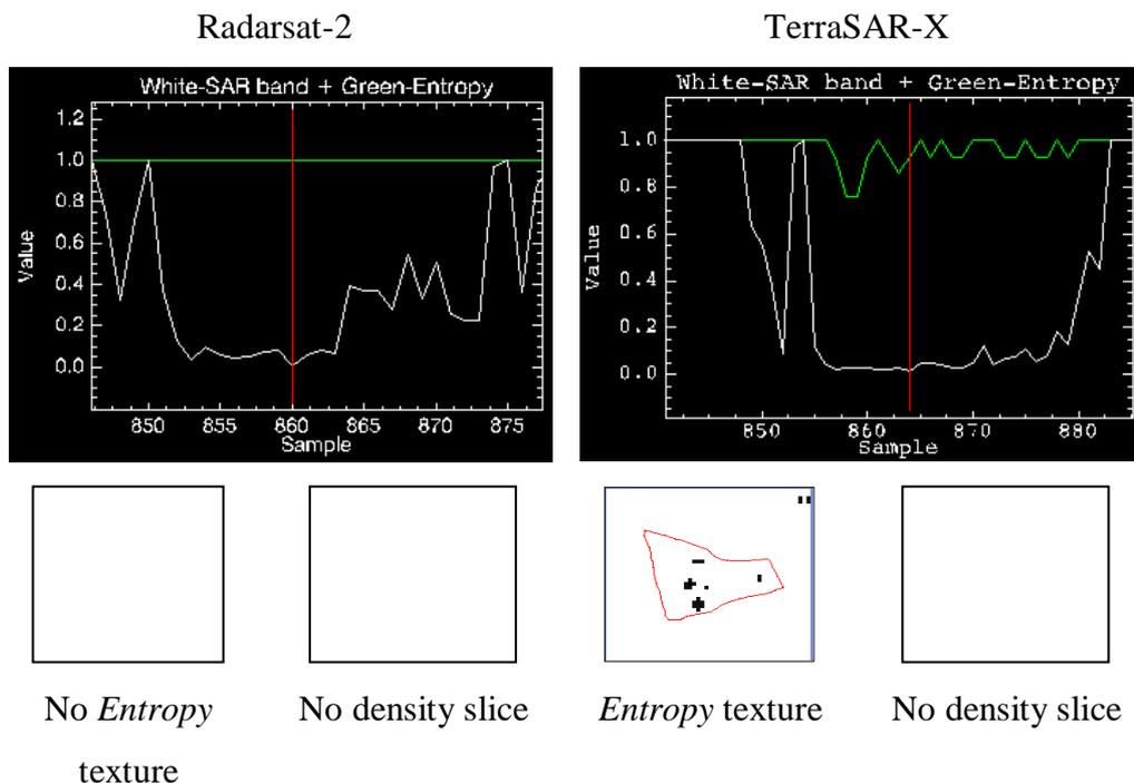
Figure 6.17: Reflectance profiles of occurrence *entropy* texture measure for Radarsat-2 HH and TerraSAR-X HH images (note that there is no output texture signature other than a solid white colour, and as a result there is no density slice).
