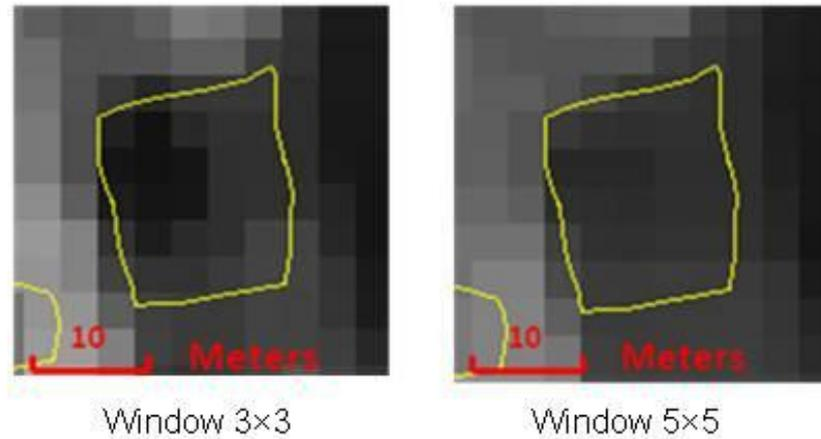
Figure 6.12: A comparison between 3×3 and 5×5 window sizes of enhanced median filter with an area of 238m<sup>2</sup> – note that the 5×5 window size shows less intensity.
