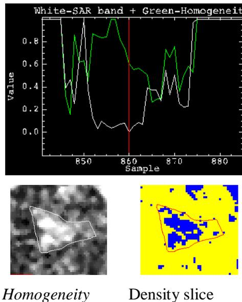
Figure 6.21: Reflectance profile of co-occurrence *homogeneity* texture measure for the Radarsat-2 HH image with extracted texture scene, and density slice in the ranges 0.0–0.4 (yellow) and 0.4–0.8 (blue).
