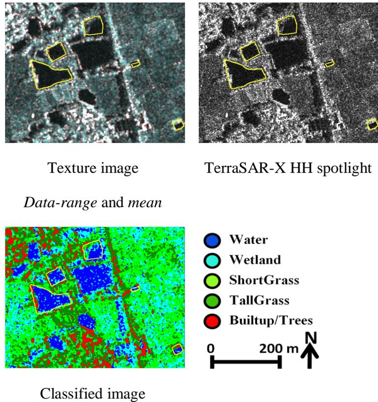
Figure 7.17: Supervised classification of *occurrence data-range and mean* texture image for TerraSAR-X HH spotlight overlaid with dGPS reference data in yellow compared to the original SAR product and the texture image
