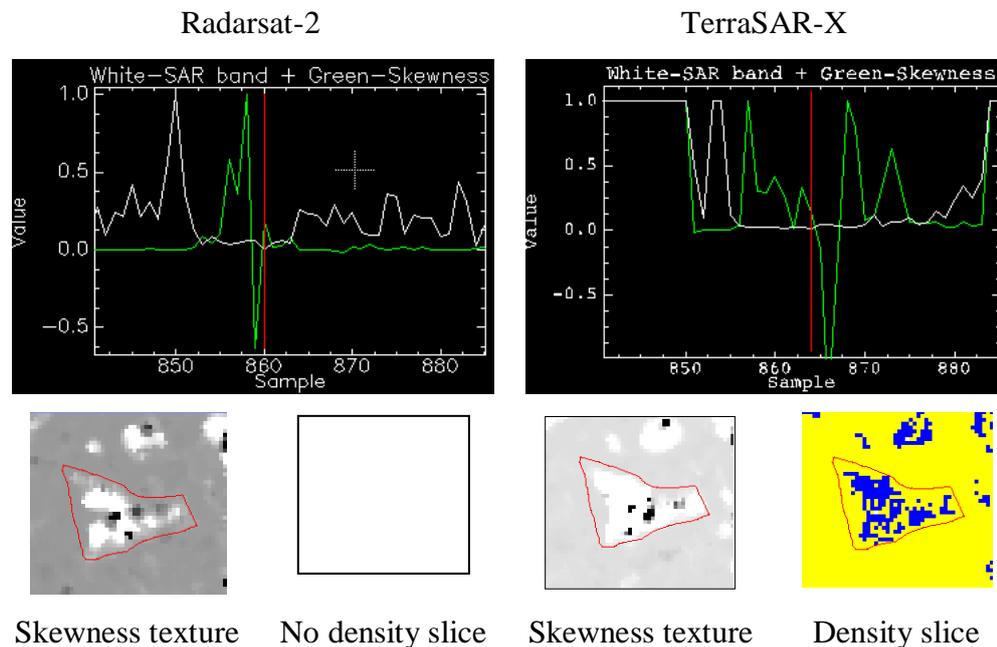
Figure 6.18: Reflectance profiles of occurrence *skewness* texture measure with extracted texture scenes for Radarsat-2 HH and TerraSAR-X images (note that there is no density slice range for the Radarsat-2 HH texture image since the value range is  $-0.00$  to  $0.00$ ).
