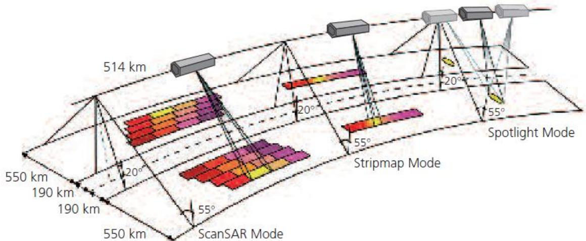
Figure 3.12: TerraSAR-X SAR modes of operation (source: DLR, 2009).
