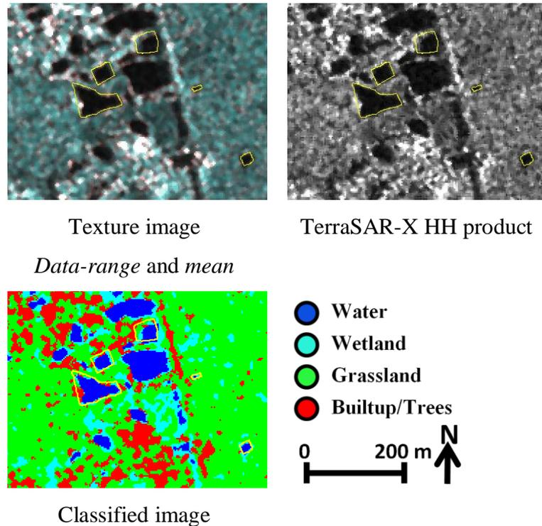
Figure 7.15: Supervised classification of *occurrence data-range* and *mean* texture image for TerraSAR-X HH Stripmap overlaid with dGPS data compared to the original SAR product and the texture image
