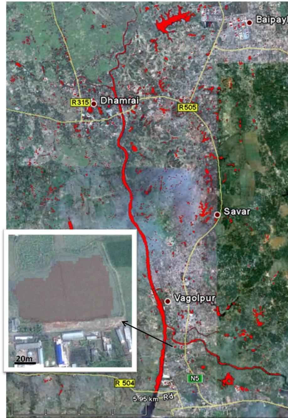
Figure 8.9: An example of  *water*  class layer of the study area (in red) produced from the developed methods and mashup in the Google Earth. Note the water body zoomed in (the white rectangle) showing the water layer in transparent red colour presenting the ability of the proposed water area mapping method.
