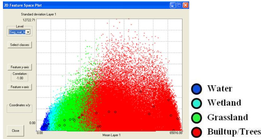
Figure 7.23: Checking signatures separability using Definiens 2D feature space plot for training classes
