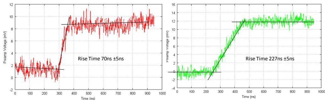
Fig 5-4 Preamplifier traces captured from the XR-100T detector illuminated by a  $^{57}\text{Co}$  source. The traces on the left and right of the figure represent the fastest and slowest rise times observed from this detector respectively.
