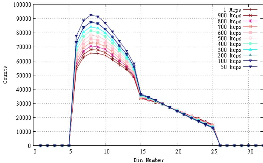
Fig 4-15 Spectra produced by pulse height detection Algorithm 3 for various input count rates using a data set of one million random events from 30 keV to 125 keV. Here discarded counts have been added back into the spectrum by reference to the non piled up output spectrum.
