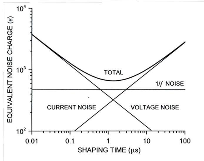
Fig 2-8 Diagram showing ENC as a function of shaping time<sup>22</sup> for a typical detector system as outlined in Fig 2-7.
