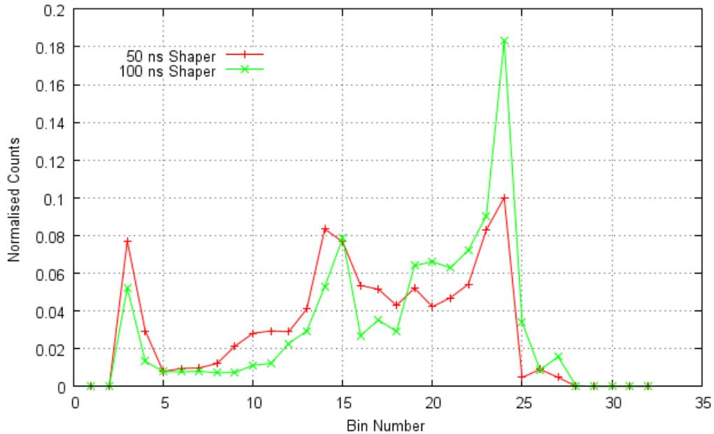
Fig 5-5  $^{57}\text{Co}$  spectra from an XR-100T detector with various shaping times. MCA spectrum captured using an FPGA programmed with Algorithm 1<sup>v</sup>.
