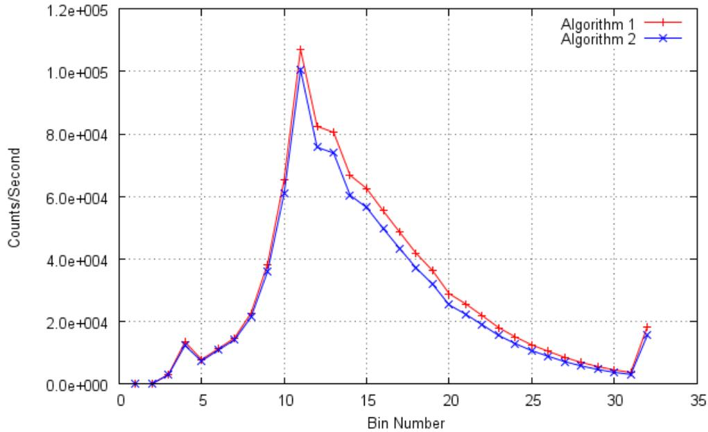
Fig 5-9 Graph showing the  $I_0$  spectra acquired using Algorithms 1 and 2 with a beam current of  $0.303\text{ mA}$  and a tube voltage of  $160\text{ kV}$  using a CR-200-50ns shaper. The acquisition time for these spectra was 160 seconds.
