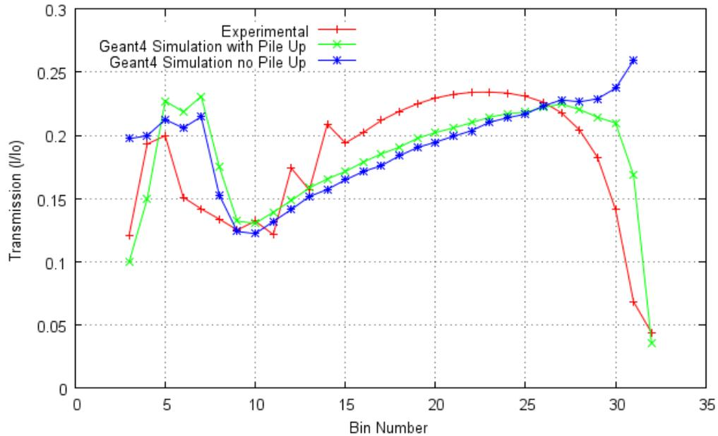
Fig 6-6 Graph showing the transmission spectra from an  $I/I_0$  measurement of a 1000 ml PET bottle of water. The experimental data was collected by use of the FPGA implementation of Algorithm 2. The modelled transmissions are from a simulation with and without pulse pile up consideration.
