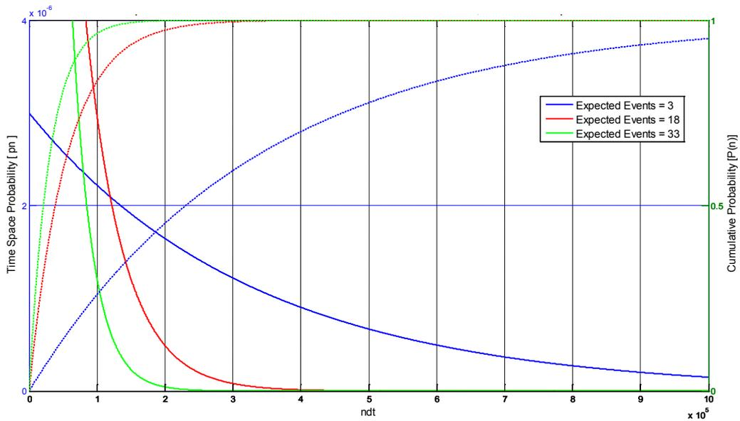
Fig 4-1 Time interval (solid line) and cumulative (dashed line) probabilities as a function of time interval,  $n\delta t$ . Here the expected total count is 99 in a total time,  $N\delta t = 1 \text{ ms}$  where  $N = 1 \times 10^6$  and  $\delta t = 1 \text{ ns}$ .
