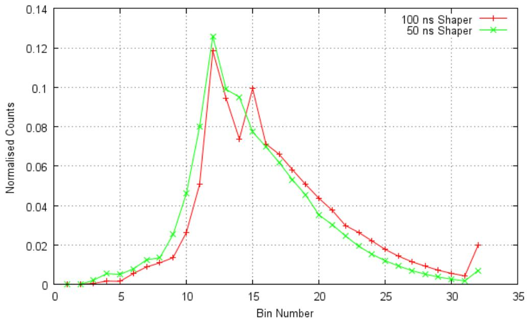
Fig 5-6 Graph showing the x-ray spectra acquired using Algorithm 1 on FPGA. Shaping times of  $100\text{ ns}$  and  $50\text{ ns}$  were selected. The x-ray beam current was  $0.104\text{ mA}$  and the tube voltage was  $160\text{ kV}$ .
