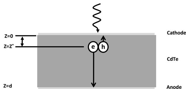
Fig 7-2 Diagram showing the creation of an electron-hole pair at a distance  $z^*$  from the cathode. Interactions at  $z > z^*$  suffer ballistic deficit effects due to the longer collection time of the hole signal.
