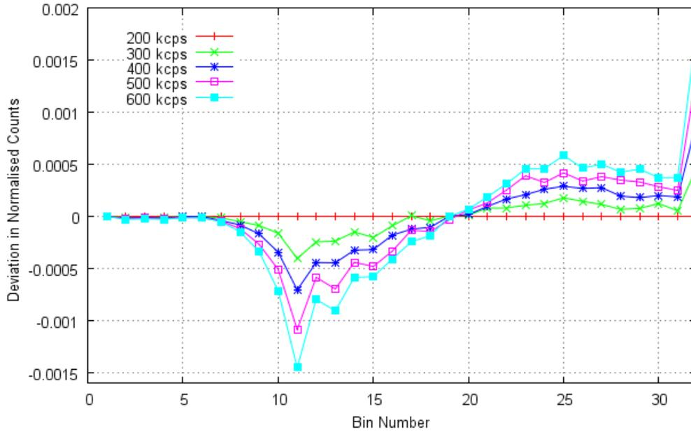
Fig 7-20 Deviations plot of normalised  $I_c$  counts as a function of bin number for various count rates. Here the deviation is with respect to a rate of 200  $kcps$  measured in  $I_c$  and the counts are taken from all locations within the HW plot. The rate dependant deviation in counts is as discussed in Chapter 4 and due to pulse pile up.
