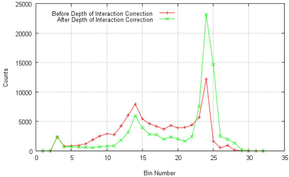
Fig 7-16 Graph showing the  $^{57}\text{Co}$  spectrum before and after depth of interaction correction. The data here was taken using an FPGA with a  $128 \times 32$  value lookup table which was used to reassign pulses to the correct bin.
