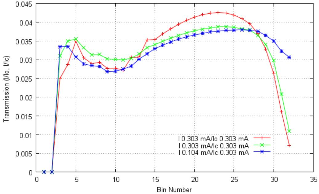
Fig 5-16 Transmission plots under various beam current and normalisation conditions showing the reduction in rollover which occurs when the count rate in the  $I$  and  $I_0$  (or  $I_c$ ) spectra are equalised.
