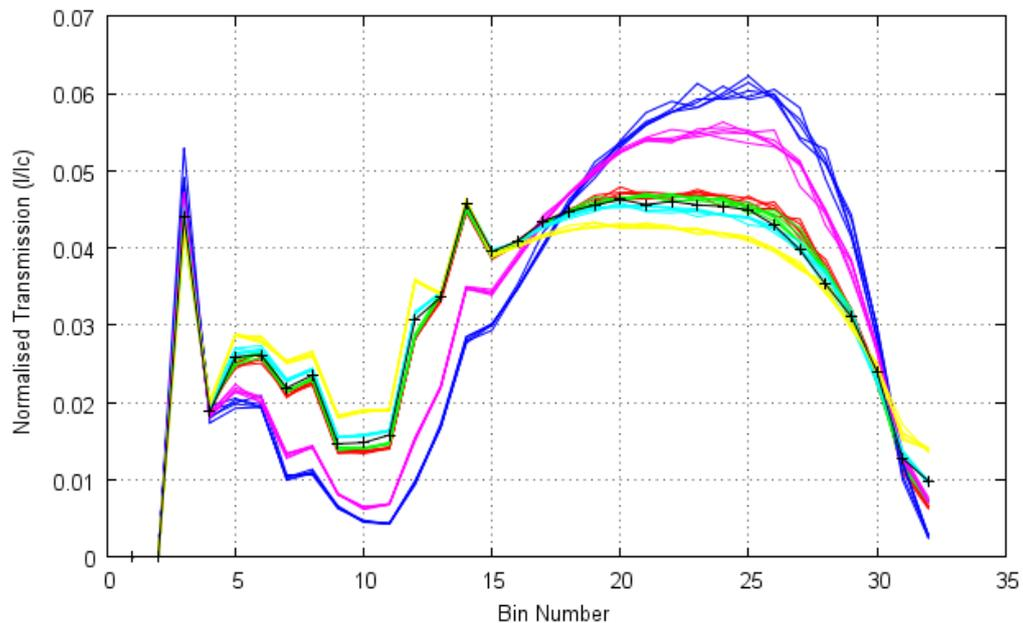
Fig 5-18 Graph showing  $I/I_c$  spectra for various threat items in a 100 mm pyrex cuvette. The count rate here was set to 500 *kcps* for  $I_c$  and pulse detection Algorithm 1 was used. The black line is the transmission of water shown for reference<sup>vi</sup>.
