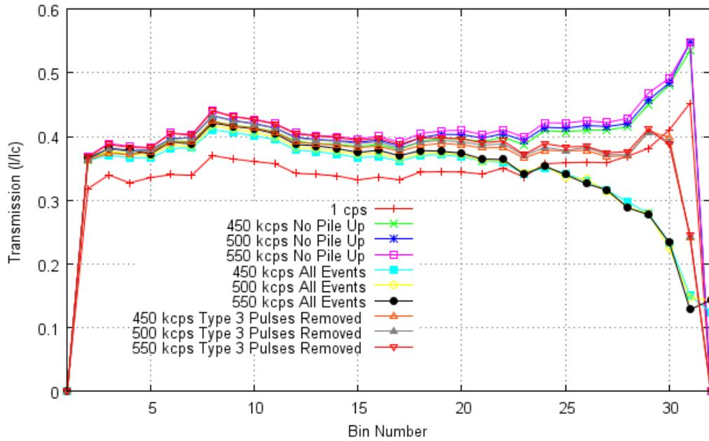
Fig 7-23 Modelled transmission spectra from a Geant4 simulation. Here the transmission is calculated from  $I/I_c$  where  $I_c$  is derived from a calibration block made from PEEK. The transmission data shown is with pile up removed, all events with no pile up removal and with type 3 events removed. Each simulation was carried out at rates of 450, 500 and 550 *kcps* as measured in  $I_c$ .
