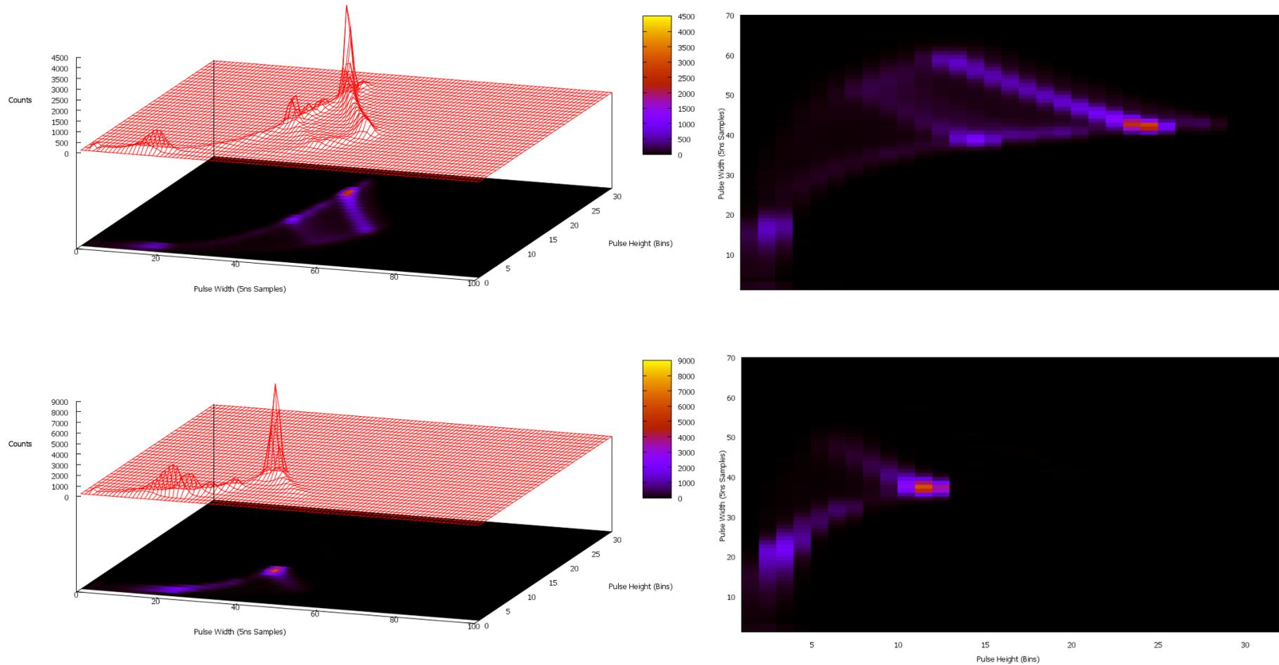
Fig 7-5 Three dimensional HW surface plots for  $^{57}\text{Co}$  (top left) and  $^{241}\text{Am}$  (bottom left) with corresponding density plots. 100,000 events were collected using a DSO90254A oscilloscope and Matlab analysis software. The main peaks are at 122.1 keV for  $^{57}\text{Co}$  and .59.5 keV for  $^{241}\text{Am}$ .
