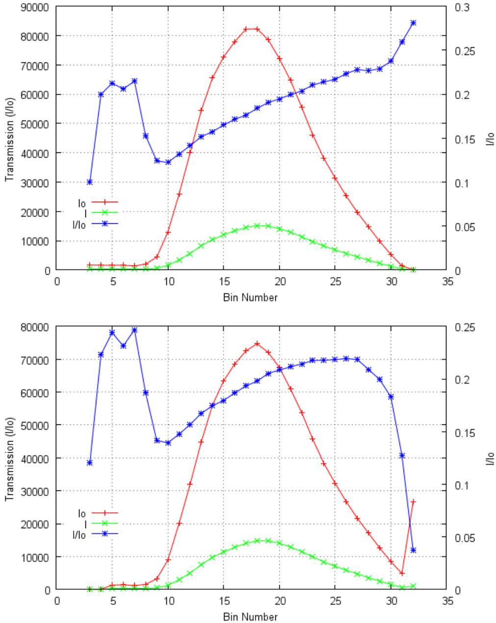
Fig 6-5 Simulated  $I$ ,  $I_0$  and  $I/I_0$  spectra for a 1000 ml bottle of water. The graph at the top of the figure shows a low count rate simulation at 1 cps and the graph at the bottom of the figure shows a simulation at 500 kcps.
