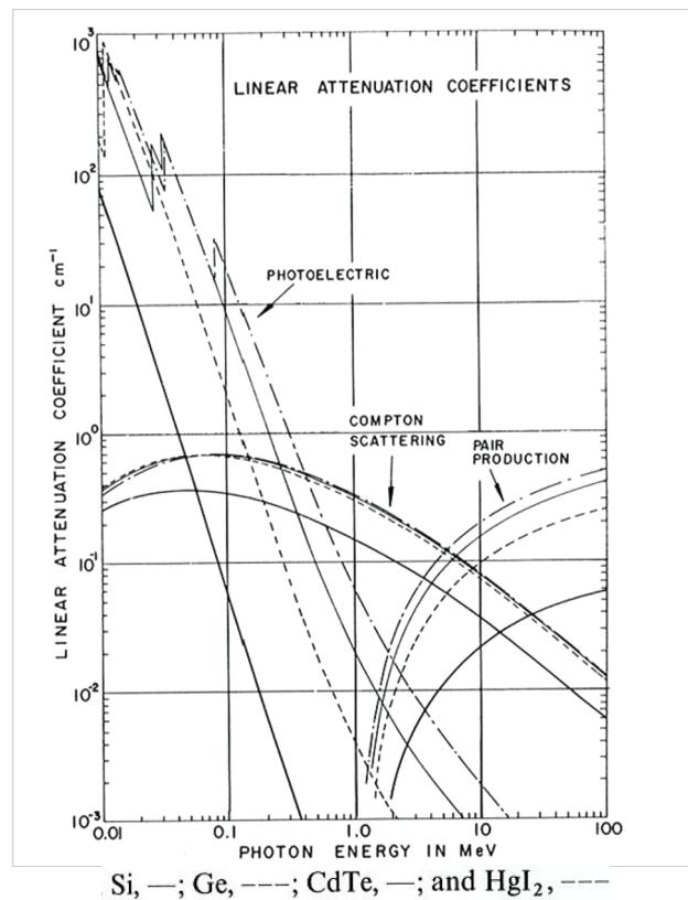
Fig 2-1 Linear attenuation coefficient as a function of energy for CdTe showing the energy regimes for the photoelectric effect, Compton scatter and pair production<sup>20</sup>.
