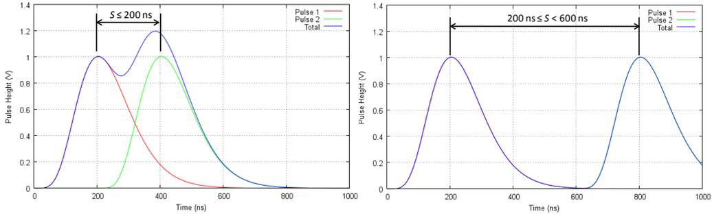
Fig 4-10 Illustration of Algorithm 3 showing the conditions for discarding pulses. Here if pulse separations,  $S \leq 200 \text{ ns}$  both pulses are discarded, if  $200 \text{ ns} \leq S < 600 \text{ ns}$  (right) only pulse 2 is discarded.
