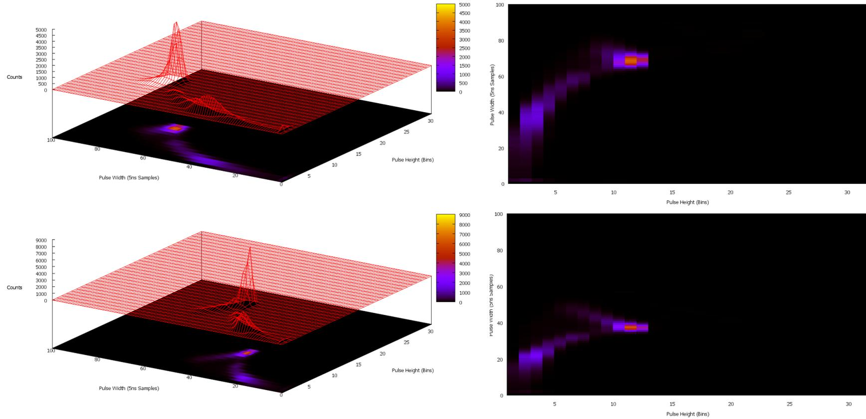
Fig 7-6 HW plots for 100,000 events with shaping times of 100 ns (top) and 50 ns (bottom) for a  $^{241}\text{Am}$  source. The main peak is at 59.5 keV.
