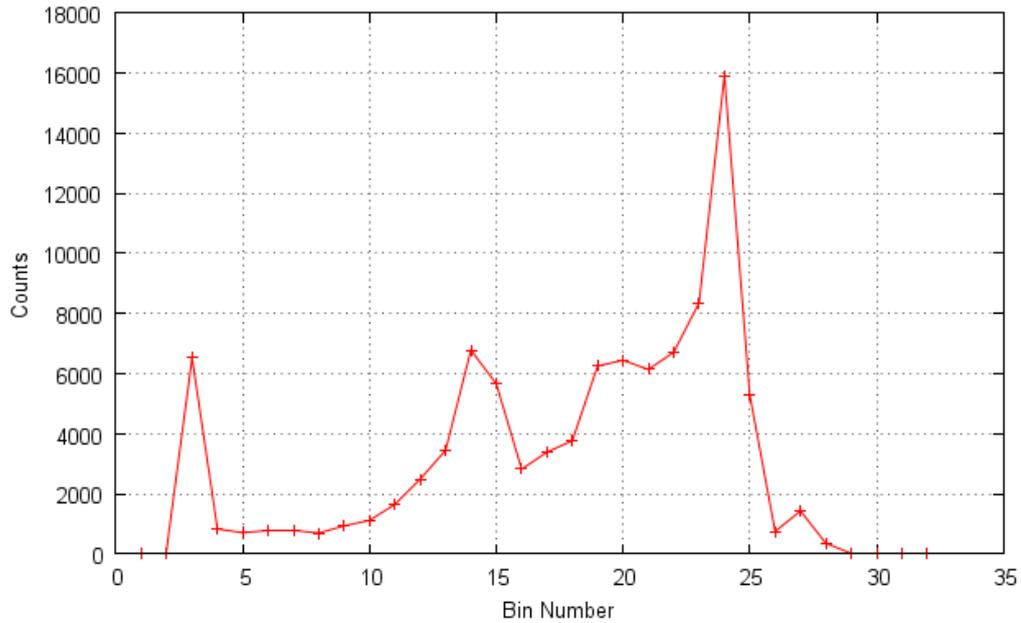
Fig 5-1 <sup>57</sup>Co spectrum captured using an oscilloscope emulation of Algorithm 1 with an Amptek XR-100T detector and a Cremat CR-200-100ns shaping amplifier. A total of 100,000 events were captured during this acquisition.
