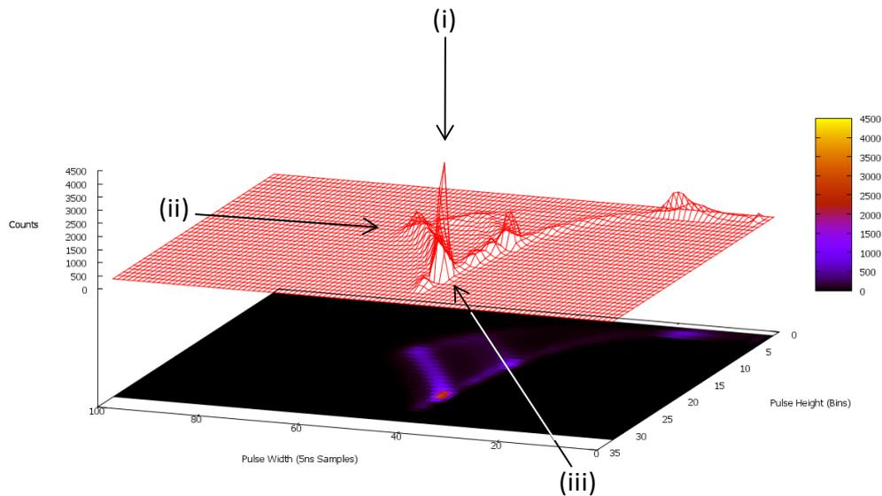
Fig 7-11 HW plot of the spectrum from a  $^{57}\text{Co}$  source. This 3D plot is of the same data set as that shown in Fig 7-4 with the third axis indicating the number of counts at a given  $(H, W)$  coordinate.
