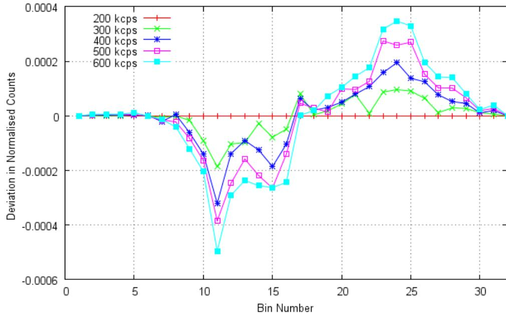
Fig 7-21 Deviations plot of normalised counts as a function of bin number for various count rates. Here the deviation is with respect to a rate of 200 *kcps* in  $I_c$  and the counts are taken only from those occupying the lozenge region of the HW plot.
