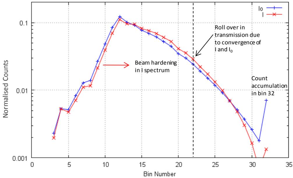
Fig 5-12 Normalised  $I$  and  $I_0$  spectra using pulse height detection Algorithm 1. Here the  $I$  measurement is taken with a 100 mm cuvette filled with water in the beam path. Note the log y scale.
