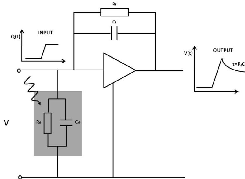
Fig 2-5 Schematic diagram of a charge sensitive preamplifier showing the input signal,  $Q(t)$  and the output signal,  $V(t)$ . The exponential decay of the output signal is defined by the time constant,  $\tau$  of the feedback resistor and capacitor  $C_f$  and  $R_f$  respectively.
