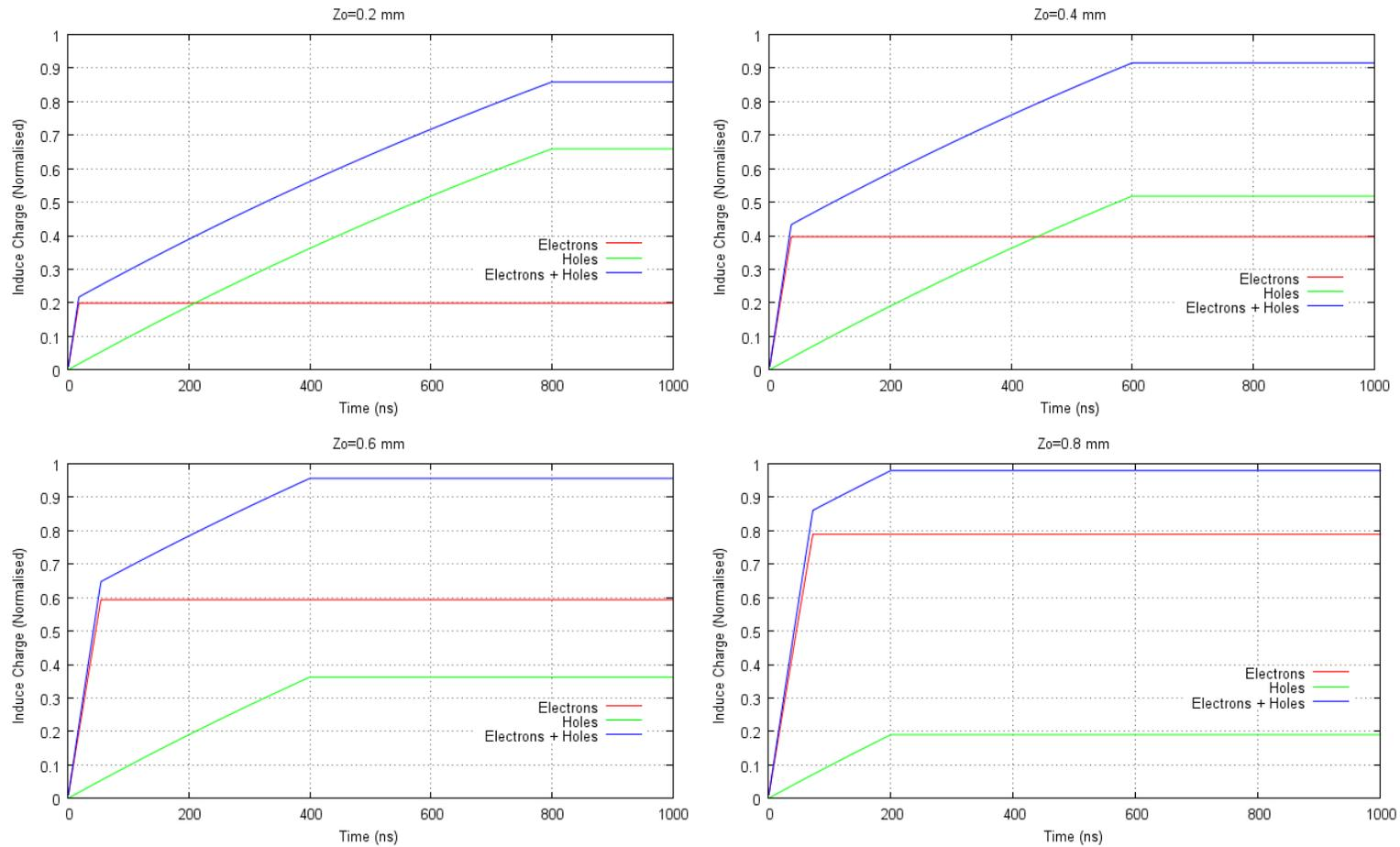
Fig 6-2 Simulation of charge transients for various depths of interaction within a 1 mm thick CdTe detector. Here a uniform electric field of  $1000 \text{ Vcm}^{-1}$  assumed and a mobility lifetime product for electrons and holes of  $3 \times 10^{-3}$  and  $2 \times 10^{-4} \text{ cm}^2 \text{V}^{-1}$  respectively. Here  $Z_0$  refers to the depth of x-ray interaction measured with respect to the cathode.
