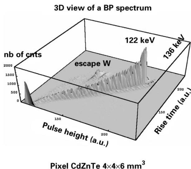
Fig 2-9 Biparametric spectrum from a <sup>57</sup>Co source<sup>47</sup>.
