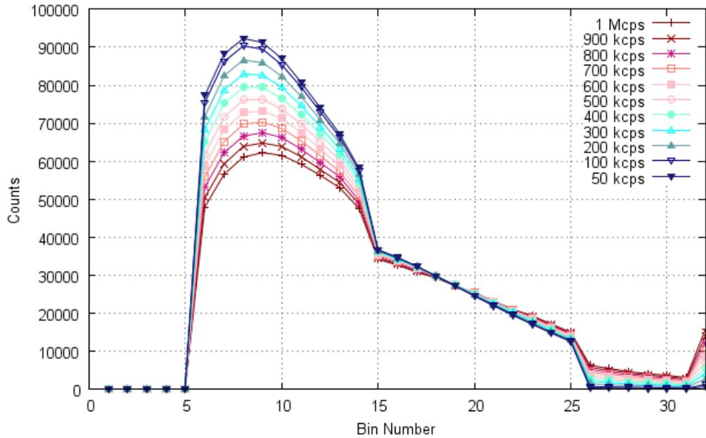
Fig 4-11 Spectra produced by pulse height detection Algorithm 1 for various input count rates using a data set of one million random events from 30 keV to 125 keV.
