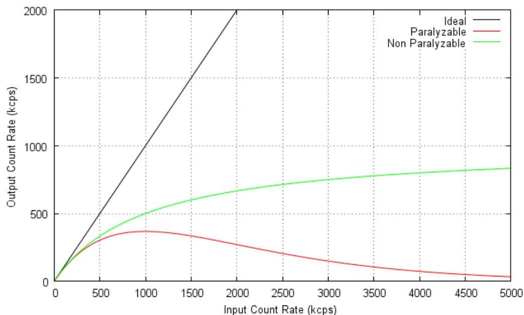
Fig 2-10 Output count rate as a function of input count rate for both paralyzable and non paralyzable pulse height detection systems. Here the dead time for both systems is  $560 \text{ ns}$  which is defined by the width of each pulse.
