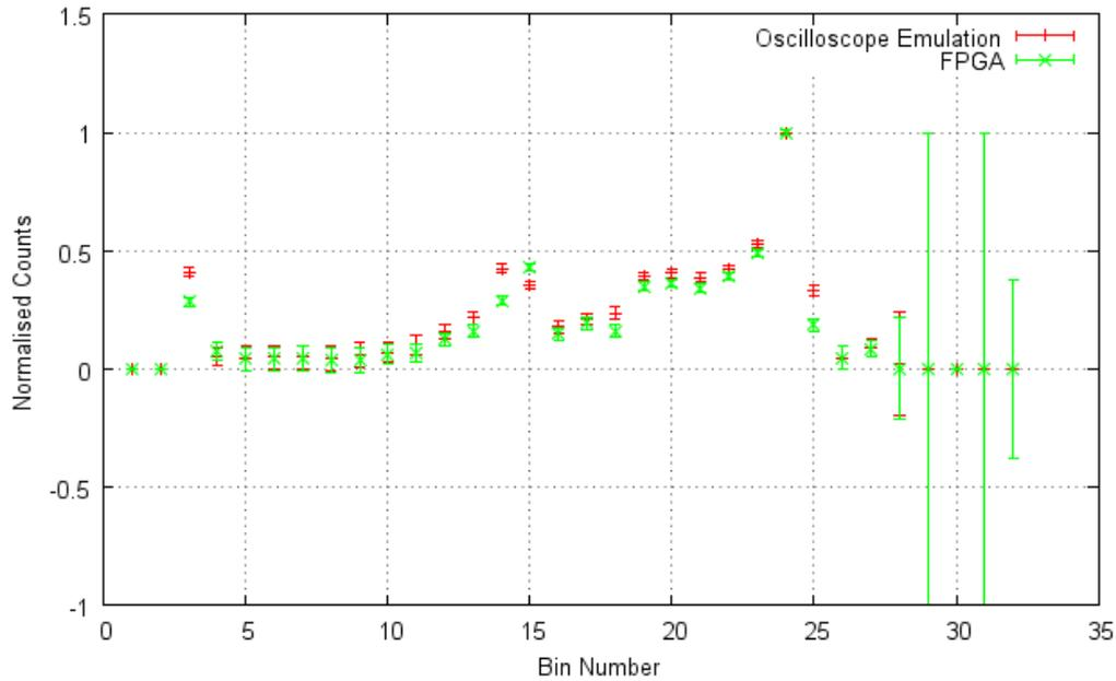
Fig 5-3 Graph showing  $^{57}\text{Co}$  spectra using an oscilloscope emulation of Algorithm 1 and an FPGA running the same algorithm in firmware. The error bars are derived from ten repeat measurements.
