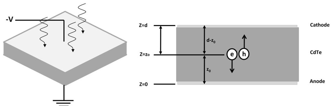
Fig 2-2 Diagram showing a planar detector with an applied bias voltage,  $-V$ . The cross section illustrates the generation of electron-hole pairs due to absorption of ionising radiation. The electrons and holes then drift towards the contacts under the influence of the electric field.
