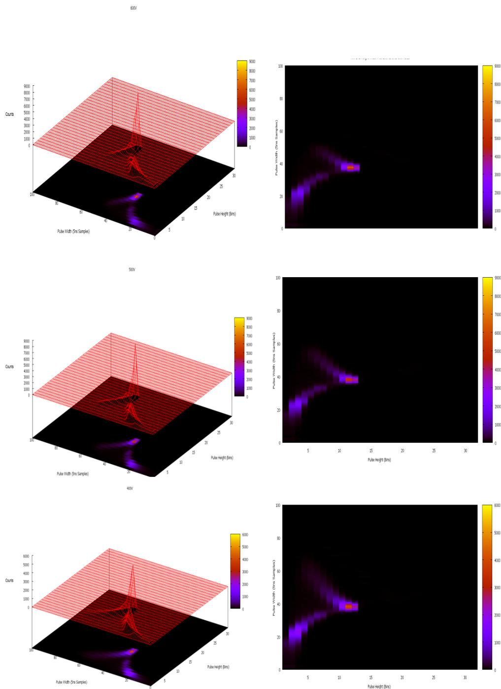
Fig 7-7 Three dimensional HW plots for 100,000 events using an  $^{241}\text{Am}$  source with a shaping time of  $50\text{ ns}$ . Here the acquisitions were carried out for different detector biases of  $600\text{ V}$  (top),  $500\text{ V}$  (middle) and  $400\text{ V}$  (bottom) to observe the effect on the  $59.5\text{ keV}$  tail.
