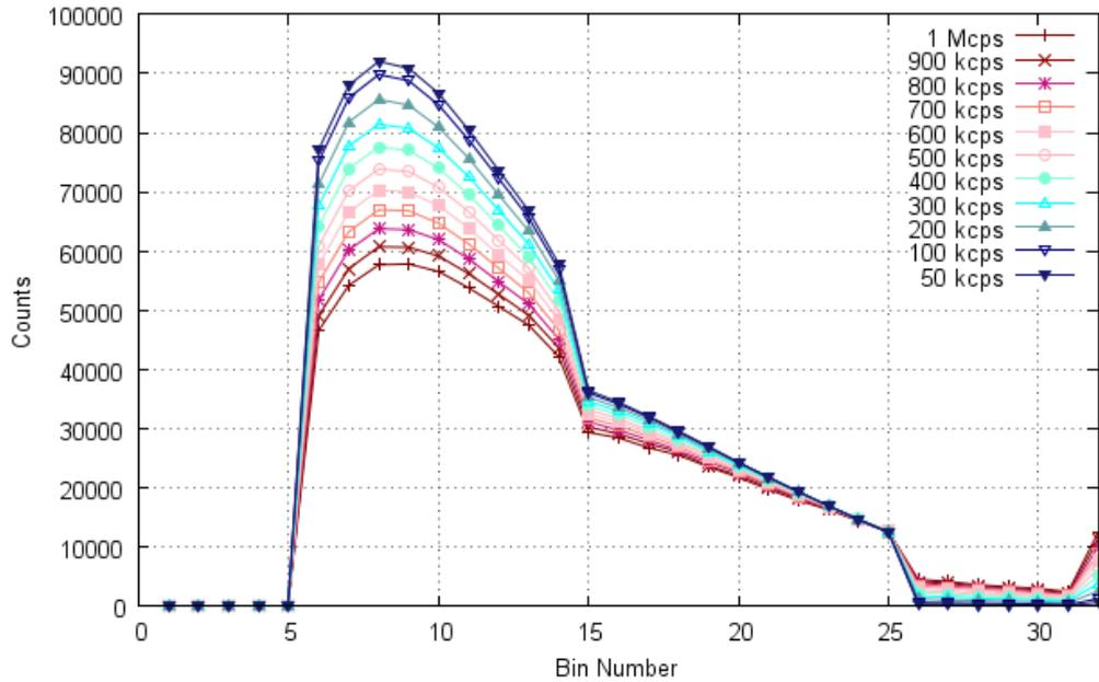
Fig 4-13 Spectra produced by pulse height detection Algorithm 2 for various input count rates using a data set of one million random events from 30 keV to 125 keV.
