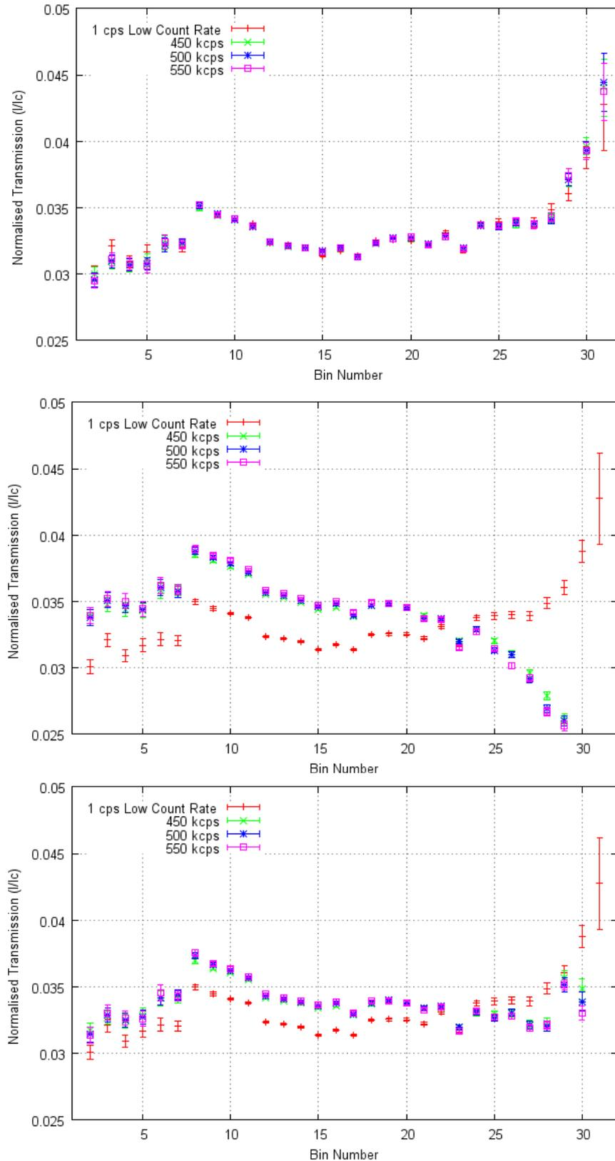
Fig 7-24 Normalised transmission spectra from a simulation with various degrees of pile up treatment: All pile up removed from  $I$  and  $I_c$  (top), no pile up removed (middle), and pile up removed from inside lozenge only (bottom). Each plot shows three spectra with a count rate of 450 kcps, 500 kcps and 550 kcps to illustrate the transmission stability at varying count rates. A low count rate simulation at 1 cps is also shown in each graph.
