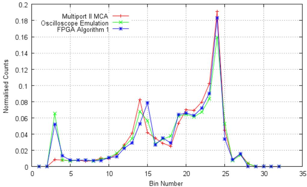
Fig 5-2 Comparison of  $^{57}\text{Co}$  spectra acquired using oscilloscope and FPGA implementations of Algorithm 1 along with an acquisition taken using a Canberra Multiport II MCA. Here the Multiport II spectrum shown is from Fig 3-5 and has been re binned into 32 bins for comparison.
