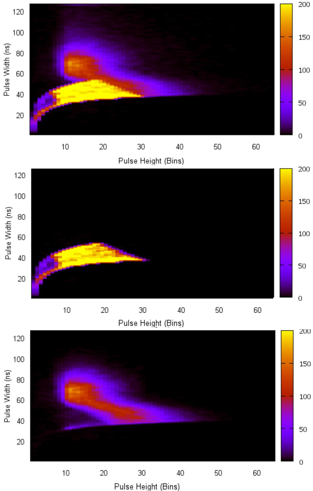
Fig 7-18 Simulation of x-rays incident on a detector from a tungsten tube. The spectra shown here are at a detected count rate of 500 *kcps* in  $I_c$ . From the top to the bottom of the figure: (a) HW density plot showing the locations of all piled up and non piled up events (top), (b) all non piled up events (middle), (c) piled up events only (bottom).
