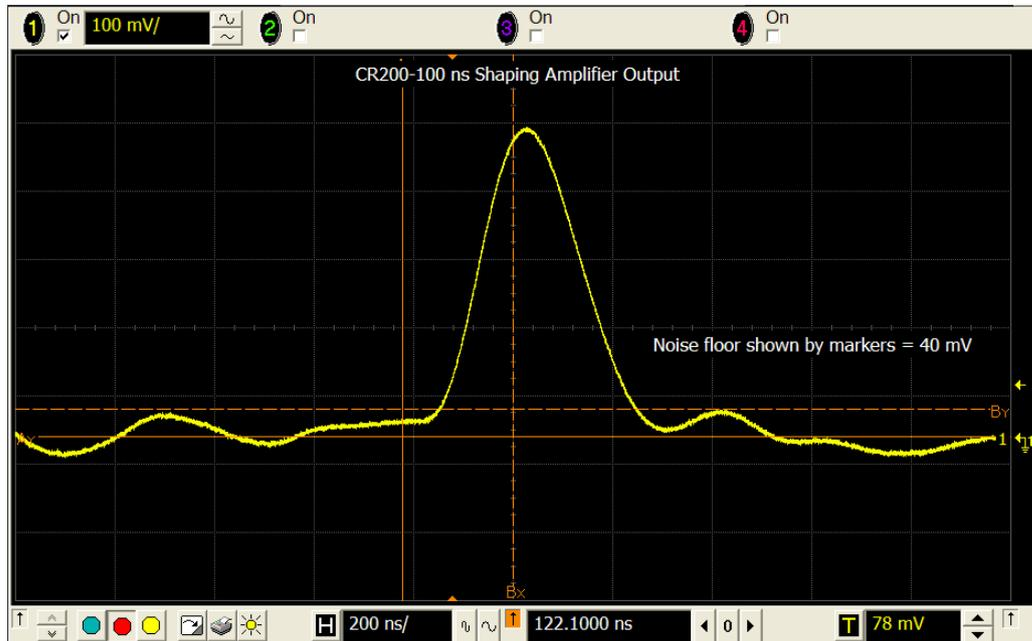
Fig 3-3 Shaped output signal from a CR-200-100ns shaping amplifier. As can be seen the noise appears below  $60\text{ mV}$ .
