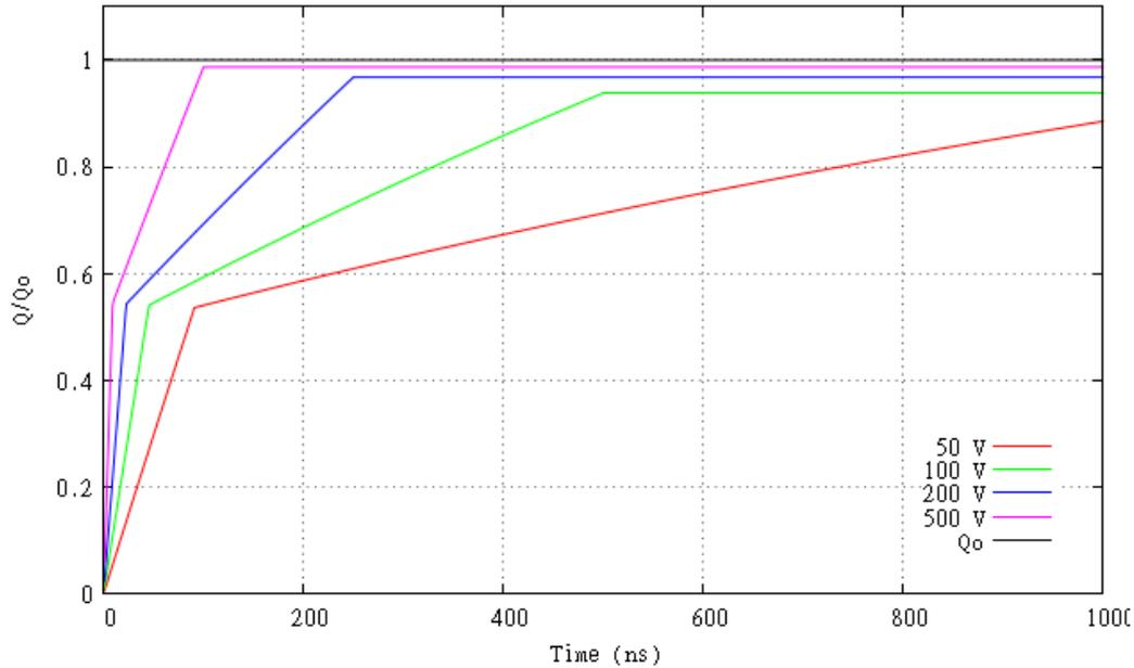
Fig 2-3 Graph showing the bias voltage dependence of the magnitude of the induced charge signal. Here the variation in amplitude is primarily due to the trapping of holes as they move a distance  $z = d/2$  to the cathode. The detector thickness is  $0.1 \text{ cm}$  and the mobility lifetime product of electrons and holes is  $3 \times 10^{-3} \text{ cm}^2 \text{ V}^{-1}$  and  $2 \times 10^{-4} \text{ cm}^2 \text{ V}^{-1}$  respectively.
