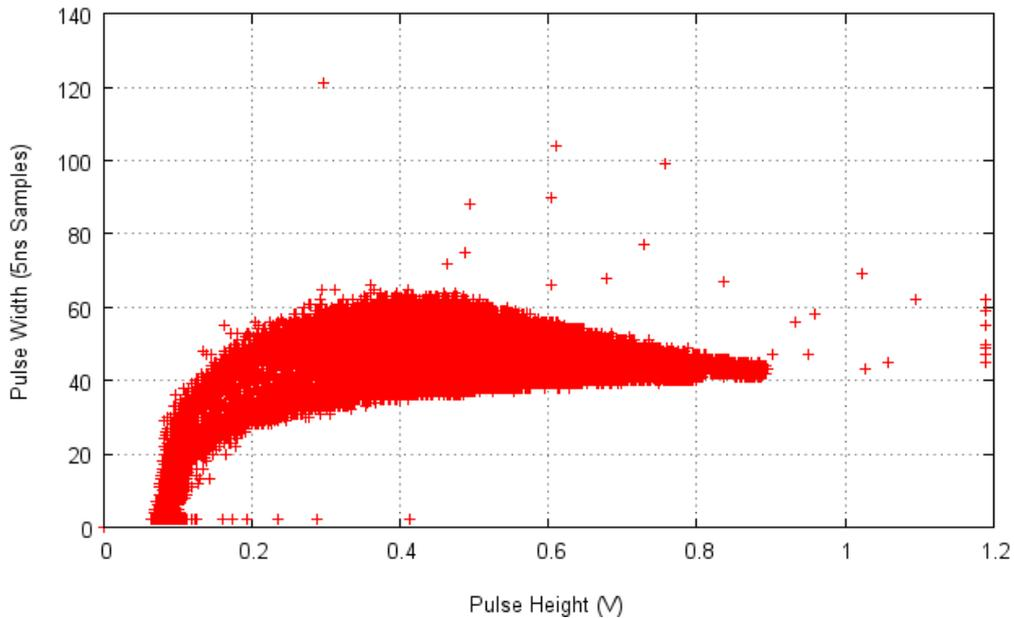
Fig 7-4 HW plot from a XR-100T detector for 100,000 events using a low count rate  $^{57}\text{Co}$  source in order to achieve a near pile up free measurement regime. Here the detector bias was 600 V and the shaping time was 50 ns.
