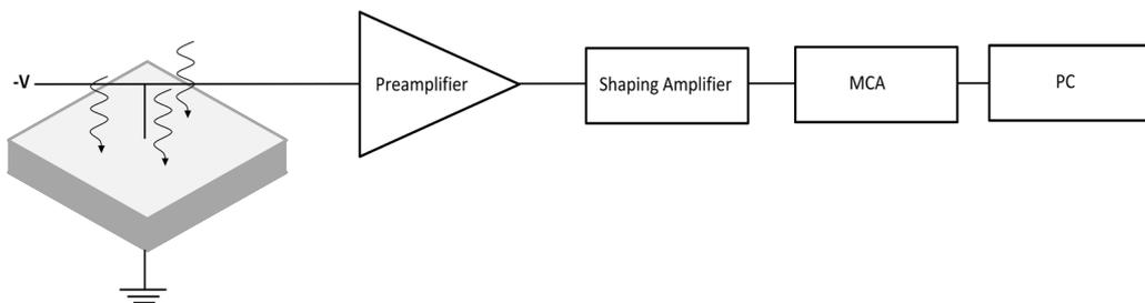
Fig 2-4 Diagram showing a typical semiconductor detector system consisting of detector, preamplification and shaping stages and pulse height analysis via a MCA and PC.
