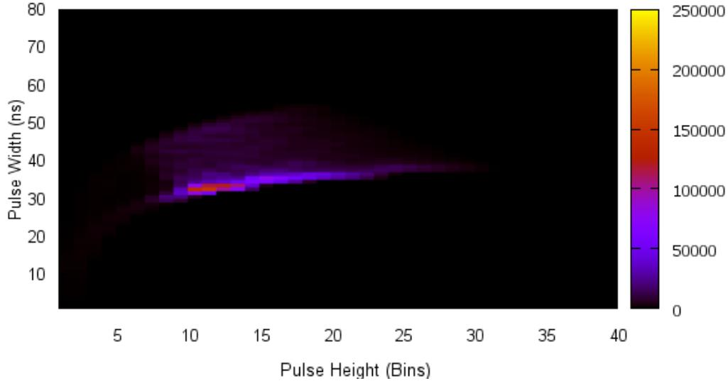
Fig 7-17 HW plot from a low count rate Geant4 simulation of the 0 to 160 keV x-ray spectrum from  $I_c$ . The simulation includes depth of interaction effects due to ballistic deficit and charge trapping which give rise to the characteristic shape of the plot.
