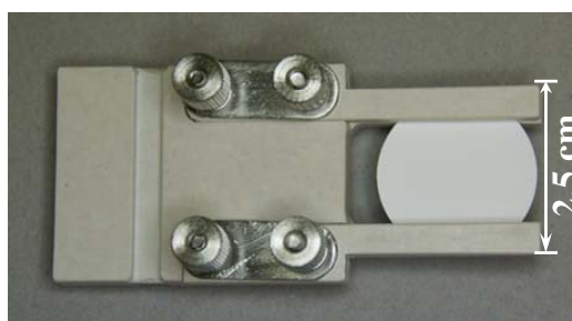
Figure 8.3 A porous membrane with the holder, used for LB film deposition.
