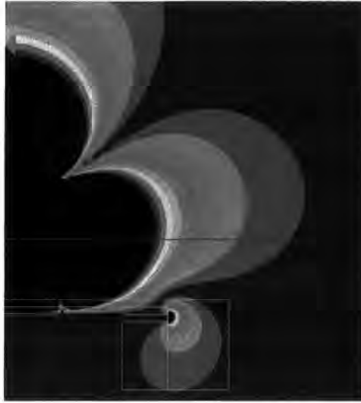
Figure 3.16. Demonstration of the edge effect on the z-component of the magnetic field around the target.
