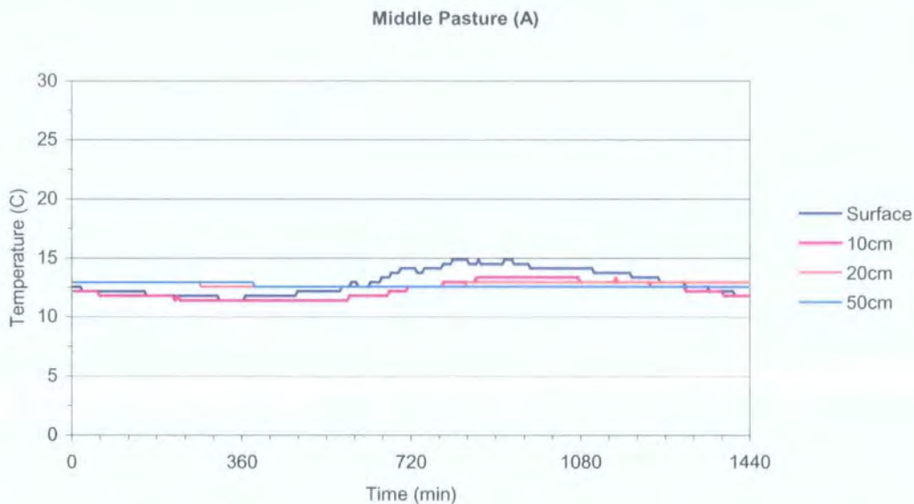
Figure 7.8: Diurnal thermal profiles at Site A under Stage II pasture 2000
