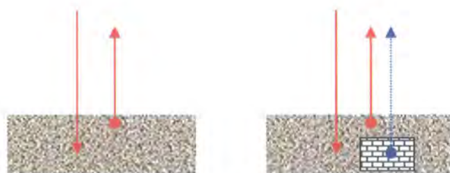
Figure 3.1: Effect of buried feature on thermal response detected at the surface
