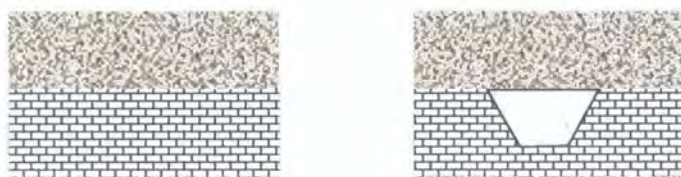
Figure 3.5: Two-layer and three-layer models representing subsurface structure, taken from Perriset & Tabbagh (1981)
