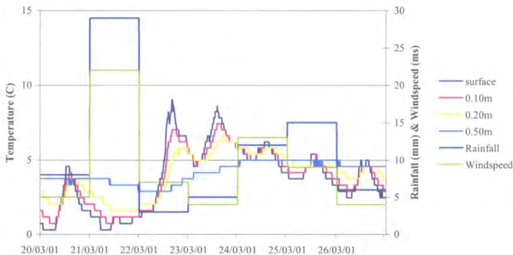
Figure 7.4: Thermal characteristics with overlay showing high daily rainfall and high wind speed
