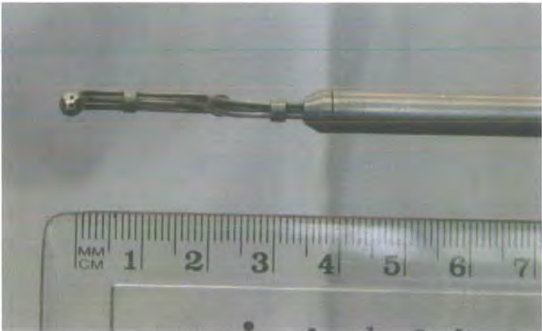
Figure C.3: Photograph of the Five-Hole Probe.
