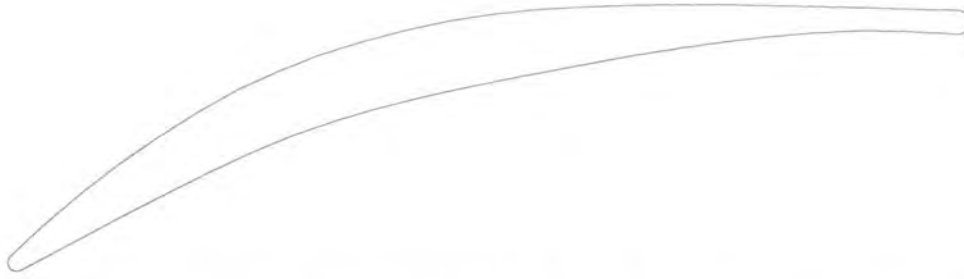
Fig. 7.6a Controlled diffusion airfoil blade of the oscillating compressor cascade
