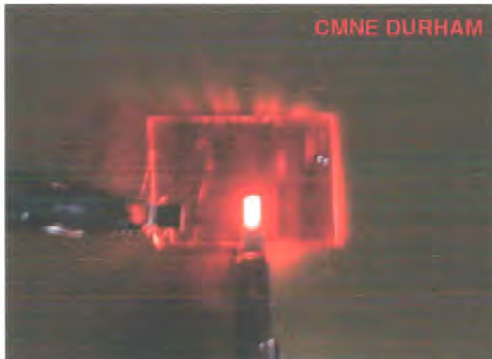
Figure 5: A photograph of a bilayer LED ITO/MEH(Ru)(90 nm)/ 36d (55 nm)/Al working at a current density of ca. 100 mAcm -2 under forward bias, without encapsulation. The peak external quantum efficiency of the LED was ca. 0.7% and the brightness was ca. 4,000 cd m -2 . 30
