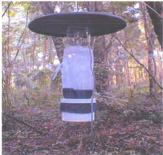
Plate 8.2 CDC light trap baited with CO 2 with auto switching for night-time release of gas and lighting used as part of West Nile virus surveillance.
