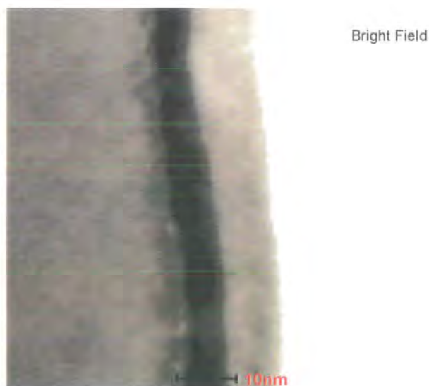
Figure 3.7: Cross-sectioned transmission electron image of a Si/Ni 81 Fe 19 (8nm)/Al(10nm) bilayer.
