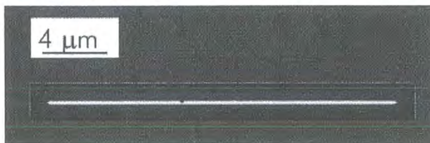
Figure 6.12: FIB image of a 20 \mu\text{m} wire, with a trap of D_t = 150 nm in the wire side.
