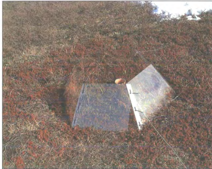
Figure 2.4: An example of an open-top chamber in the lower tundra site. The OTC had an area of 1 m 2 at the base and reached approximately 50 cm off the surface of the ground. The OTCs were secured with guy ropes to prevent movement. Photograph taken April 2003.
