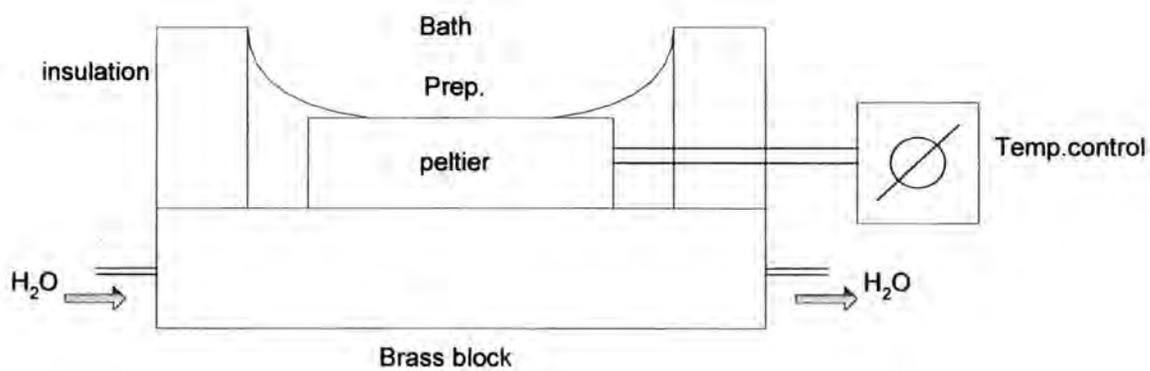
**Figure 2.2: Peltier junction.**
