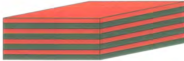
Figure 1.2: Two materials with different refractive indices (red and green) may be used to form a dielectric stack, or multi-layer film. The periodicity of the layers restricts the propagation of electromagnetic waves perpendicular to their surface. The device could also be referred to as a one-dimensional photonic crystal.
