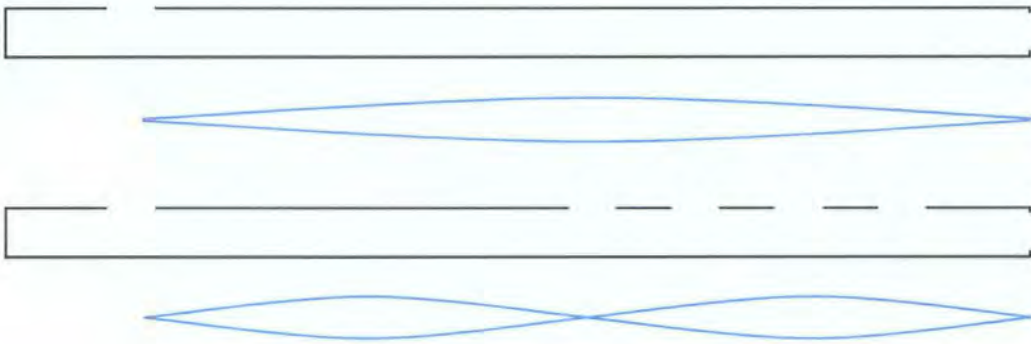
Figure 2-4 Fundamental waves on a flute
