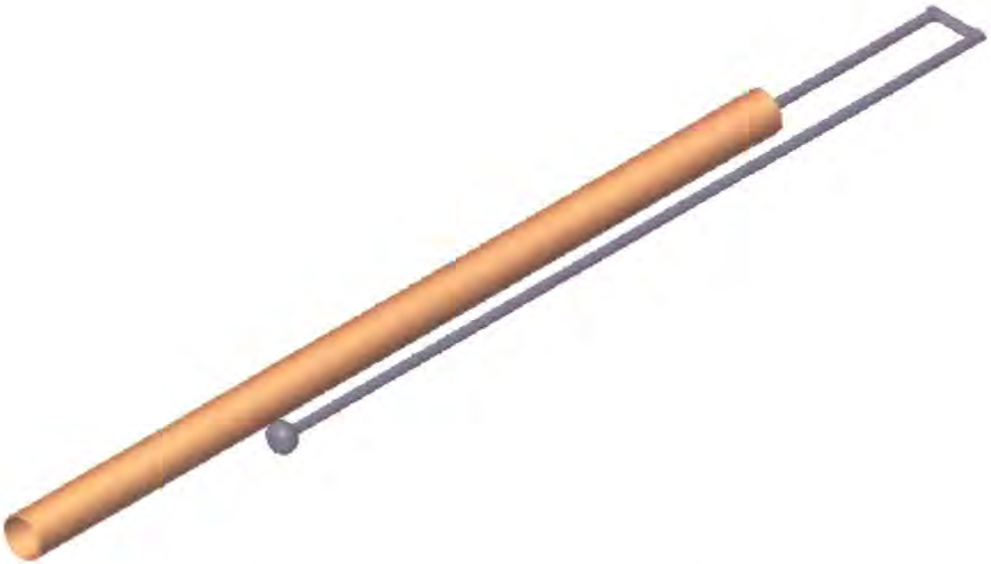
Figure 7-7 Modified design of plunger flute
