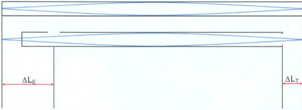
Figure 2-5 A flute with its actual length and its acoustical length
