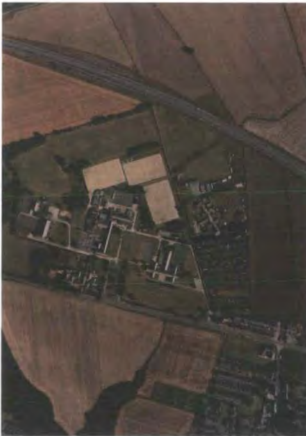
Fig. 156 The straight boundary between Walbottle Campus and the allotment gardens is the course of the Walbottle Moors Waggonway, preserved here as a track (copyright R&I 10591057, 7 September 1991). The route has been broken by the A69 dual carriageway, but in the ploughed field to the north of the road, it continues as a dark linear soilmark.
