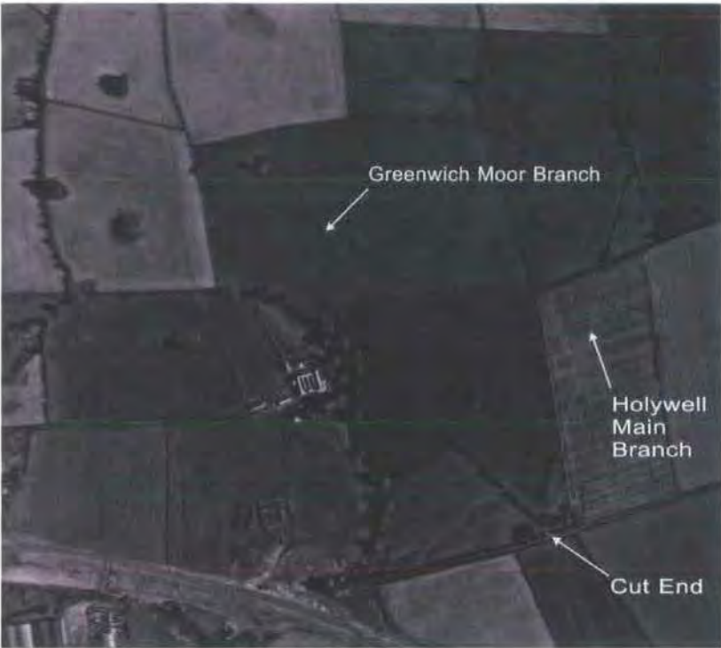
Fig. 153 The earthwork and cropmark remains of the 1769 Walbottle Moors Waggonway are clearly visible on this aerial photograph – the two branches meet at Cut End. (copyright Fairey Surveys Ltd 5640, 27 August 1974)
