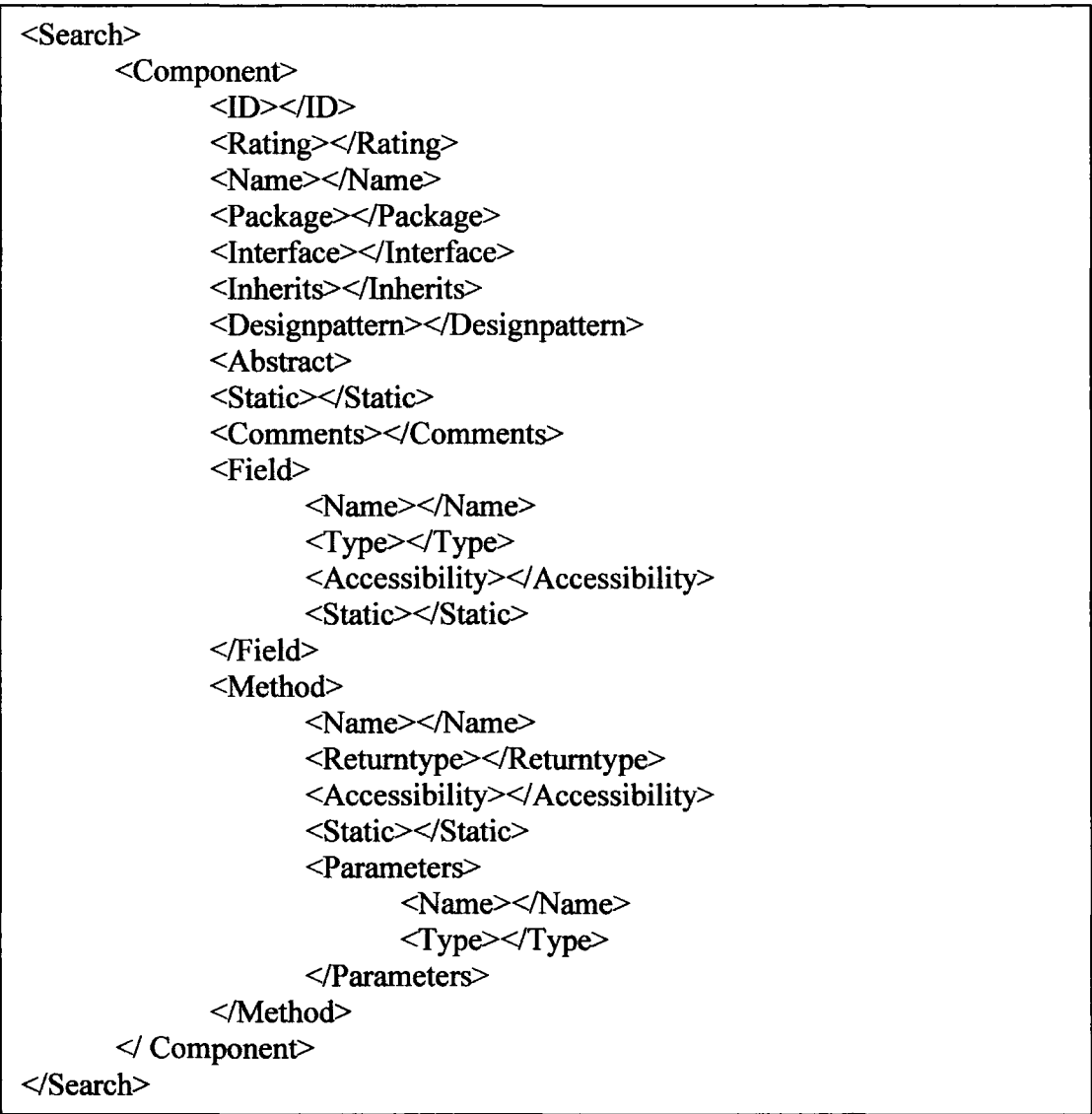
Figure 3.4-2: The XML encodings for sending a response for a search request from the identify components web service.
