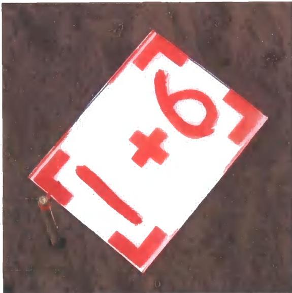
**Figure 2.8** Panel used for ground control points (GCPs)
