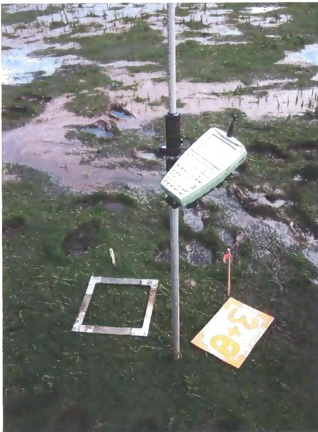
Figure 2.9 30 cm<sup>2</sup> quadrat and GPS used to denote position
