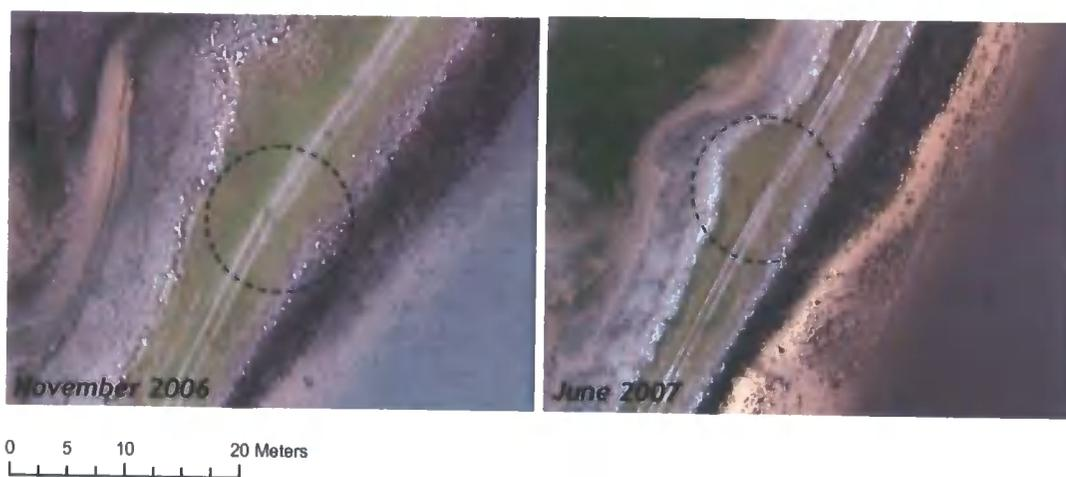
**Figure 4.3** Inaccurate image 'stitches' produced by mosaicking process
