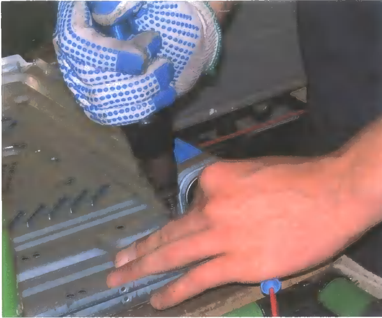
Illustration 5.6. Using the down-driver to secure the clip on the capacitor
