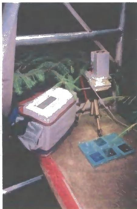
**Plate 7.2:** Photograph showing the LCA4 set up on a scaffolding platform, with an artificial light source attached to the conifer leaf chamber and the five null density glass filters.
