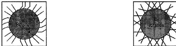
(a) The rotation of a circular brush in a square box (b) X-PLY mechanism stops the rotation
