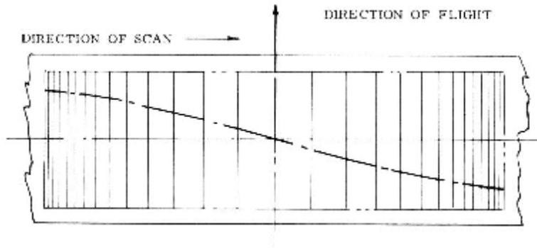
Figure 13-5 – Effect of IMC distortion of centreline scan.
