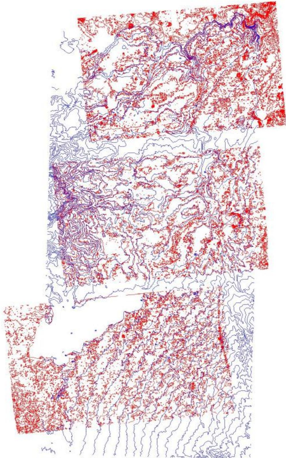
**Figure 8-8 – Contour comparison. The blue line shows contours of the map at 10 m intervals, the red line shows the contours derived from the DEM. The visual inspection shows a good fit.**
