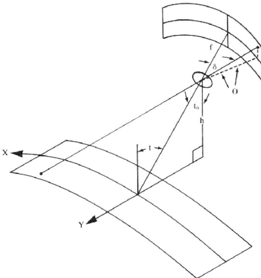
Figure 13-10 – Panoramic camera footprint (Slama *et al.*, 1980, p.942).
