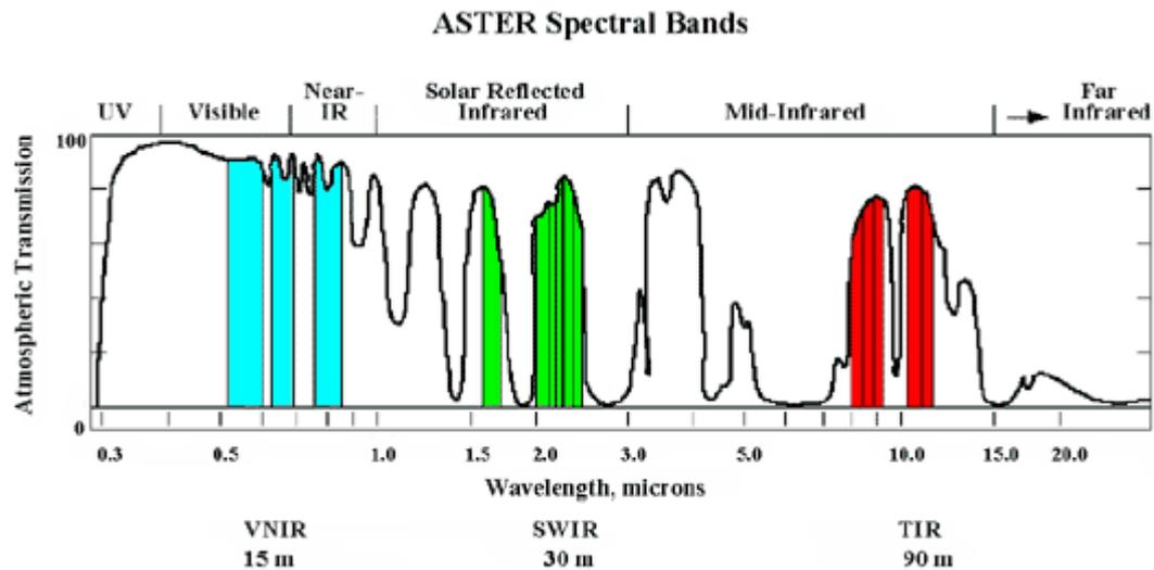
Figure 3-3 – ASTER bands superimposed on model atmosphere
