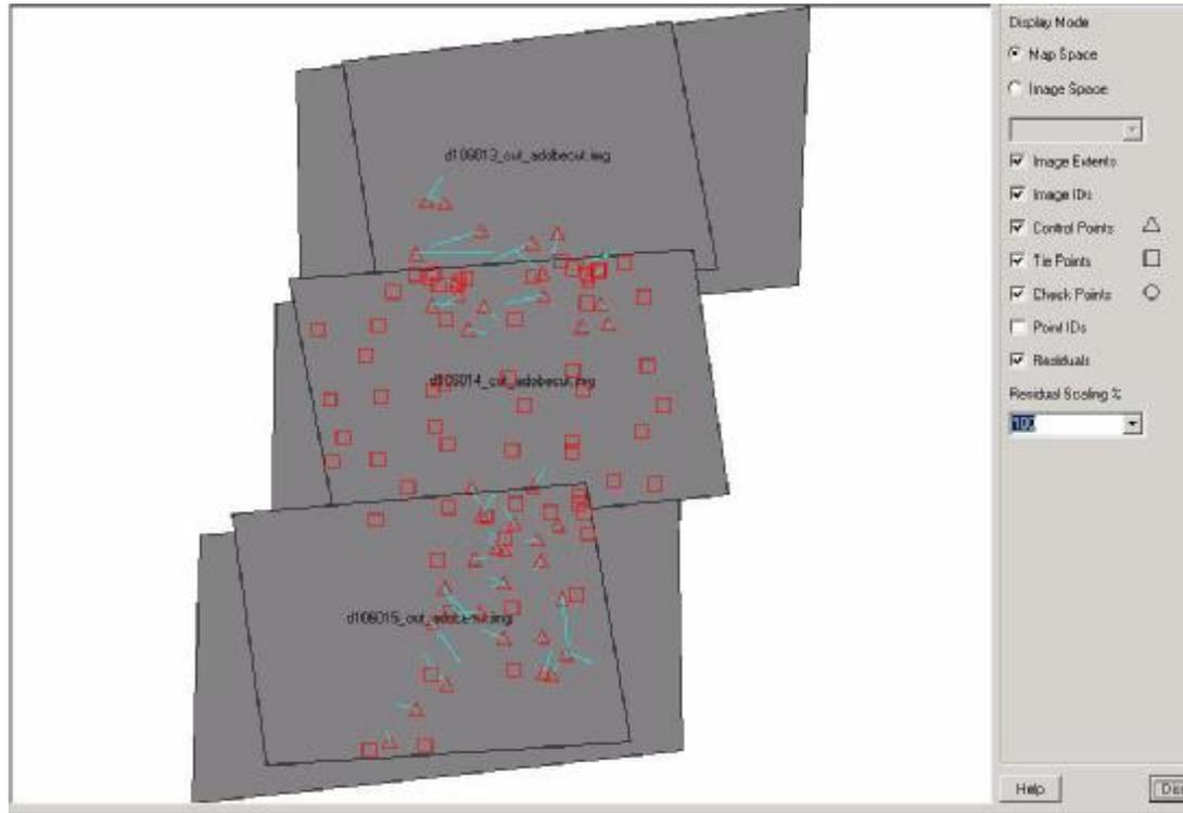
**Figure 7-8 – Distribution of GCPs and tie points in the strip stereopair.**
