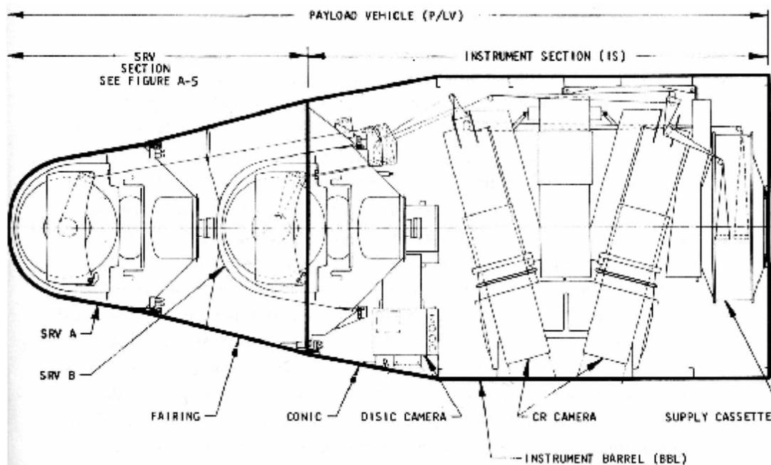
Figure 2-6 – The KH-4B satellite (Source: Day *et al.*, 1998)
