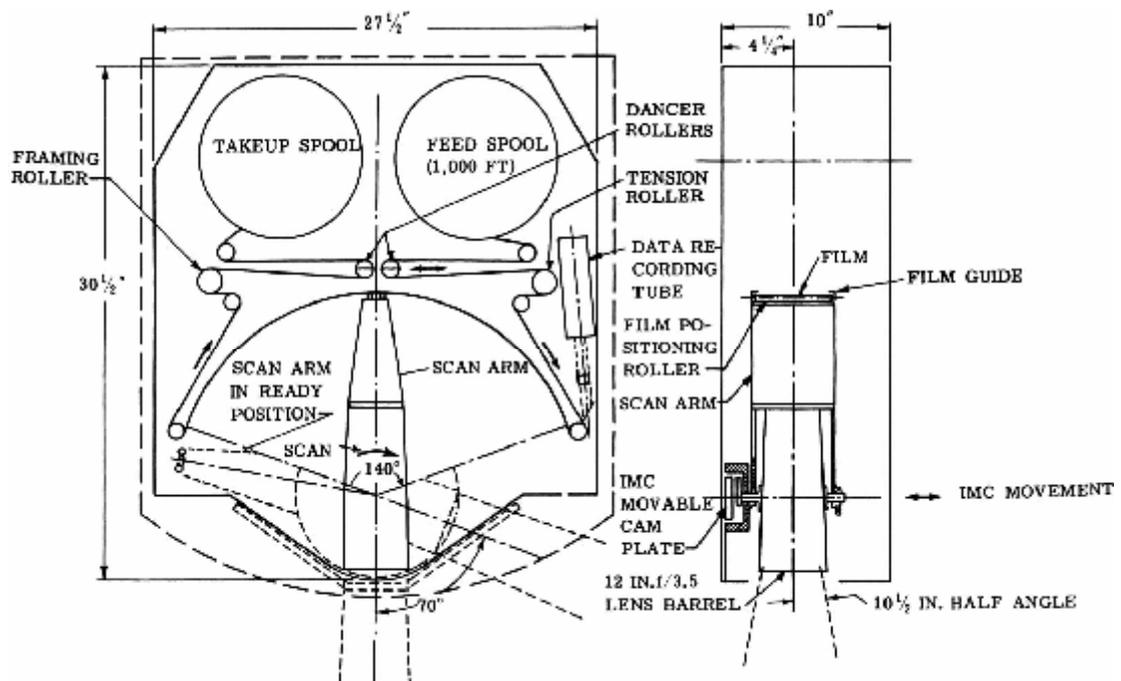
Figure 2-2 – HYAC panoramic camera (Source: Slama et al., 1980).
