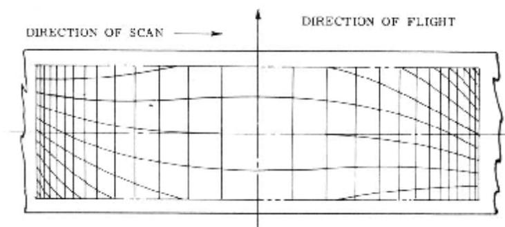
Figure 13-7 – Resultant image in the vertical panoramic camera.
