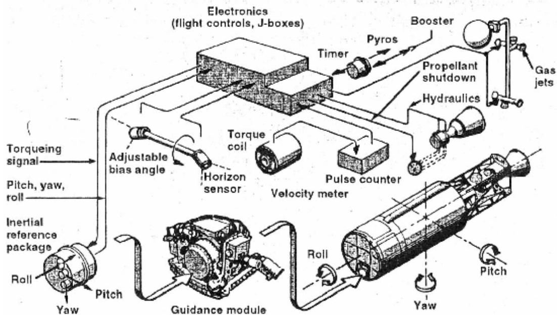
Figure 2-11 – The guidance and control system (Source: Powell, 1997)
