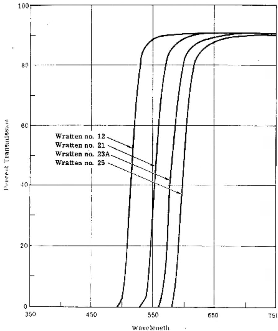
Figure 2-14 – Characteristic curves of CORONA filters (NRO, 1970b).
