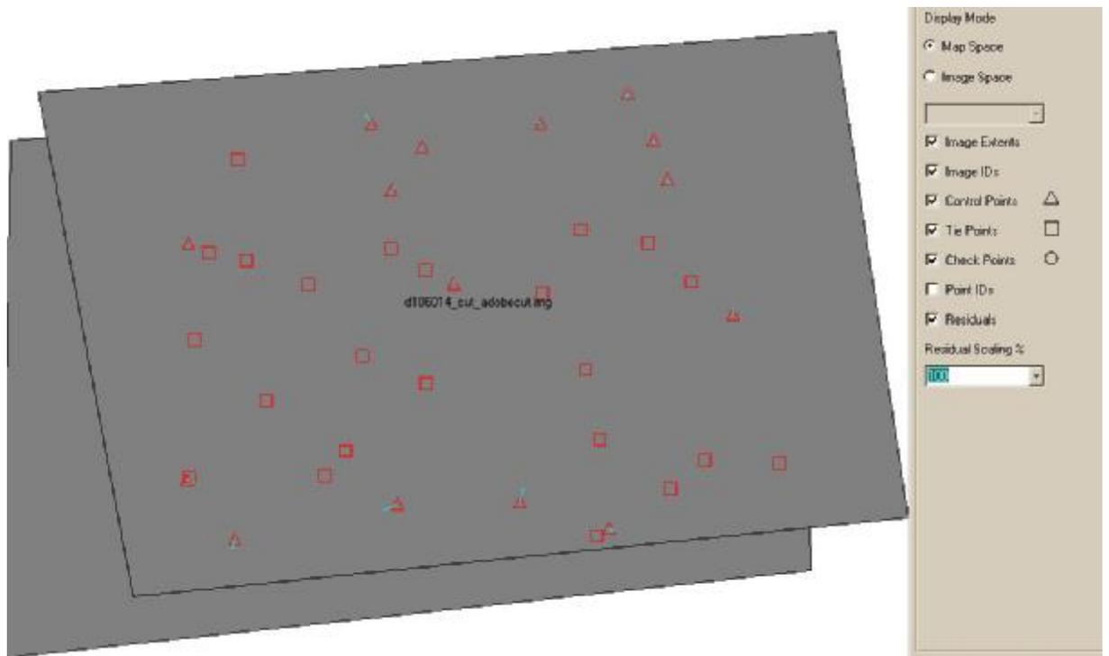
Figure 15-5 – Distribution of GCPs and tie points within the stereopair 008-014.
