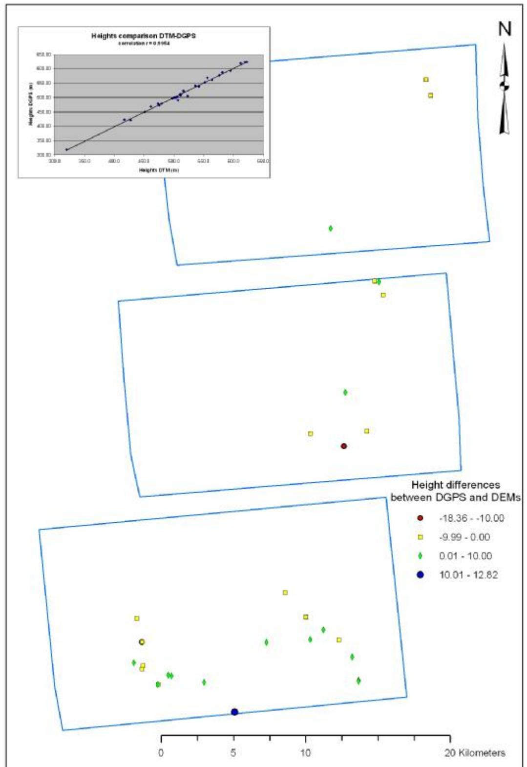
Figure 8-7 – The spatial distribution of the DGPS check points within the DEM footprint is shown here in with the DEM-DGPS chart. Correlation  $r = 0.9954$ .
