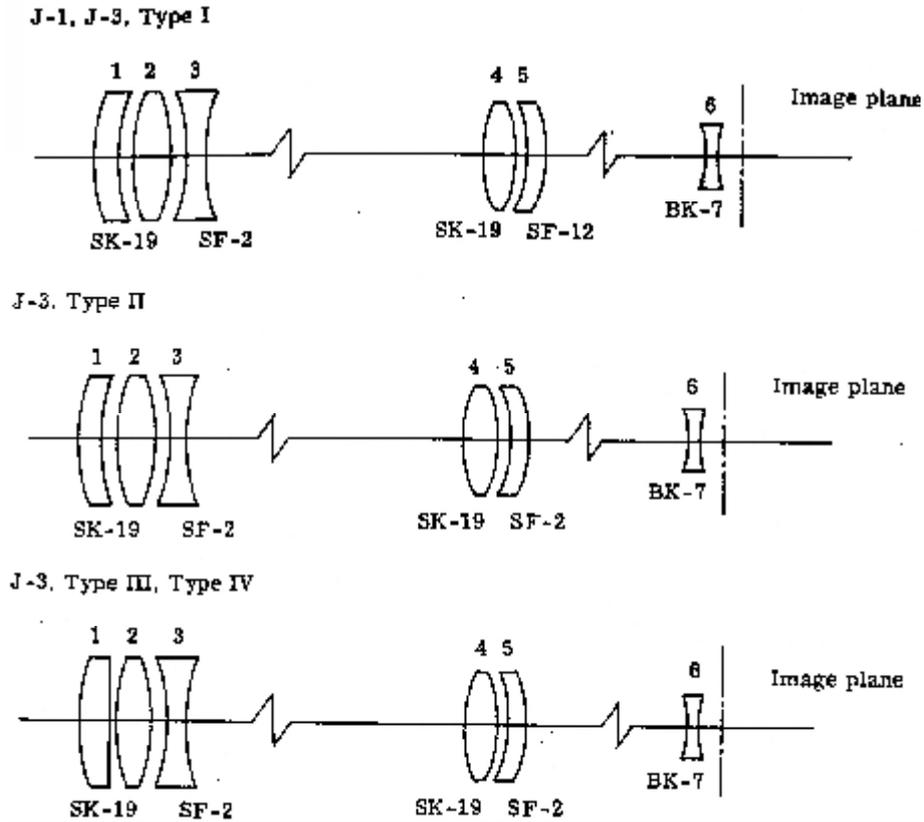
Figure 2-7 – Petzval lens diagrams (NRO, 1970a)
