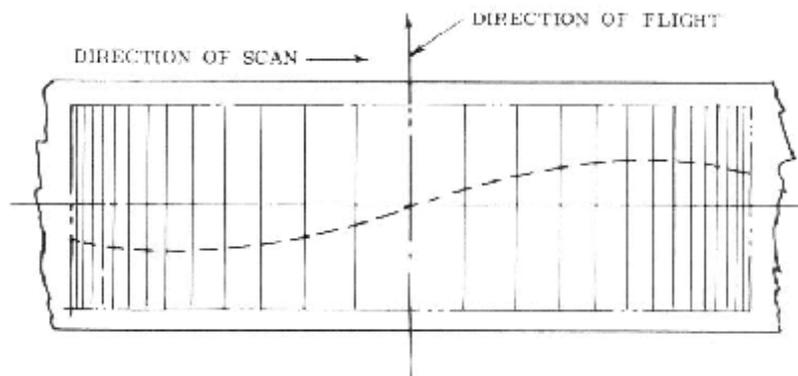
Figure 13-4 – Scan positional distortion superimposed on panoramic distortion.
