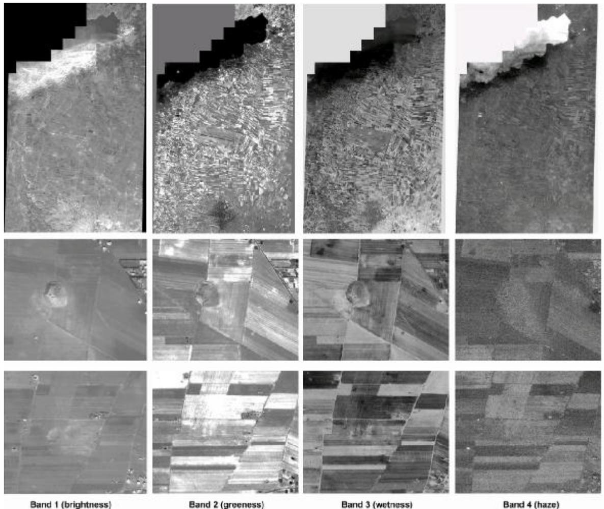
**Figure 5-14 – Tasseled-cap transformation applied to IKONOS multispectral image.**
