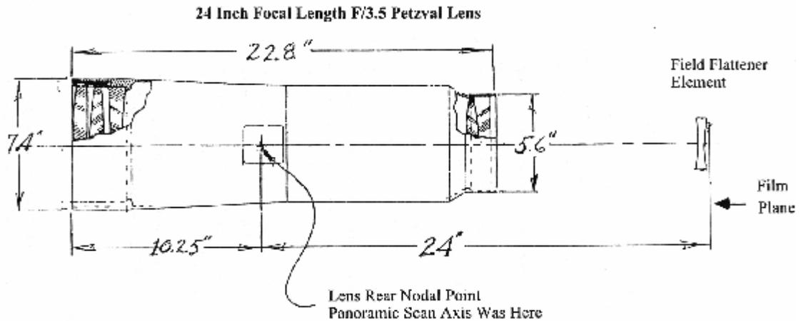
Figure 2-1 – The CORONA Petzval lens design (Madden, 1996)
