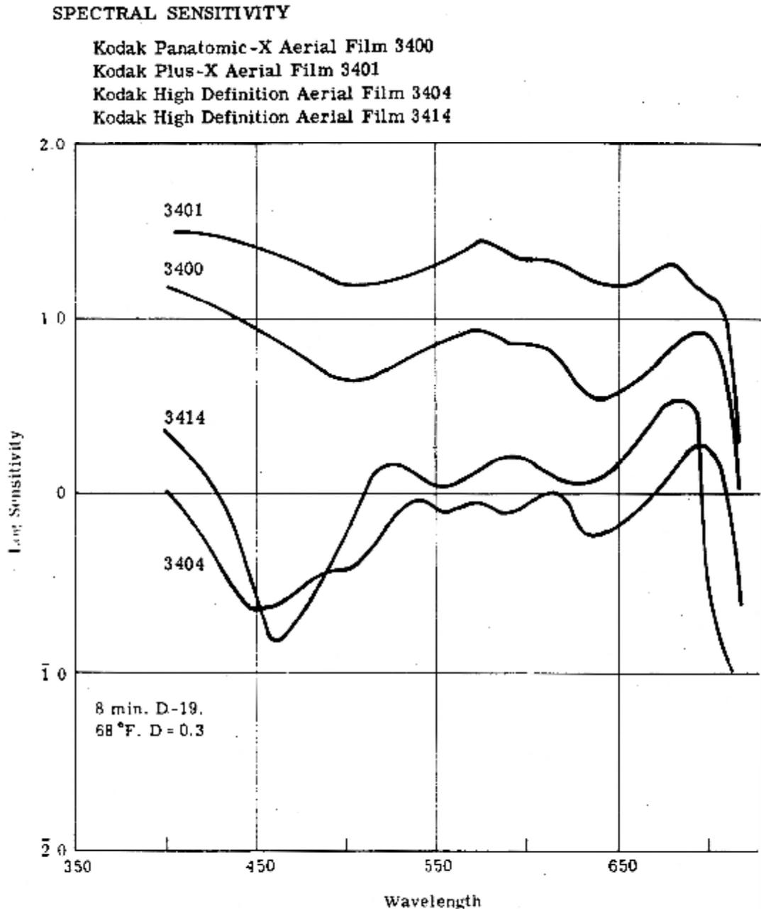
Figure 2-15 – CORONA films. Spectral sensitivity curves (NRO, 1970b).
