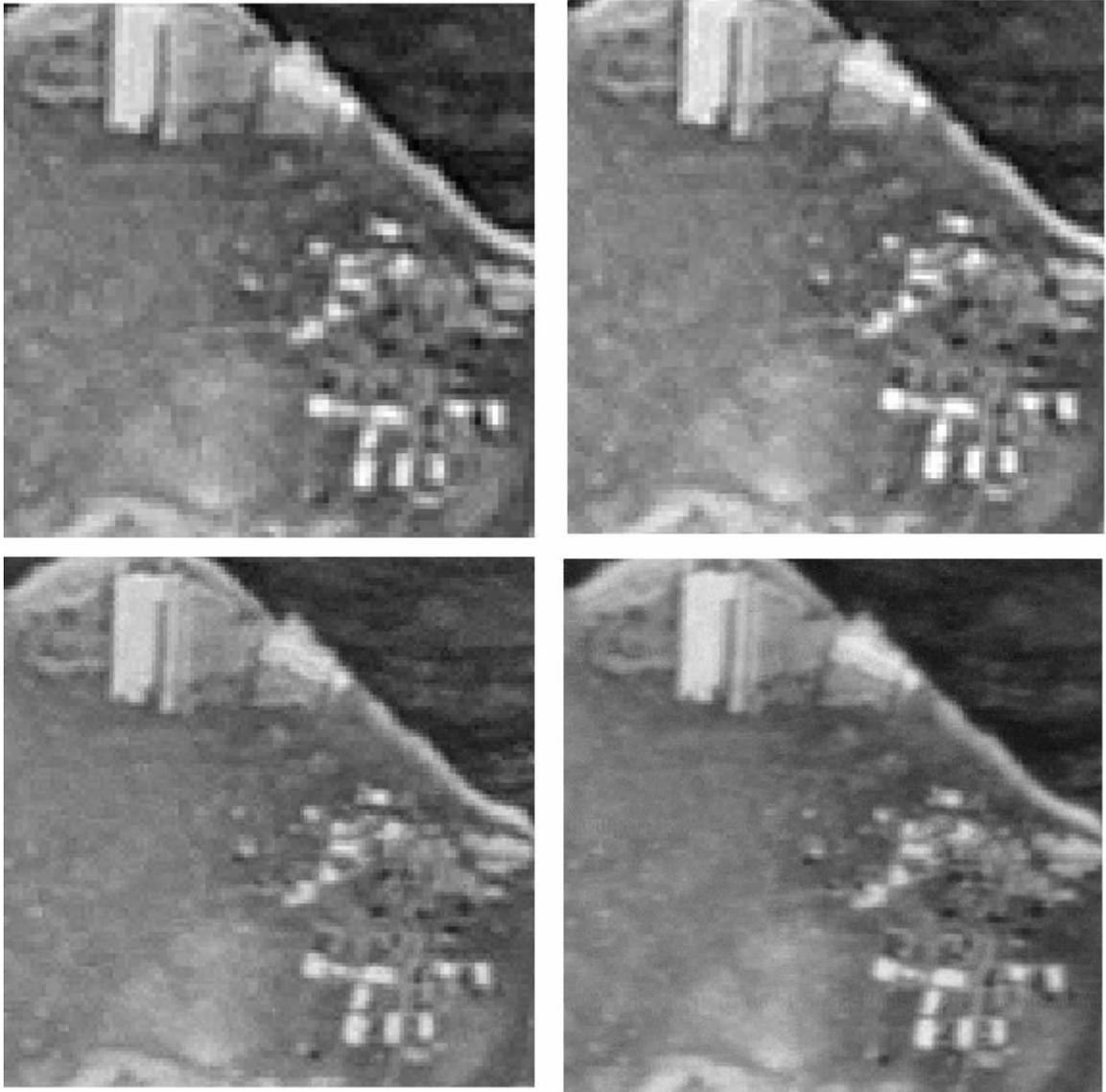
Figure 4-3 – Different scanning resolutions of the same area. Upper left 22.5  $\mu\text{m}$  (~1100 dpi), upper right 20  $\mu\text{m}$  (~1300 dpi), low left 15  $\mu\text{m}$  (~1700 dpi), and low right 7.5  $\mu\text{m}$  (~3400 dpi).
