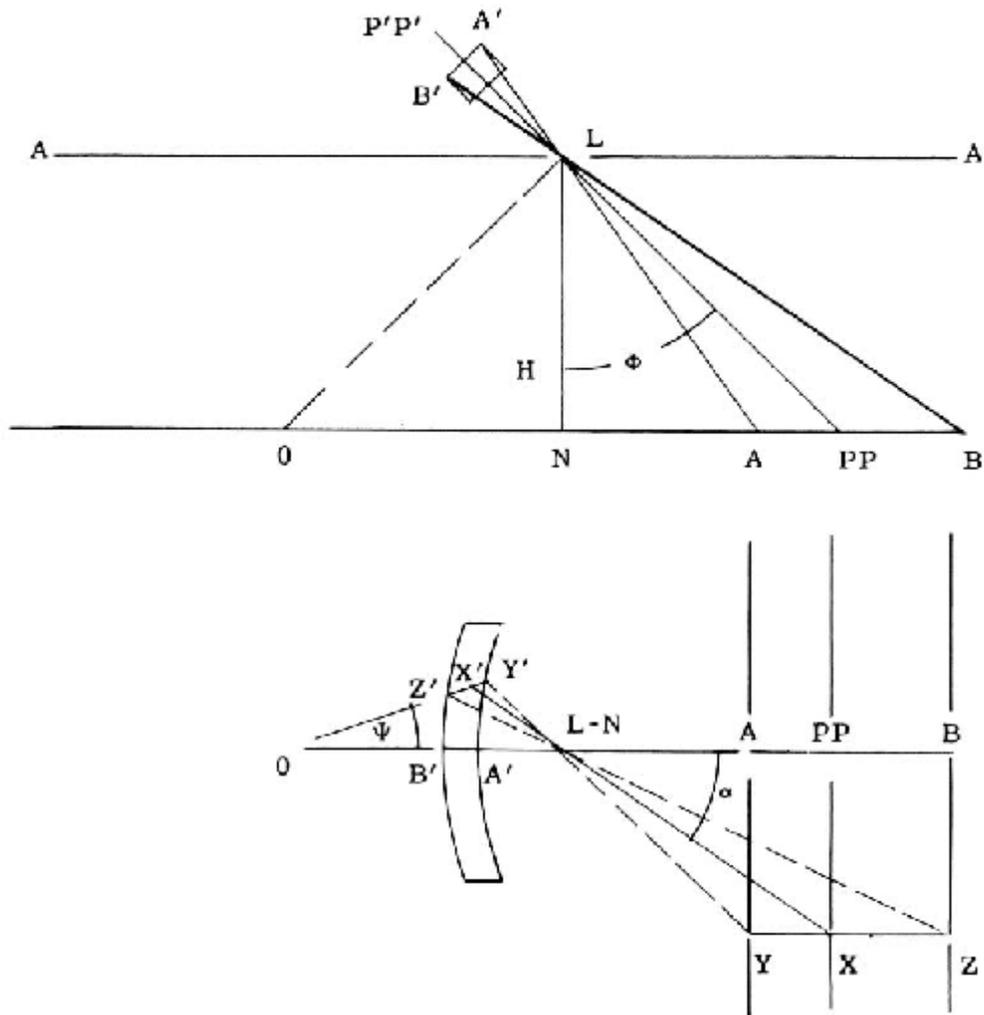
Figure 13-8 – Geometry of tipped panoramic distortion.
