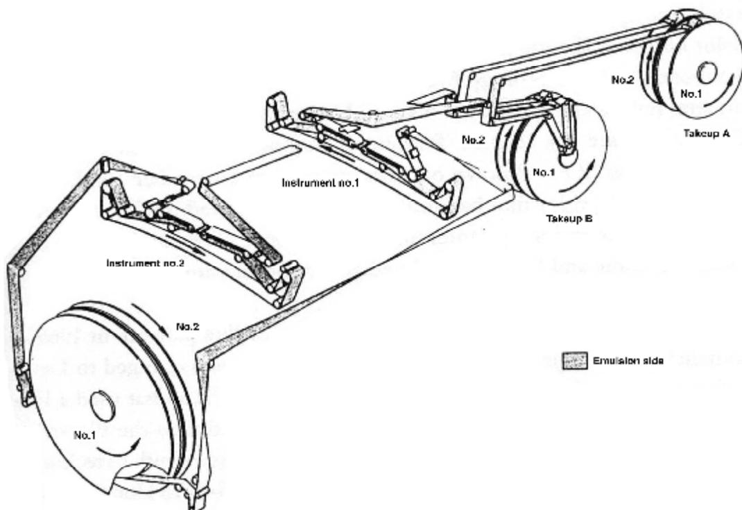
**Figure 2-5 – The film path of the KH-4B spacecraft. It has all these twists and turns because of the need to accommodate the small diameter of the satellite. The counter-rotating motion of the film and the cameras improved stability of the satellite (NRO, 1970b).**
