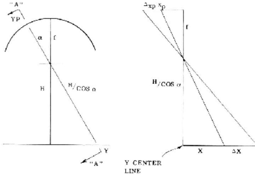
Figure 13-1 – Geometric relationship of panoramic distortion.
