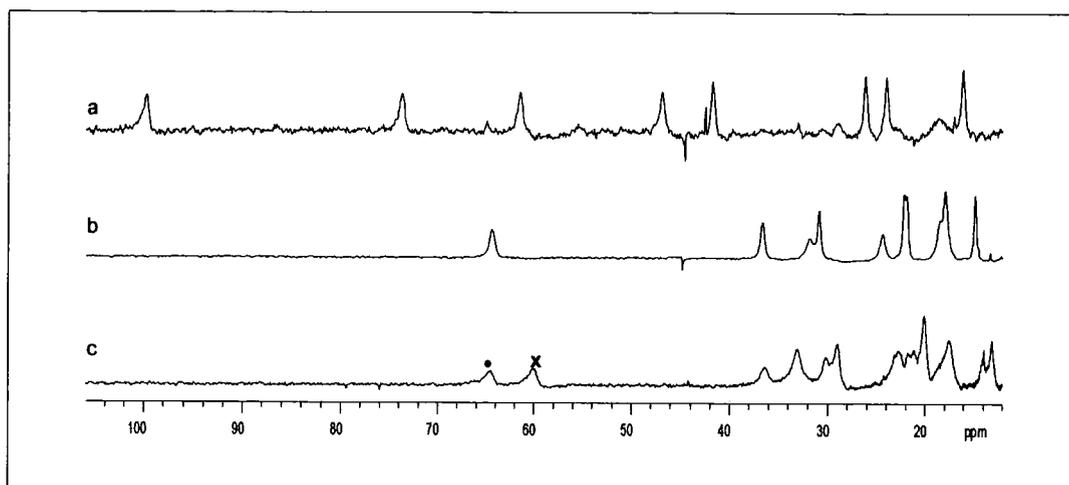
**Figure 3.18** Partial  $^1\text{H}$  NMR of (a)  $[\text{Yb.Ld}]$  **30** (diaqua species), (b) in the presence of 10 equivalents of (S)-alanine and (c) 10 equivalents of racemic alanine, showing the most shifted axial ring proton of the S ( $\bullet$ ) and R ( $\times$ ) adducts (200 MHz,  $\text{D}_2\text{O}/\text{CD}_3\text{OD}$ , 295 K,  $\text{pD} \sim 8$ ).
