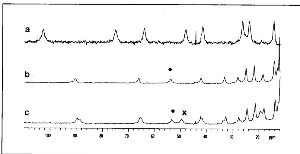
**Figure 3.14** Partial  $^1\text{H}$  NMR of (a)  $[\text{Yb.Lc}]^{3+}$  **14** (diaqua species), (b) in the presence of 2 equivalents of (S)-mandelic acid and (c) 2 equivalents of racemic mandelic acid, showing the proton resonances of the S (•) and R (x) adducts, which were used to assess the degree of enantioselectivity in the binding (200 MHz,  $\text{D}_2\text{O}/\text{CD}_3\text{OD}$ , 295 K).
