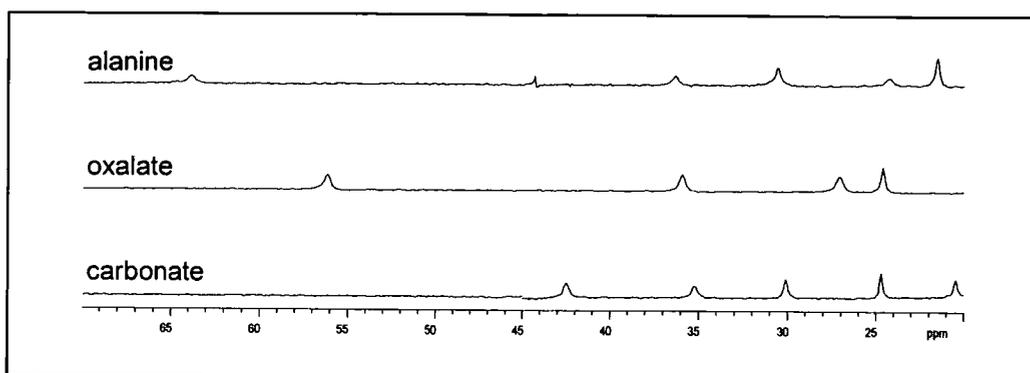
**Figure 3.5** Partial  $^1\text{H}$  NMR spectra for complexes of  $[\text{Yb.Ld}] \text{ 30}$  (10 mM) with the following added anions (ten-fold excess): alanine (pD 7.8); oxalate (pD 6.1); carbonate (pD 8.3); (200 MHz,  $\text{D}_2\text{O}$ , 295 K).
