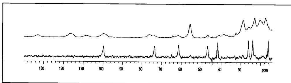
Figure 2.22 Partial  $^1\text{H}$  NMR spectra of [Yb.Ld] 30, showing the presence of dimers in a 10 mM solution of the complex (upper) and only one species in 1 mM solution (lower) (200 MHz,  $\text{D}_2\text{O}$ , 295 K).
