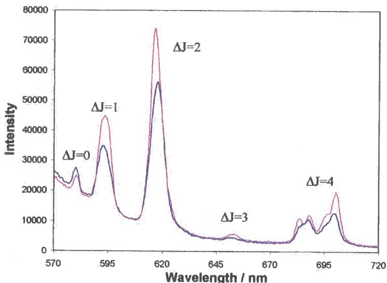
**Figure 2.34** Emission spectra of  $[\text{Eu.La}]^{3+}$  **13** (blue) and in presence of a 10 fold excess of added S-lactate (pink) ( $\lambda_{\text{ex}} = 254$  nm, 0.25 mM, pH 7.4, 0.1 M MOPS, 295 K).
