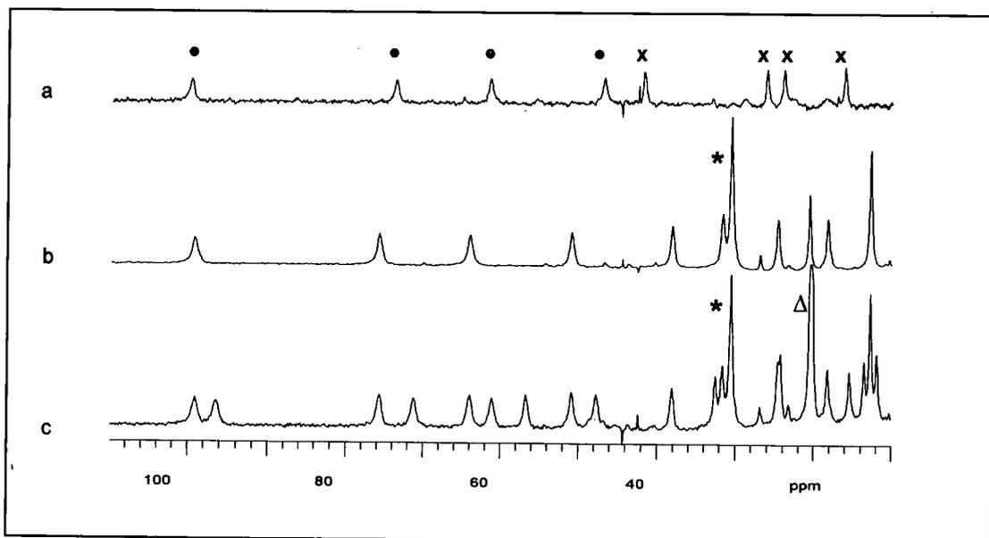
**Figure 2.23** Partial  $^1\text{H}$  NMR of (a) [Yb.Ld] **30** (1 mM) (diaqua species showing four axial (•) and four equatorial (x) ring protons), (b) in the presence of 1 equivalent of (S)-Lac [(+)- (S)-Lac CH<sub>3</sub>], and (c) 2 equivalents of racemic Lac [(Δ) (R)-Lac CH<sub>3</sub>] (200 MHz, D<sub>2</sub>O, 295 K).
