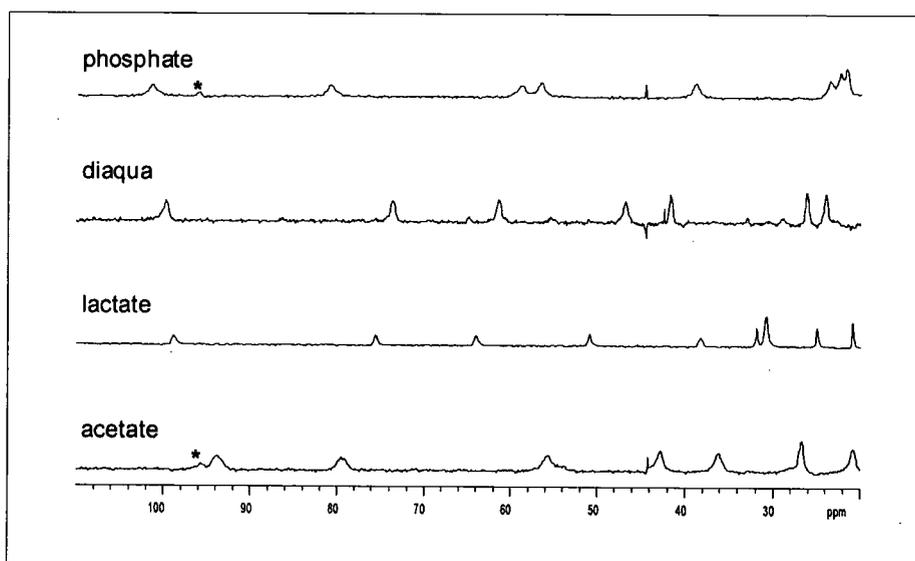
Figure 3.4 Partial <sup>1</sup>H NMR spectra for complexes of [Yb.Ld] 30 (10 mM) with the following added anions (ten-fold excess): HPO<sub>4</sub><sup>-</sup> (pD 8.7); water (pD 4.4, spectrum of the 1 mM solution); lactate (pD 6.2); acetate (pD 6.6); (200 MHz, D<sub>2</sub>O, 295 K). \*Impurity of the tetraalkylated complex (< 5%).
