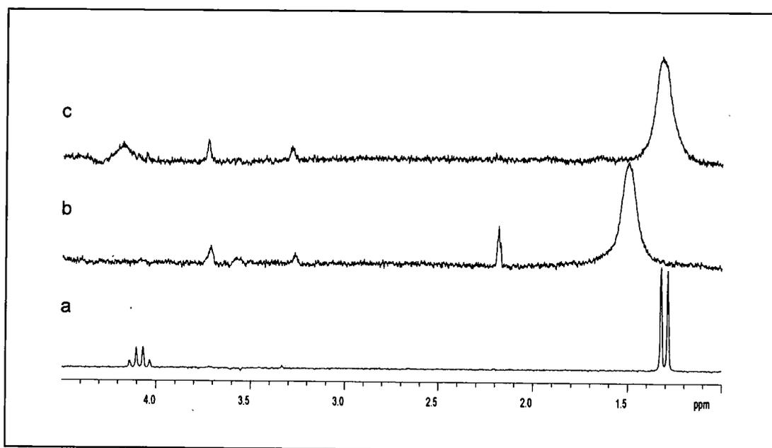
**Figure 2.31**  $^1\text{H}$  NMR spectra of a) S-lactate solution (10 mM), b) S-lactate solution +0.1 equivalents of  $[\text{Pr.Lc}]^{3+}$ , c) S-lactate solution +0.1 equivalents of  $[\text{Nd.Lc}]^{3+}$  (200 MHz,  $\text{D}_2\text{O}$ , 295 K).
