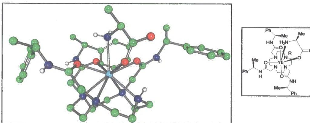
**Figure 3.15** Side view representation of  $(RRR)\text{-[Yb.DO3Ph-S-alanine]}^{2+}$  (SAP,  $\Lambda(\delta\delta\delta\delta)$ ) showing the amino acid NH occupying the axial position and a carboxylate O binding equatorially, completing the  $O_4$  plane.
