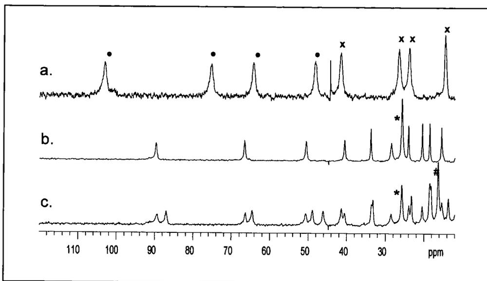
**Figure 2.18** Partial  $^1\text{H}$  NMR of (a)  $[\text{Yb.Lc}]^{3+}$  **14** (diaqua species showing four axial (•) and four equatorial (x) ring protons), (b) in the presence of 1 equivalent of (S)-Lac [(\*) (S)-Lac  $\text{CH}_3$ ], and (c) 2 equivalents of racemic Lac [(#) (R)-Lac  $\text{CH}_3$ ] (200 MHz,  $\text{D}_2\text{O}/\text{CD}_3\text{OD}$ , 295 K).
