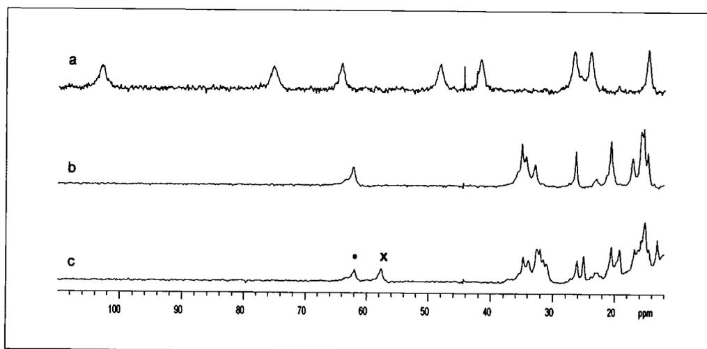
**Figure 3.19** Partial  $^1\text{H}$  NMR of (a)  $[\text{Yb.Lc}]^{3+}$  **14** (diaqua species), (b) in the presence of 10 equivalents of (S)-methionine and (c) 10 equivalents of racemic methionine, showing the most shifted axial ring proton of the S (•) and R (x) adducts (200 MHz,  $\text{D}_2\text{O}/\text{CD}_3\text{OD}$ , 295 K, pD  $\sim$ 8).
