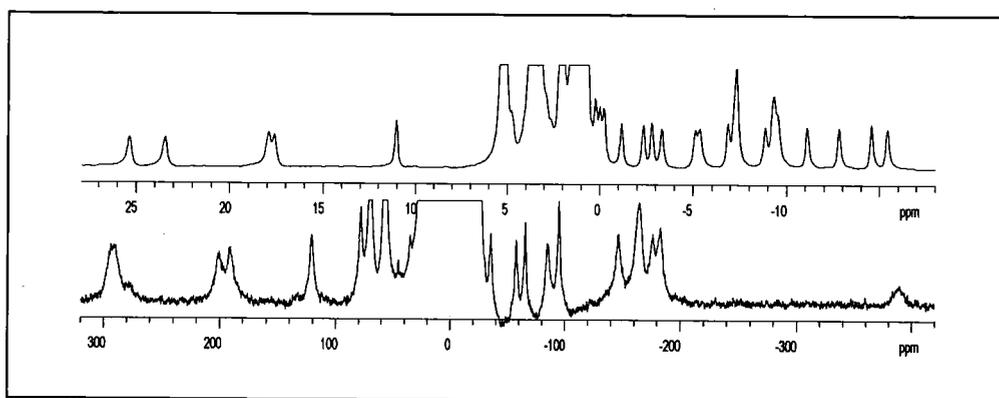
**Figure 2.30**  $^1\text{H}$  NMR spectra of  $[\text{Eu.Ld}]$  **35** (200 MHz,  $\text{CD}_3\text{OD}$ , 295 K) (upper) and  $[\text{Tm.Ld}]$  **40** (65 MHz,  $\text{CD}_3\text{OD}$ , 295 K) (lower), highlighting the greater shifting and broadening ability of the  $\text{Tm}^{3+}$  ion compared to the  $\text{Eu}^{3+}$  ion.
