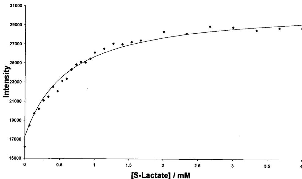
**Figure 2.39** Variation of  $\text{Eu}^{3+}$  emission intensity (614 nm) for  $[\text{Eu.Lc}]^{3+}$  **19** as a function of added S-lactate (1 mM complex, pH 7.4, 0.1 M MOPS, 295 K), showing the fit to the experimental data points.
