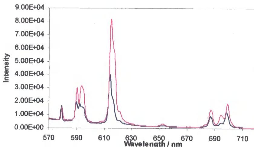
**Figure 2.38** Emission spectra of the zwitterionic [Eu.Ld] **35** (blue) and in the presence of a 10 fold excess of S-lactate (pink) ( $\lambda_{\text{ex}} = 397$  nm, 2.5 mM, pH 7.4, 0.1 M MOPS, 295 K).
