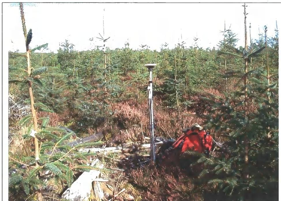
Figure 3.6 Differential GPS measurement of sample plot centre.
