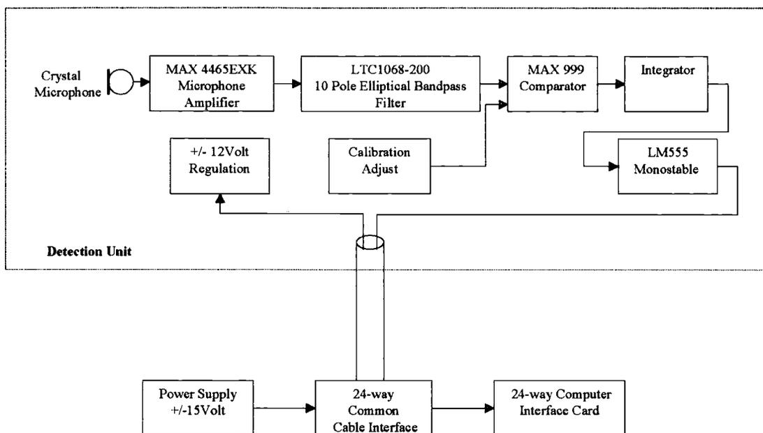
Fig 5.1 Schematic of actograph detection unit
