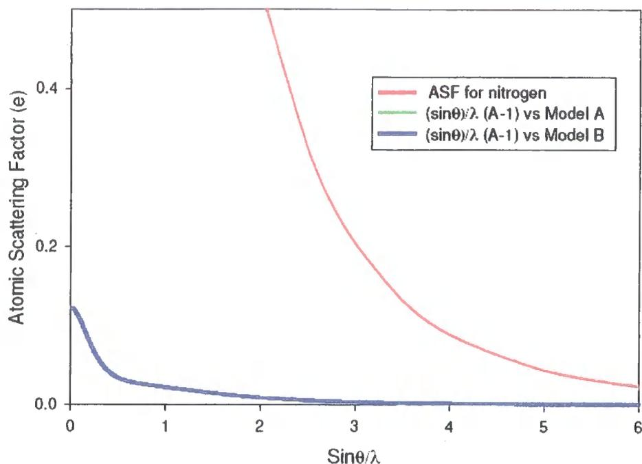
**Figure A3.1.2:** Graph showing the effect of multiplying the atomic scattering factor (ASF) for nitrogen by a Bessel function. The ASF for models A and B overlay each other, and for this reason their graphs cannot be resolved.
