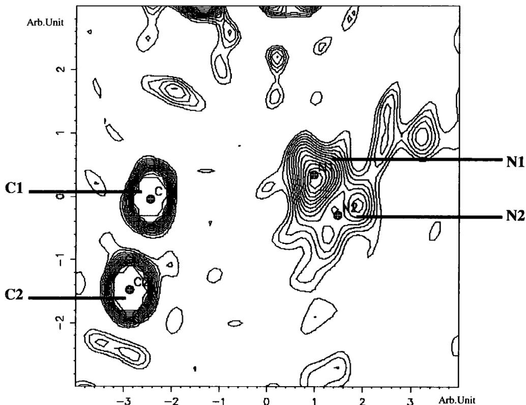
**Figure 5.3.9:** Slant-plane  $F_{\text{obs}}$  Fourier map defined by atoms N1, N2, and C1. The contour range is set to 0-5 eÅ<sup>3</sup> and the contour level is set to 0.3125 eÅ<sup>3</sup>.
