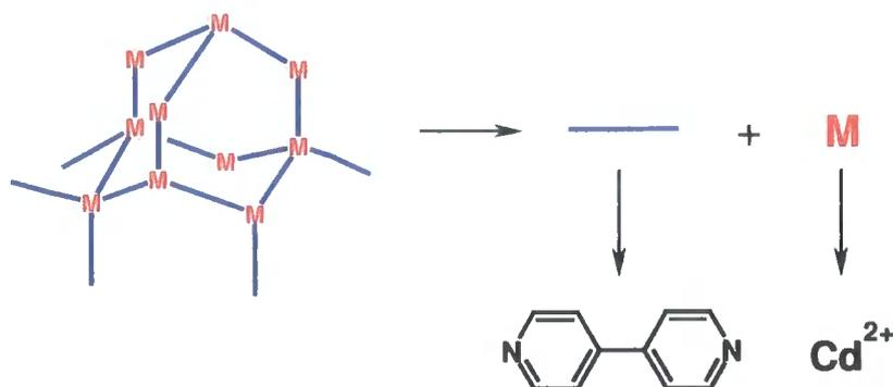
**Figure 4.1.1:** Simplistic representation of the design strategy for a framework with a diamond topology (left). The structure can be regarded as being composed of linear linker molecules (—) coordinated to metal ions (M) with tetrahedral coordination geometry. The chemical precursors for this structure may be the linear 4,4'-bipyridine ligand and a metal species that typically adopts a tetrahedral geometry such as Cd(II) or Zn(II).
