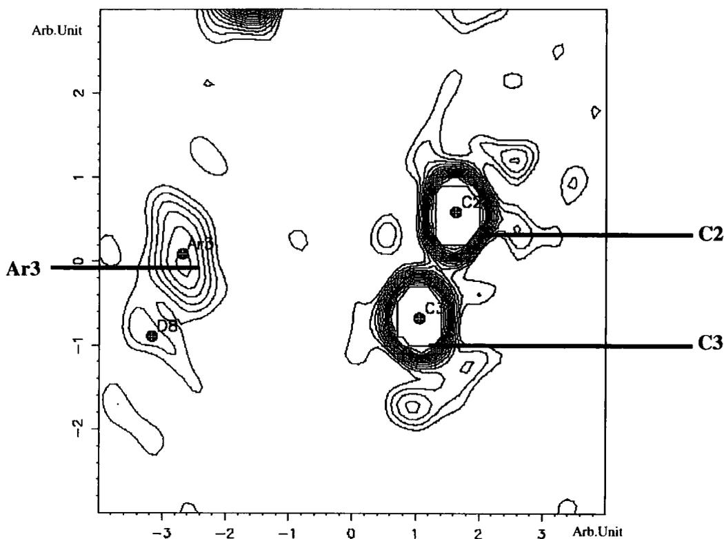
**Figure 5.3.23:** Slant-plane  $F_{\text{obs}}$  Fourier map defined by atoms C2, C3, and Ar3. The contour level is set to  $0.25 \text{ e}\text{\AA}^3$  and the range is  $0\text{-}4 \text{ e}\text{\AA}^3$ .
