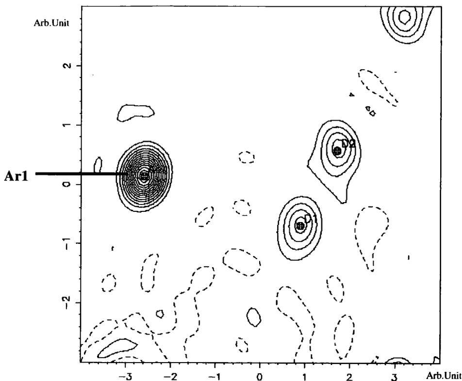
**Figure 5.3.34:** Slant-plane  $F_{\text{obs}}$  Fourier map. Atoms D1, D2, and Ar1 define the plane of the map. The contour range is  $-5.639$ - $49.077 \text{ e}\text{\AA}^3$ , and the contour level is set to  $3.4197 \text{ e}\text{\AA}^3$ .
