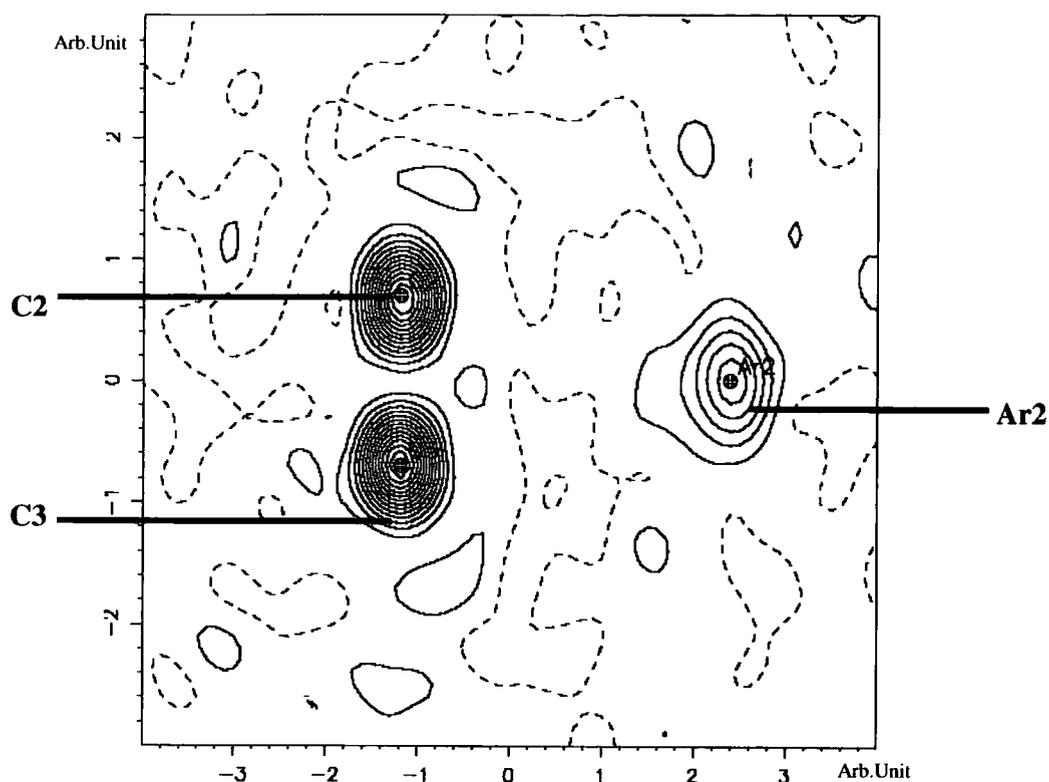
**Figure 5.3.35:** Slant-plane  $F_{\text{obs}}$  Fourier map. Atoms C2, C3, and Ar2 define the plane of the map. The contour range is  $-1.514\text{--}14.982\text{ e}\text{\AA}^3$ , and the contour level is set to  $1.0309\text{ e}\text{\AA}^3$ .
