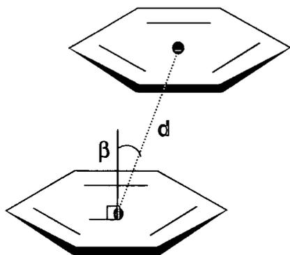
**Figure A2.1.4:** Diagram to illustrate the geometrical parameters associated with  $\pi\cdots\pi$  interactions. The  $\beta$ -angle gives an indication as to the degree of ring slippage from the totally eclipsed arrangement, and 'd' is the distance between ring centroids.
