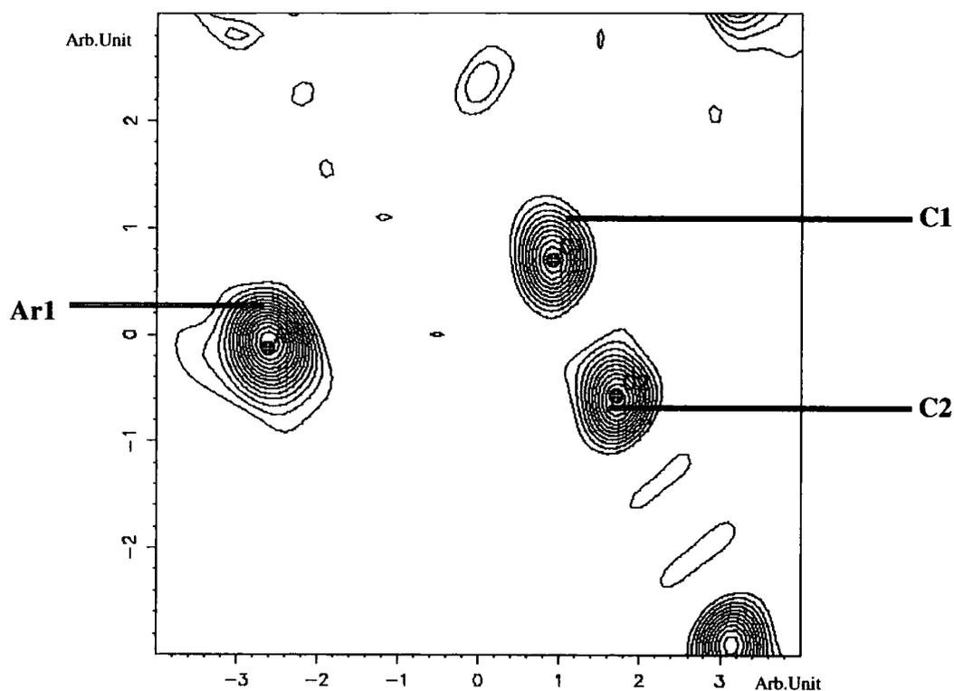
**Figure 5.3.21:** Slant-plane  $F_{\text{obs}}$  Fourier map defined by atoms Ar1, C1, and C2. Contour range is set to 0-17.44  $\text{e}\text{\AA}^3$  and the contour level is set to 1.09  $\text{e}\text{\AA}^3$ .
