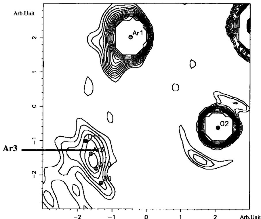
**Figure 5.3.24:** Slant-plane Fourier map defined by atoms Ar3, Ar1, and O2. This diagram shows the relative positions of the dummy atoms D9, D10 and D11. The contour level is set to 0.3636 eÅ<sup>3</sup> and the range is 0-4 eÅ<sup>3</sup>.
