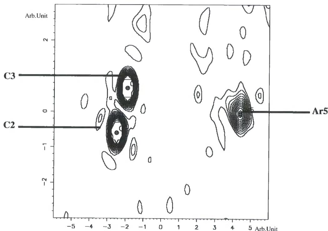
**Figure 5.3.38:** Slant-plane  $F_{\text{obs}}$  Fourier map. Atoms C2, C3, and Ar5 define the plane of the map. The contour range is 0-7  $\text{e}\text{\AA}^3$ , and the contour level is set to 0.4375  $\text{e}\text{\AA}^3$ .
