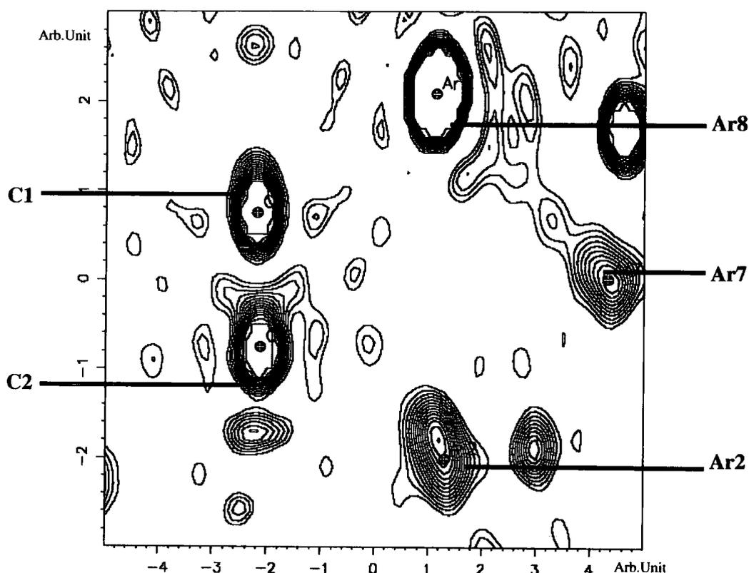
**Figure 5.3.40:** Slant-plane  $F_{\text{obs}}$  Fourier map. Atoms C1, C2, and Ar7 define the plane of the map. The contour range is  $0-7 \text{ e\AA}^3$ , and the contour level is set to  $0.4375 \text{ e\AA}^3$ .
