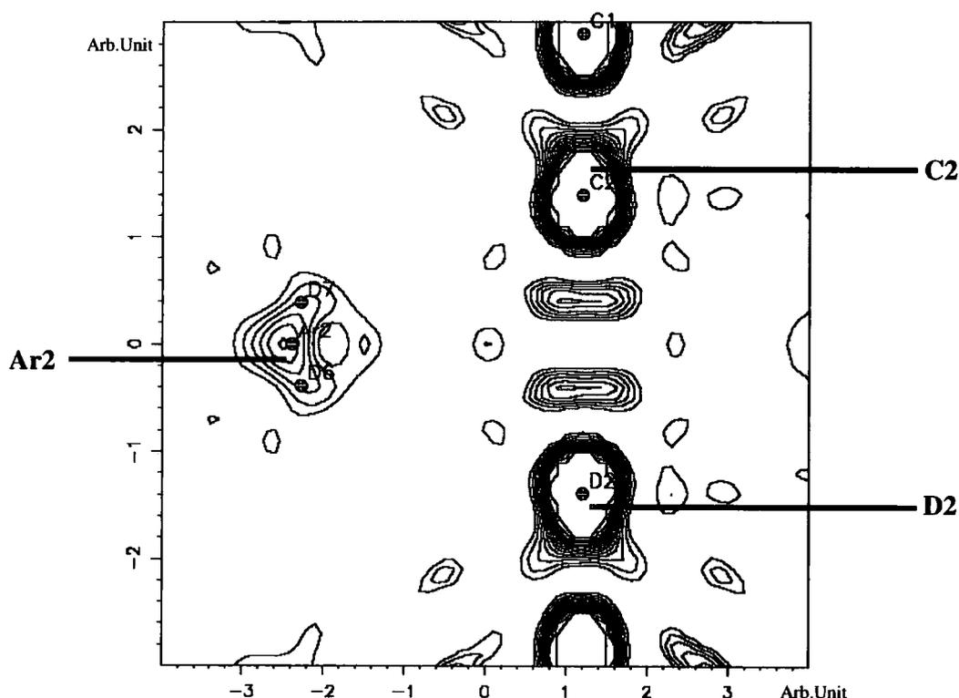
**Figure 5.3.22:** Slant-plane  $F_{\text{obs}}$  map. Atoms C2, D2, and Ar2 define the plane. The contour level is set to  $0.3636 \text{ e}\text{\AA}^3$  and the range is  $0\text{--}4 \text{ e}\text{\AA}^3$ .
