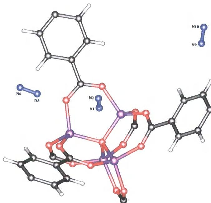
**Figure 5.3.16:** Location of the three nitrogen molecules absorbed at 30K relative to the Zn<sub>4</sub>O(BDC) framework (Zn: purple, O: red, C: black, N: blue, H: grey).
