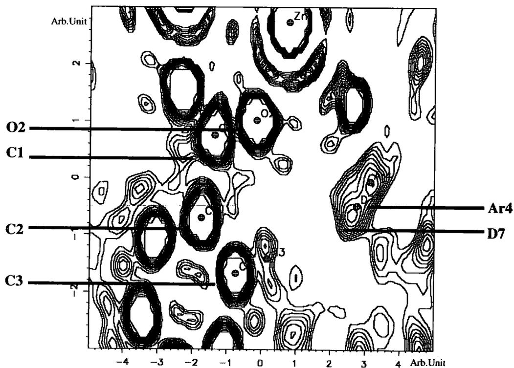
**Figure 5.3.37:** Slant-plane  $F_{\text{obs}}$  Fourier map. Atoms C1, C2, and Ar4 define the plane of the map. The contour range is 0-5  $\text{e}\text{\AA}^3$ , and the contour level is set to 0.3125  $\text{e}\text{\AA}^3$ .
