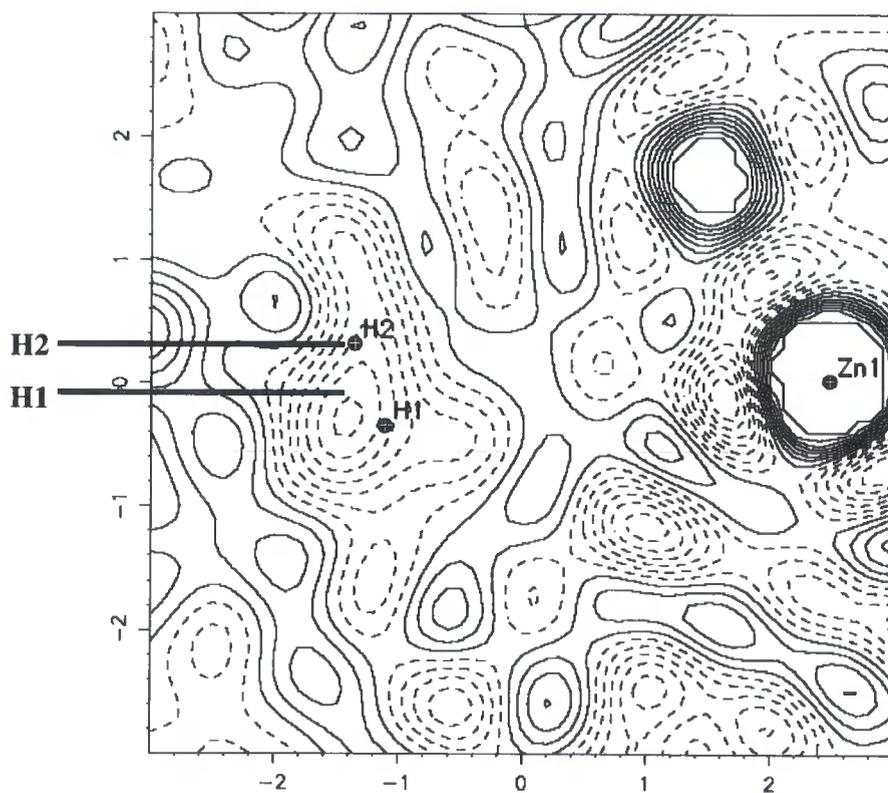
**Figure 6.3.7:** Slant plane neutron Fourier map defined by atoms H1, H2, and Zn1. The contour range is 5.0 – (-5.392) cm<sup>Å</sup><sup>2</sup>, and the level is set to 0.6495 cm<sup>Å</sup><sup>2</sup>.
