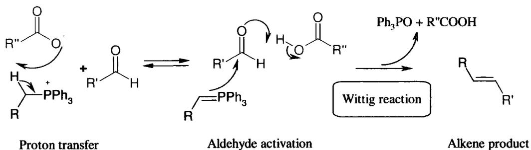
**Figure 3.1.4:** Mechanism of aldehyde activation by an acid catalysis. The species in red and blue are the ylide counterion and aldehyde respectively. Diagram adapted from Hon *et al.*<sup>[18]</sup>
