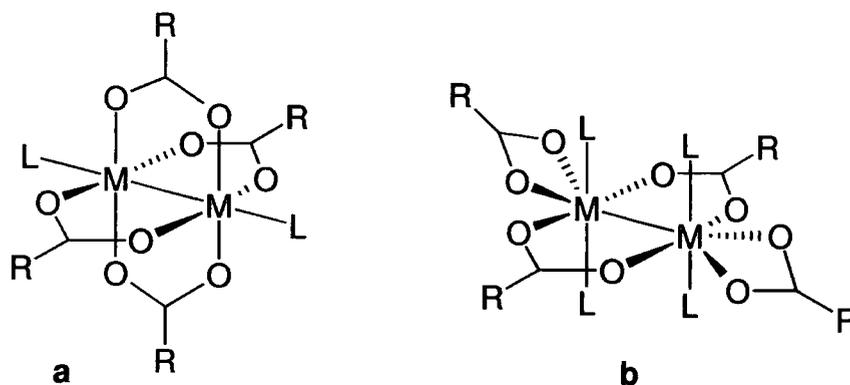
**Figure 4.1.4:** (a) The ‘lantern-like’ structure often seen in metal-BDC coordination polymers. (b) Prismatic dinuclear unit. R = benzene ring, L = additional ligand bound to the metal, M = metal site.
