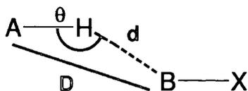
**Figure A2.1.2:** Schematic showing the geometric parameters for a hydrogen bond.
