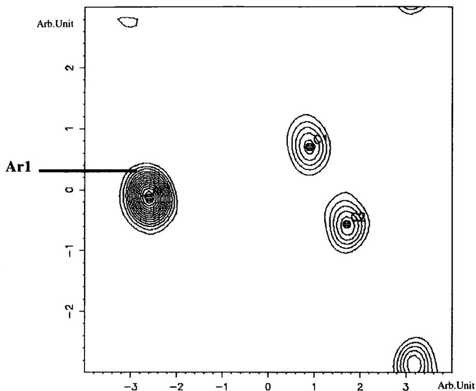
**Figure 5.3.27:** Slant-plane Fourier map defined by atoms Ar1, C1, and C2. The contour range is 0-38.14 eÅ<sup>3</sup>, and contour level is set to 2.3835 eÅ<sup>3</sup>.
