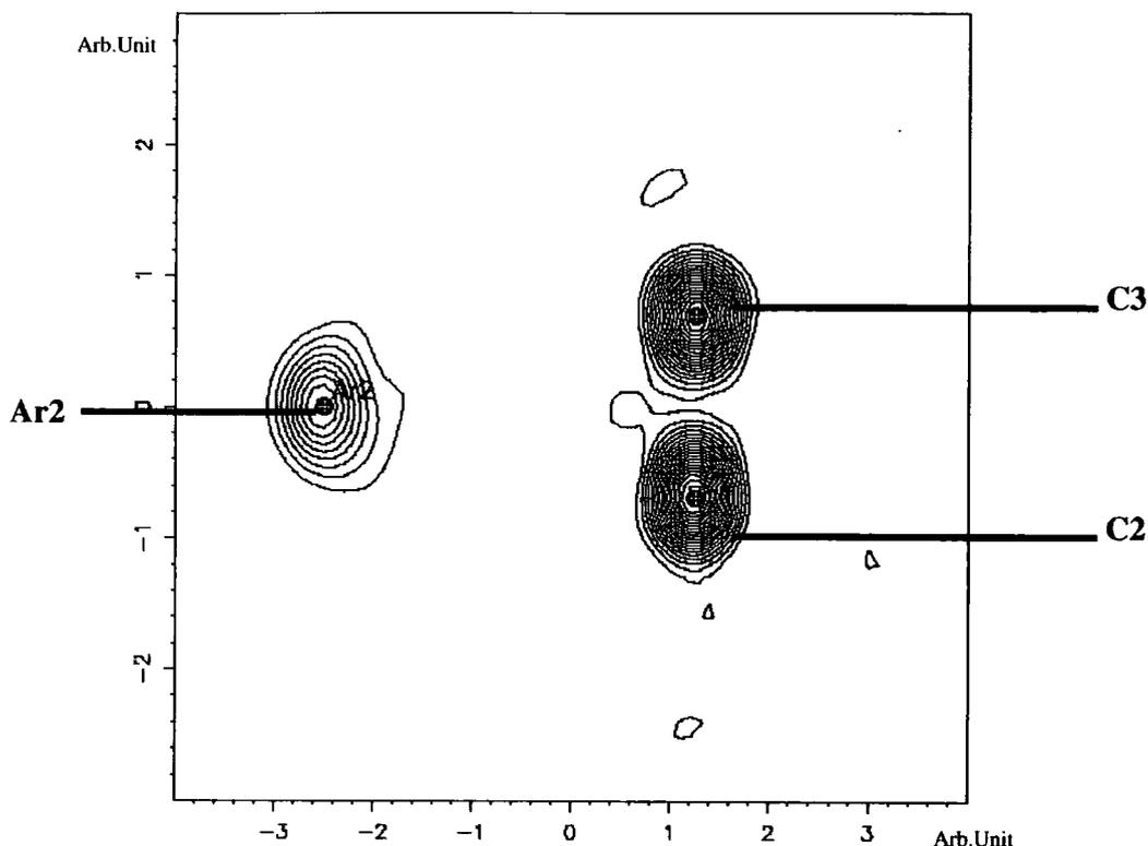
**Figure 5.3.28:** Slant-plane  $F_{\text{obs}}$  Fourier map defined by atoms Ar2, C2, and C3. The contour range is set to 0-14.88  $\text{e}\text{\AA}^3$ , and contour level to 0.7085  $\text{e}\text{\AA}^3$ .
