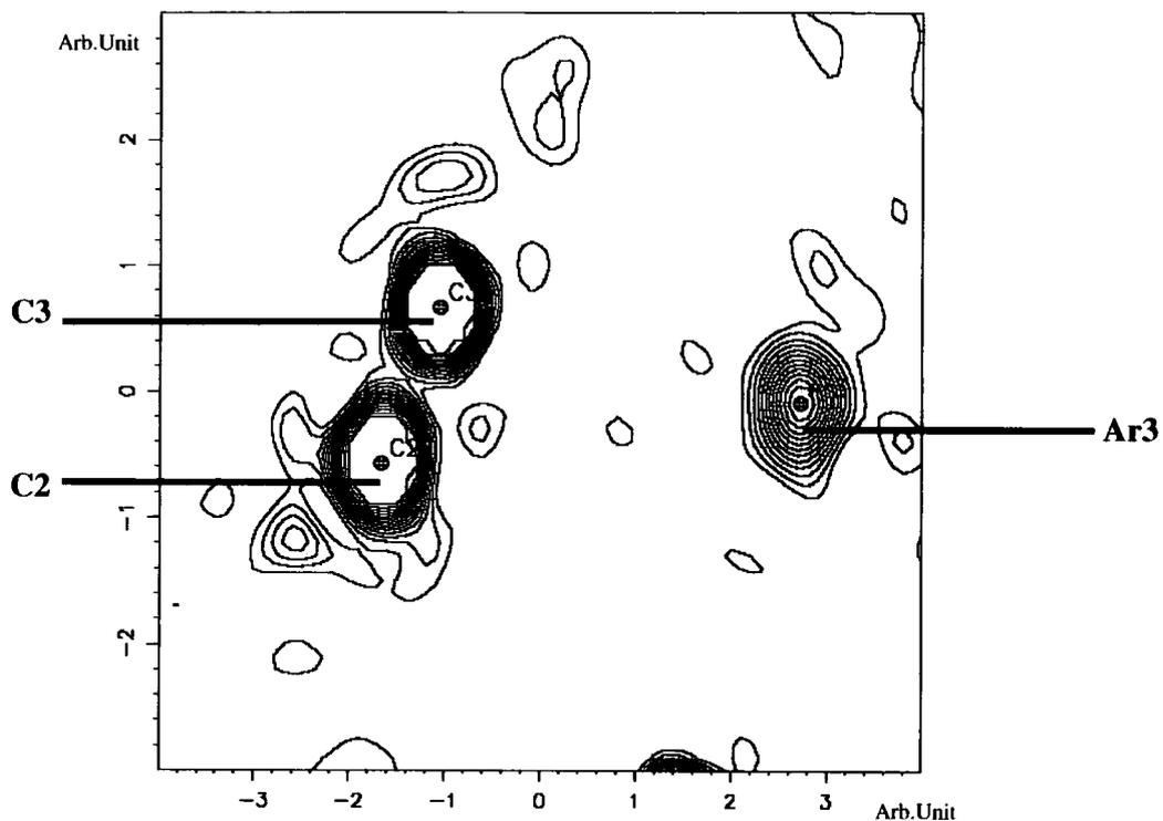
**Figure 5.3.29:** Slant-plane  $F_{\text{obs}}$  Fourier map defined by atoms Ar3, C2, and C3. The contour range is set to 0-5 eÅ<sup>3</sup>, and contour level to 0.3125 eÅ<sup>3</sup>.
