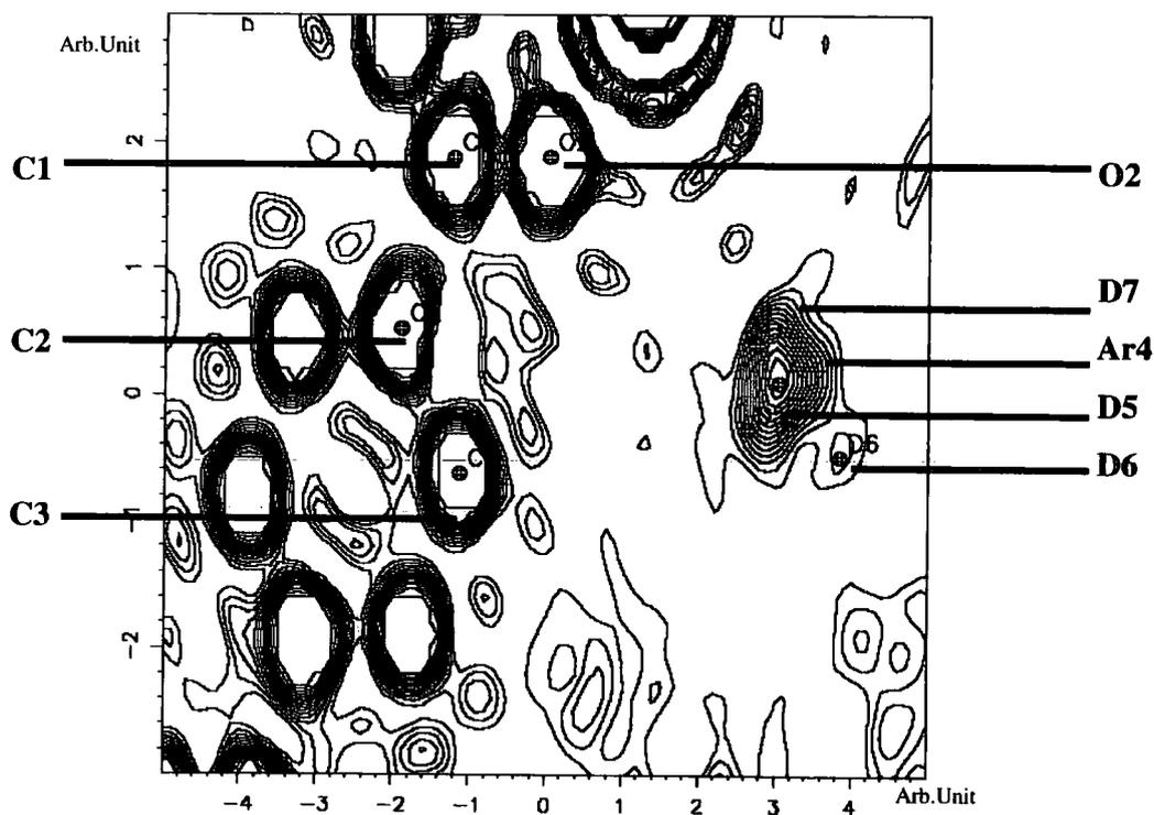
**Figure 5.3.30:** Slant-plane  $F_{\text{obs}}$  Fourier map defined by atoms Ar4, C2, and C3. The contour range is set to 0-5 eÅ<sup>3</sup>, and contour level to 0.3125 eÅ<sup>3</sup>.
