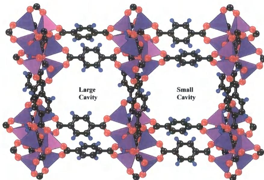
**Figure 4.1.3:** Diagram displaying the two cavity types present in the  $Zn_4O(BDC)$  framework. For clarity the hydrogen atoms are shown in blue.
