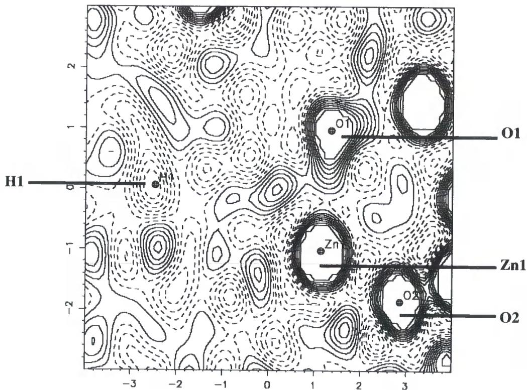
**Figure 6.3.2:** Slant plane neutron  $F_{\text{obs}}$  map defined by atoms H1, O1, and Zn1. The contour range is  $5.0 - (-5.109) \text{ cm}\text{\AA}^2$ , and the level is set to  $0.6318 \text{ cm}\text{\AA}^2$ .
