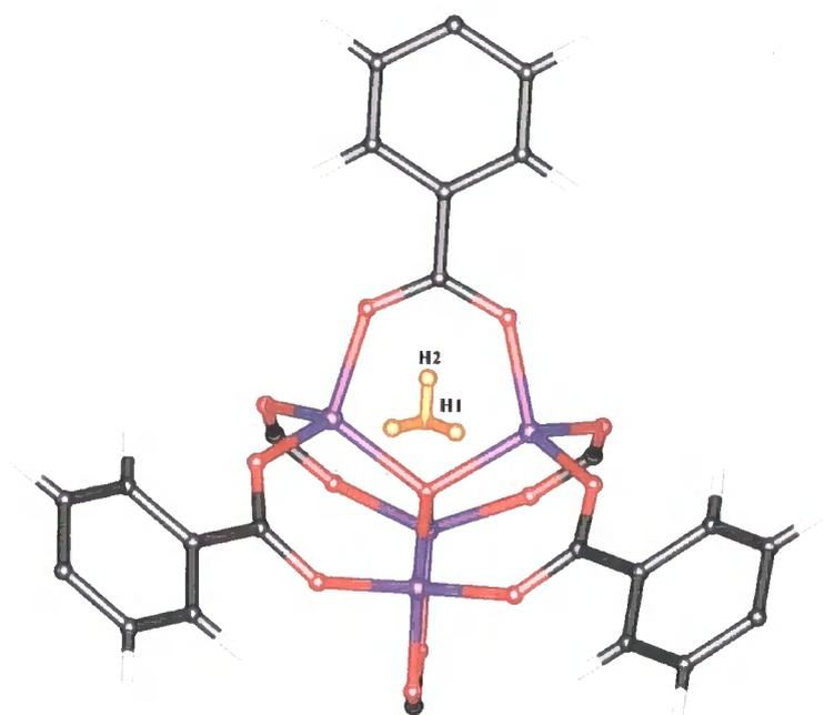
**Figure 6.3.4:** Diagram showing the location of molecule H1-H2 relative to the framework atoms at 50K. Zn: purple; O: red; C: black; framework hydrogen: grey; absorbed hydrogen: yellow. Only one position of the disordered H2 atom is labelled for clarity.
