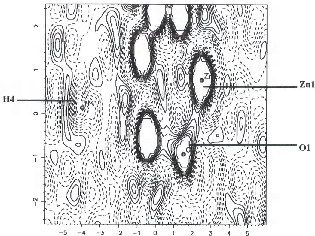
**Figure 6.3.9:** Slant plane neutron Fourier map defined by atoms H4, O1, and Zn1. The contour range is  $5.0 - (-5.961) \text{ cm}\text{\AA}^2$ , and the level is set to  $0.6850 \text{ cm}\text{\AA}^2$ .
