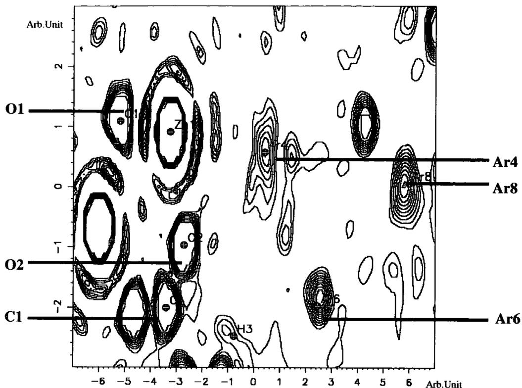
**Figure 5.3.41:** Slant-plane  $F_{\text{obs}}$  Fourier map. Atoms Zn1, O2, and Ar8 define the plane of the map. The contour range is 0-5  $\text{e}\text{\AA}^3$ , and the contour level is set to 0.4545  $\text{e}\text{\AA}^3$ .
