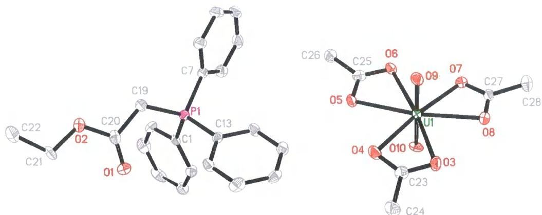
**Figure 3.3.13:** Molecular structure of the salt  $[\text{H-EPPY}]^+[\text{UO}_2(\text{CH}_3\text{COO})_3]^-$  (**9**). Thermal displacement ellipsoids are drawn at the 50% probability level.
