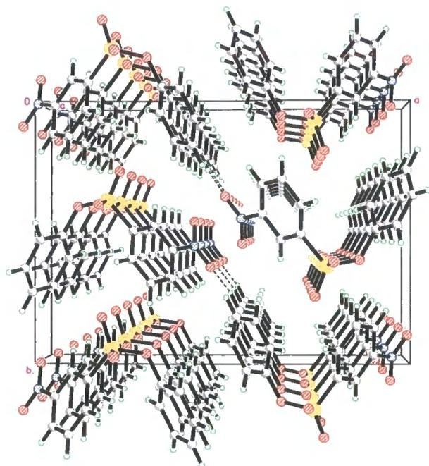
**Figure 2.3.5:** Packing diagram for compound **2** as viewed along the *c*-axis. The dashed lines indicate the C10-H10...O1<sup>IV</sup> interaction.
