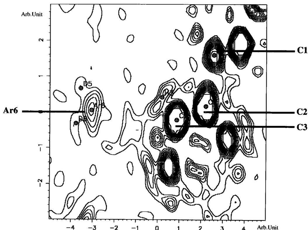
**Figure 5.3.39:** Slant-plane  $F_{\text{obs}}$  Fourier map. Atoms C2, C3 and Ar6 define the plane of the map. The contour range is  $0\text{-}5 \text{ e\AA}^3$ , and the contour level is set to  $0.3125 \text{ e\AA}^3$ .
