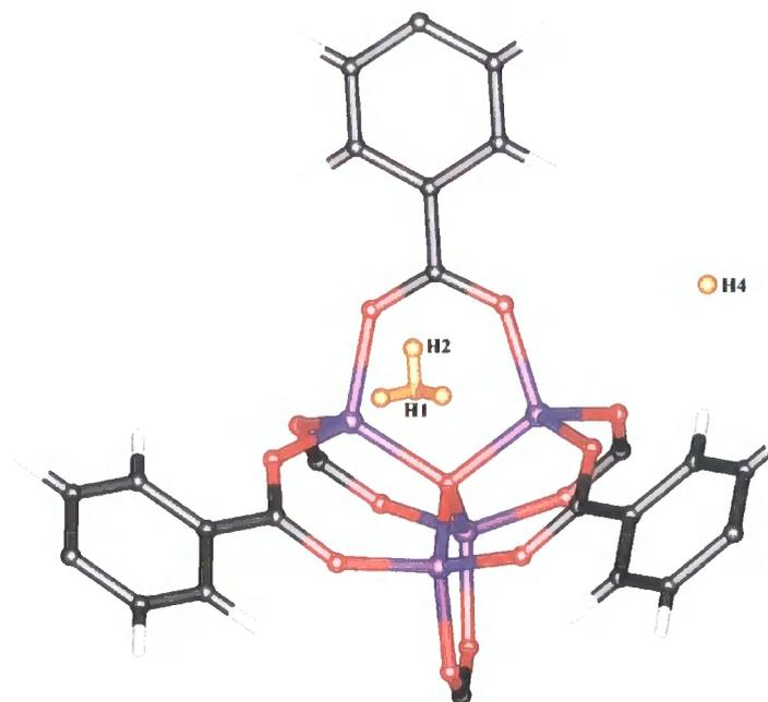
**Figure 6.3.6:** Diagram showing the location of the hydrogen molecules relative to the framework atoms at 5K. Zn: purple; O: red; C: black; framework hydrogen: grey; adsorbed hydrogen: yellow. Only one position of the disordered H2 atom is labelled for clarity.
