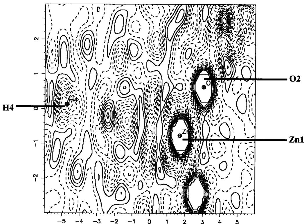
**Figure 6.3.8:** Slant plane neutron Fourier map defined by atoms H4, O2, and Zn1. The contour range is 5.0 – (-5.927) cm<sup>Å</sup><sup>2</sup>, and the level is set to 0.6829 cm<sup>Å</sup><sup>2</sup>.
