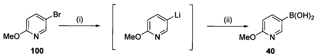
Scheme 2.2a: 2-Methoxy-5-pyridylboronic acid synthesis. Reagents and Conditions: (i) n -BuLi, Et 2 O, -78 °C, (ii) 1. TPB, -78 °C, 2. aqueous work-up.
