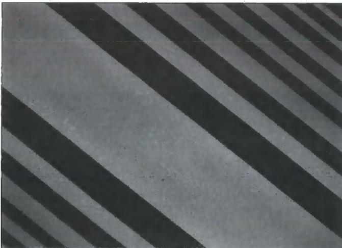
Figure 3.36: A CGH photo-reduced x25 from a laser-plotted master
