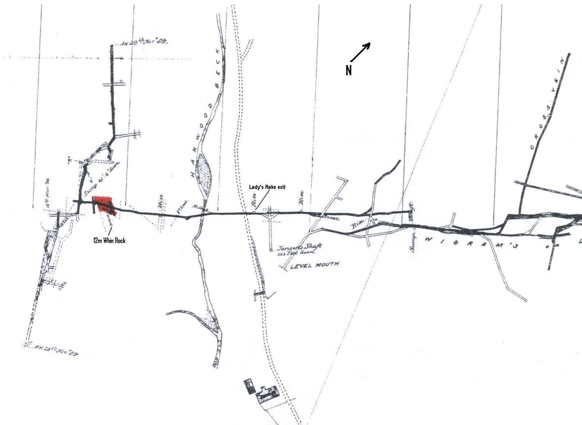
**Fig.42. Mine drawing showing a 12m wide intrusive 'hard' rock encountered by 19th century miners near Lady's Rake mine**
