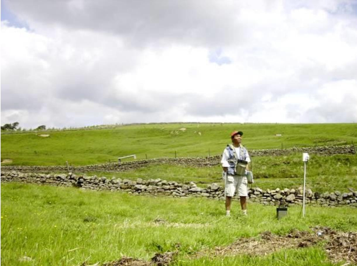
**Plate2. Magnetic survey equipment; magnetometer sensor on its pole attached to the meter itself and the GPS antenna held vertically by hand (Burtreeford fold-axis in the background).**
