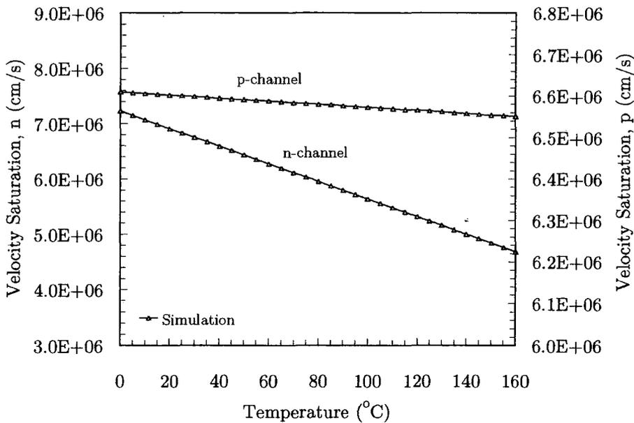
Figure 3.14: Velocity saturation as function of temperature
