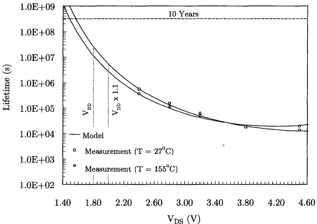
Figure 6.14: Hot-carrier lifetime (n-channel)
