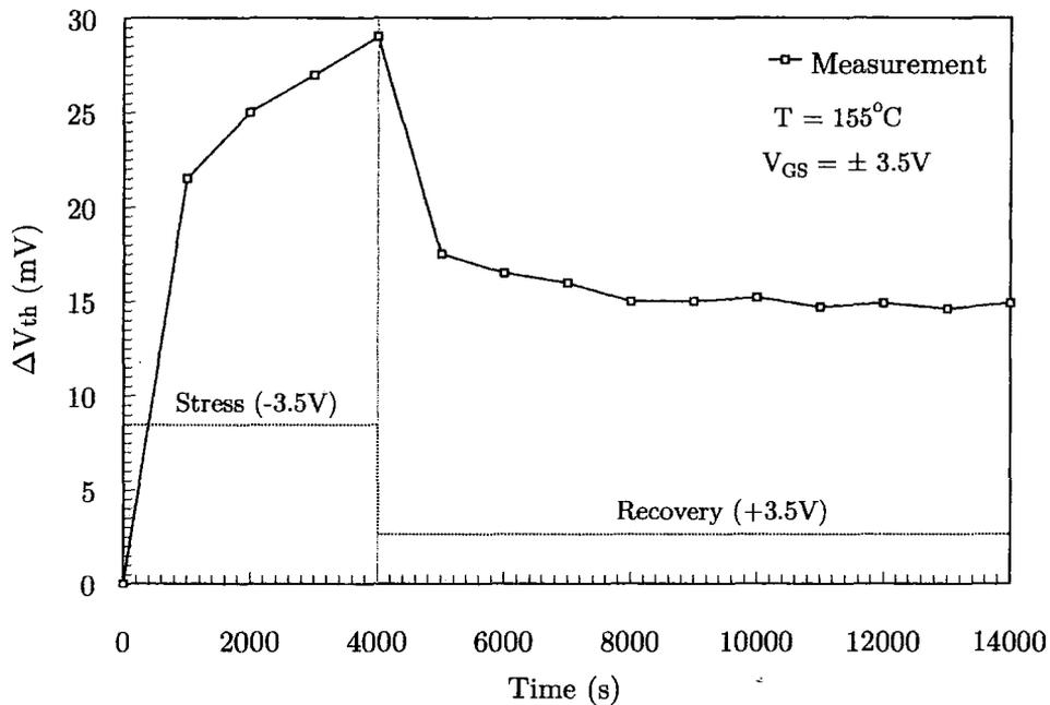
Figure 4.7: Threshold voltage recovery after NBTI stress
