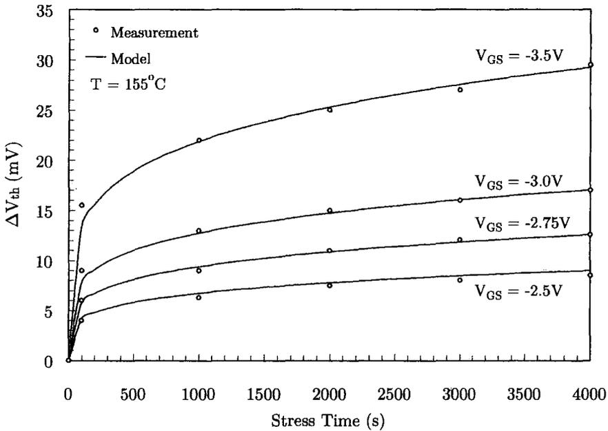
Figure 4.4: Threshold voltage shift under DC stress
