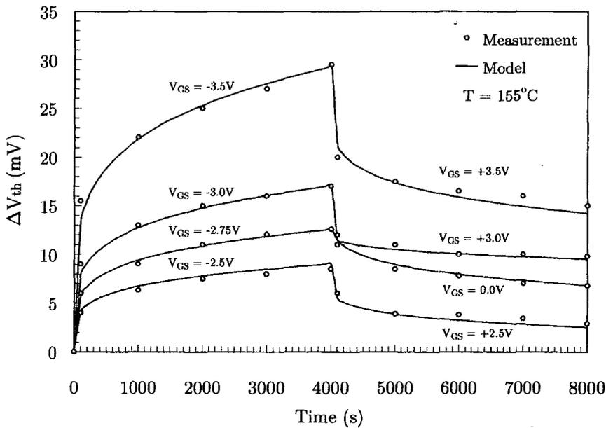
Figure 4.9: Comparison between NBTI model and experimental results
