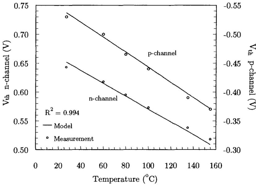
Figure 3.16: Threshold voltage as a function of temperature
