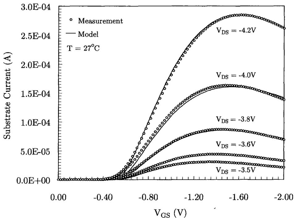
Figure 6.7: Substrate current versus gate voltage (p-channel)
