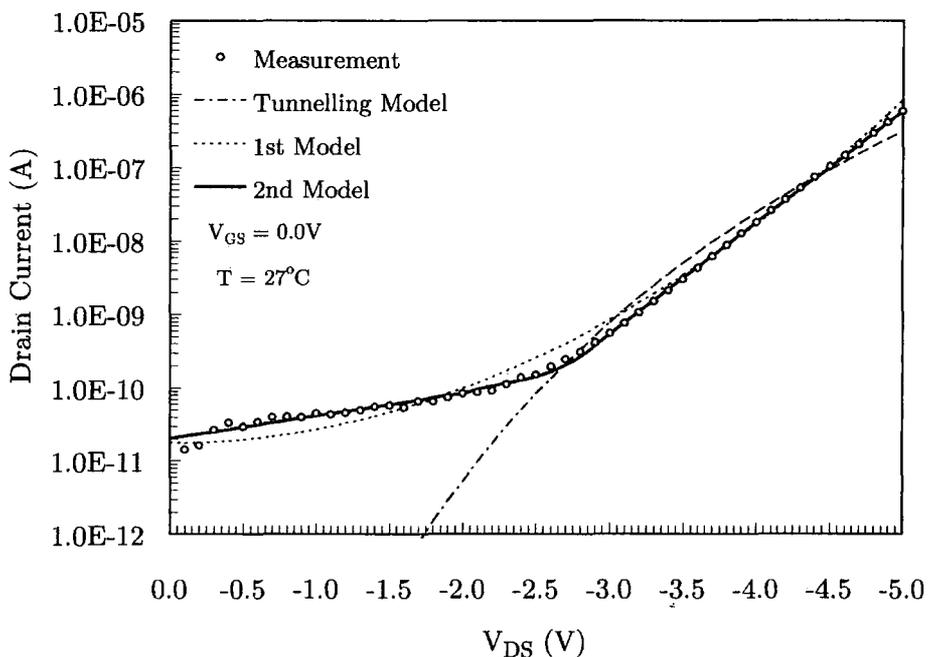
Figure 5.6: Comparison of GIDL model with 1st design
