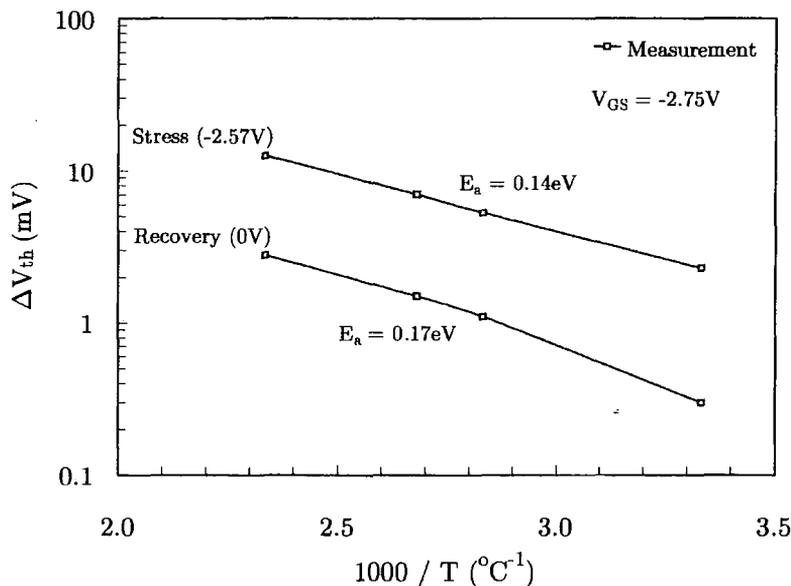
Figure 4.10: Comparison between stress and recovery activation energies
