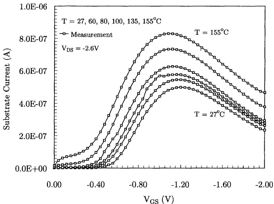
Figure 6.10: Substrate current at various temperatures (low  $V_{DS}$ )
