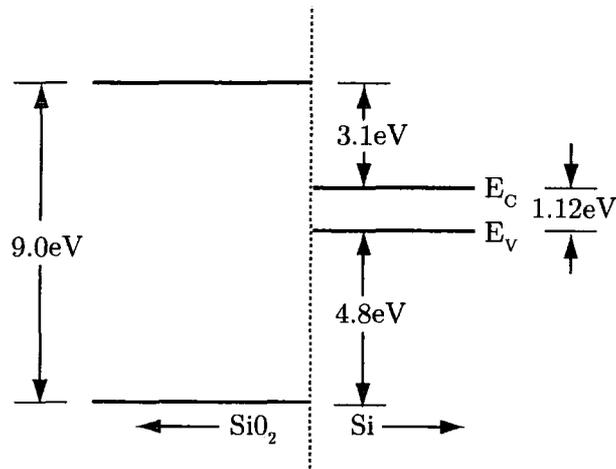
Figure 6.2: Illustration of silicon-oxide interface energy bands
