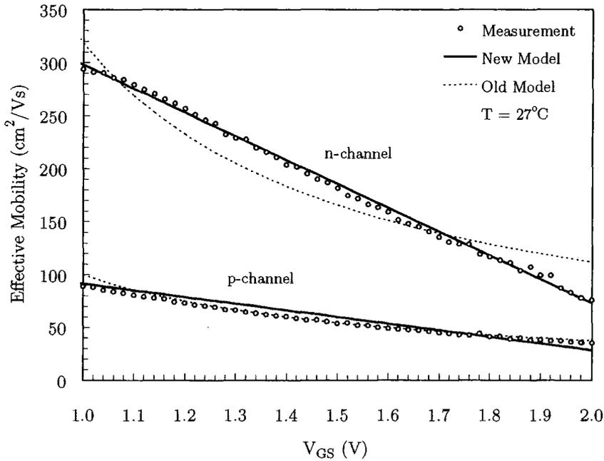
Figure 3.5: Mobility as a function of gate voltage
