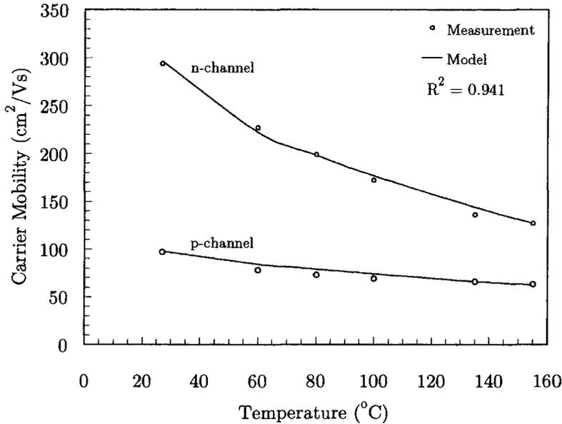
Figure 3.13: Carrier mobility as function of temperature
