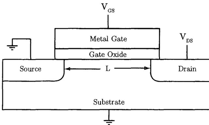
Figure 3.4: MOSFET gate construction
