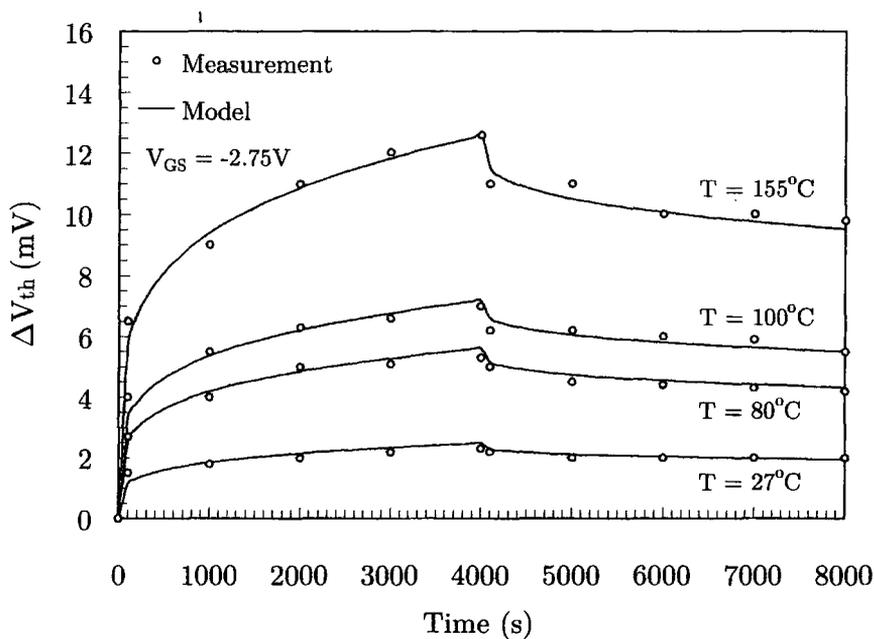
Figure 4.11: Temperature dependence of NBTI stress and recovery
