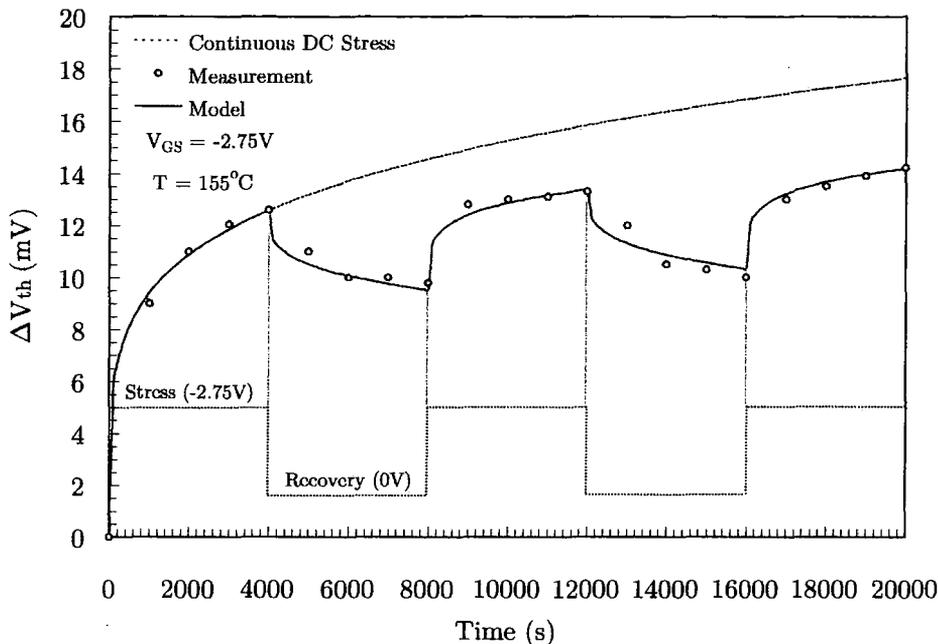
Figure 4.12: NBTI lock-in illustration
