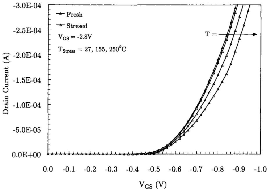
Figure 7.10: NBTI stress simulation at varied temperatures
