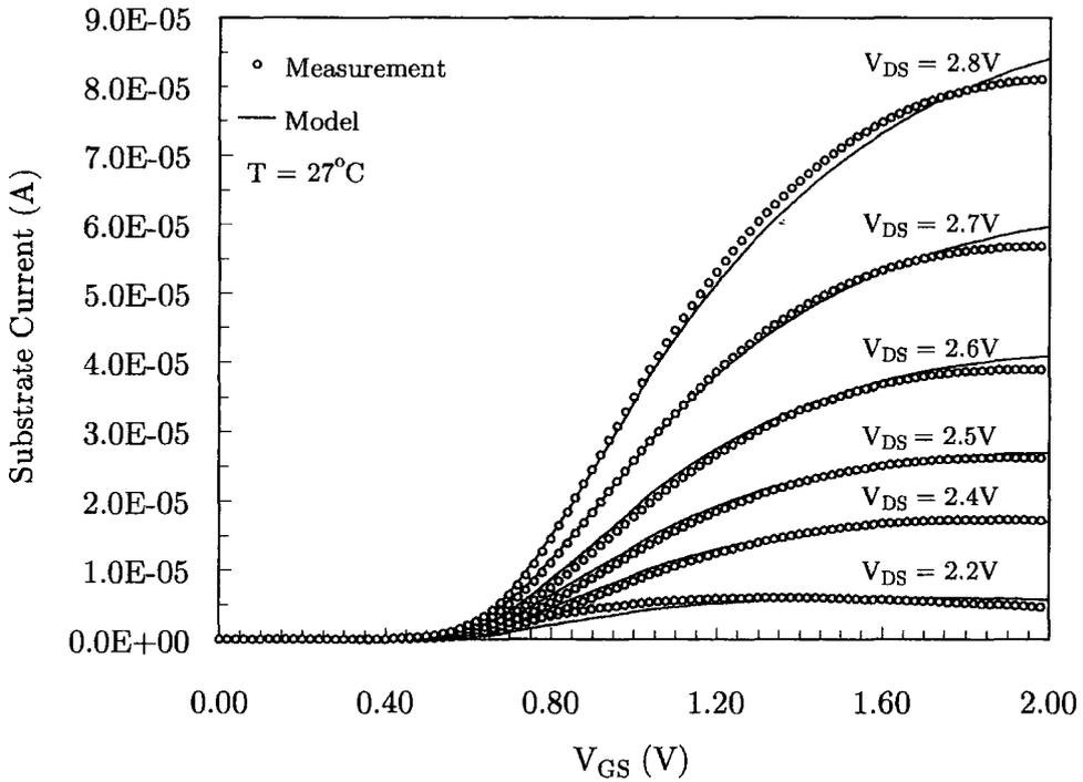
Figure 6.6: Substrate current versus gate voltage (n-channel)
