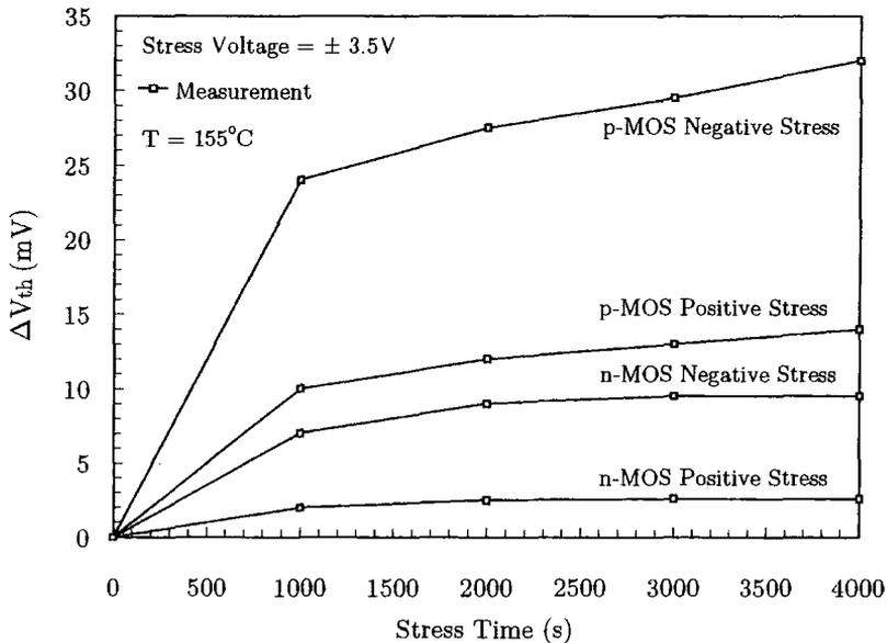
Figure 4.2: NBTI n-channel and p-channel degradation comparison
