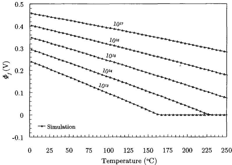
Figure 3.15: Fermi potential as a function of temperature
