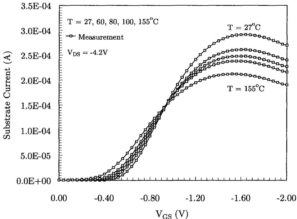
Figure 6.9: Substrate current at various temperatures (high  $V_{DS}$ )
