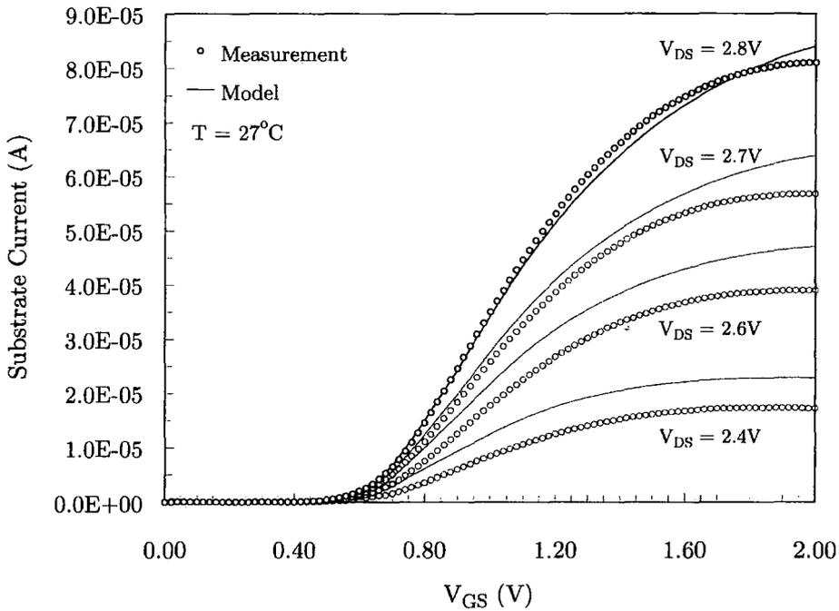
Figure 6.5: Inaccuracy in substrate current prediction (n-channel)
