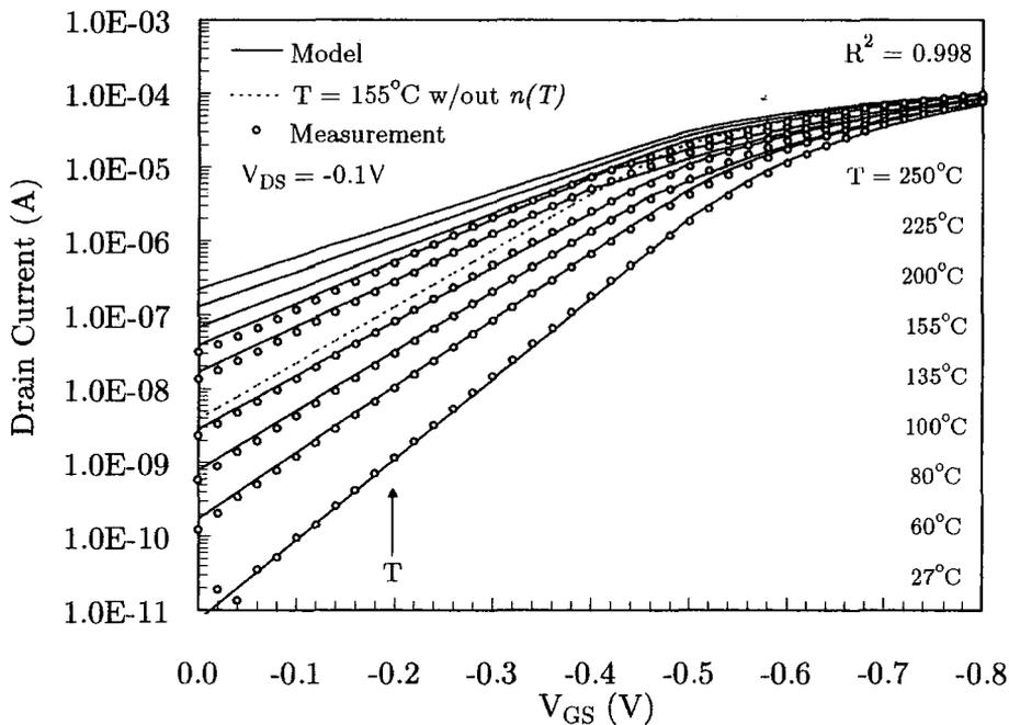
Figure 3.17: Temperature dependence of the subthreshold region (p-channel)
