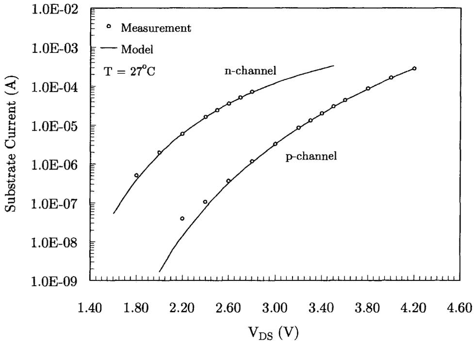
Figure 6.8: Comparison between n- and p-channel substrate currents
