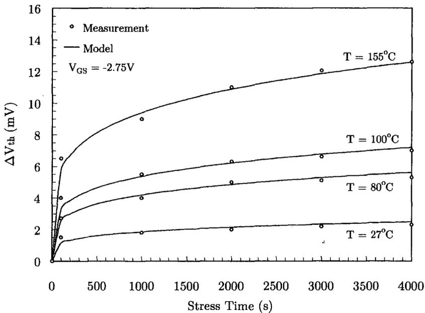
Figure 4.5: NBTI stress as a function of temperature
