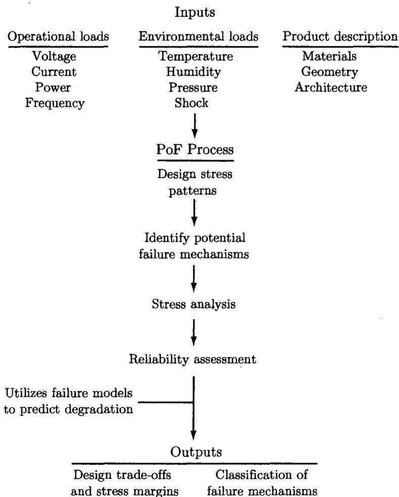
Figure 2.4: Physics of failure process
