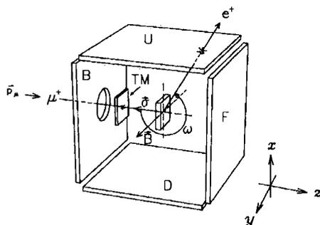
Figure 3.10: The scintillator arrangement for a continuous source the detectors are labeled, forward (F), backward (B), up (U) and down (B). Application of a magnetic field ( $B$ ) perpendicular to the beam will cause muon precession. TM is the scintillator switch to start the timing of the muon decay[7].
