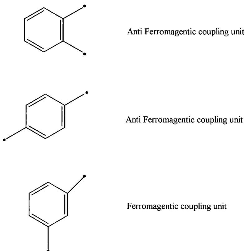
Figure 7.2: The aromatic coupling unit of connected biradicals.
