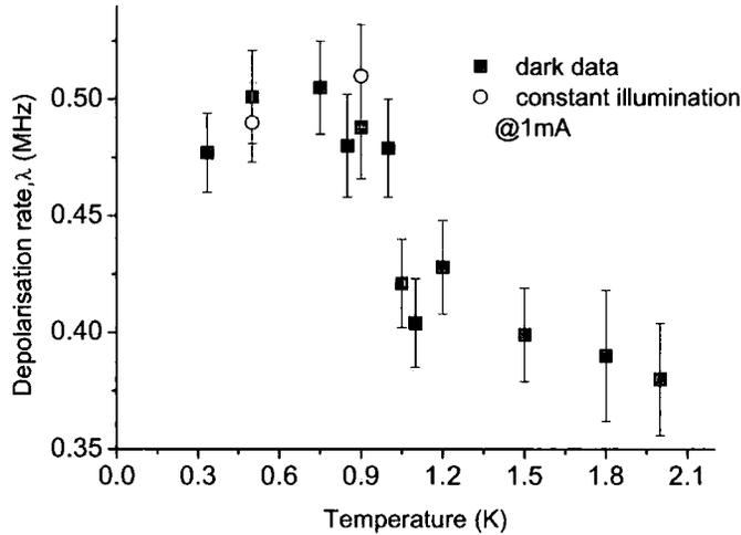
Figure 6.15: The temperature dependent depolarisation rate ( $\lambda$ ) of CdMnTe:Al. A clear change in  $\lambda$  is observed at 0.95 K which is coincident with  $T_g$  obtained via bulk magnetic measurements (Fig. 6.11). Continually illuminating the sample did not change the depolarisation rate.
