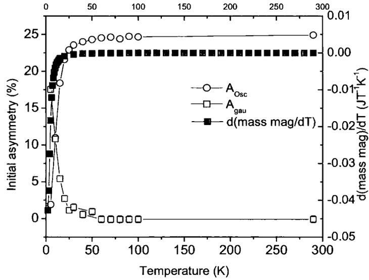
Figure B.5: Temperature dependence of the initial asymmetry of the fitting parameters identified in equation B.1  $A_{Osc}$  and  $A_{gau}$  and the derivative of the mass magnetisation with respect to temperature.
