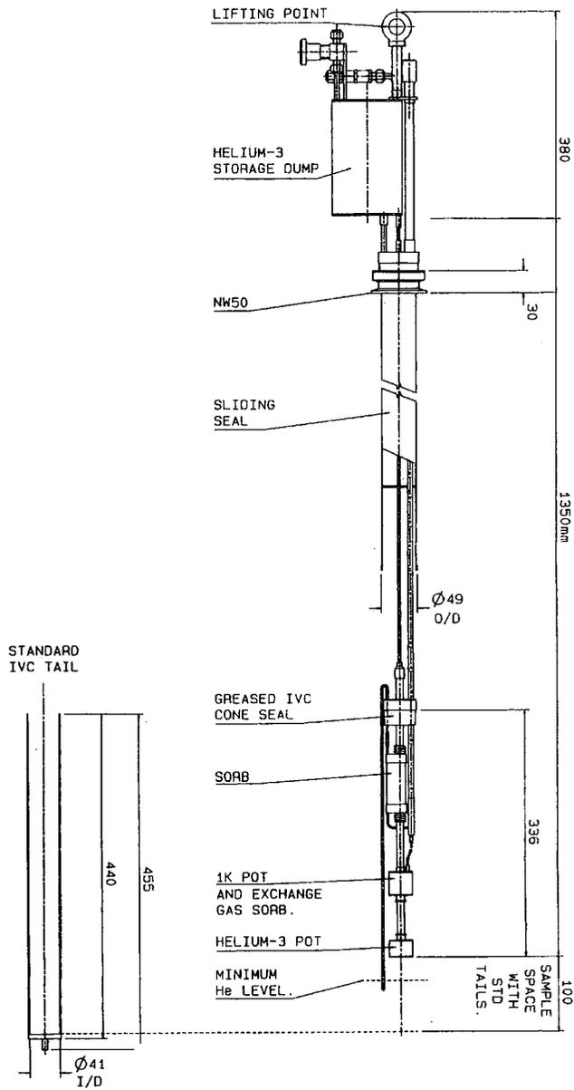
Figure 3.5: A schematic diagram of the Oxford Instruments He<sup>3</sup> Heliox cryostat, all dimensions are in mm.
