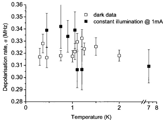
Figure 6.16: The depolarisation rate ( $\sigma$ ) of CdMnTe:In is shown through the spin glass transition identified by bulk magnetic measurements, Fig. 6.12. Data prior to illumination and during constant illumination is shown with  $T_g$  only visible under constant illumination.
