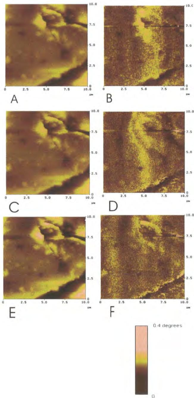
Figure 7.12: AFM images ( A, C, E ) and MFM ( B, D, F ) of PANiCNQ sample 3b<sub>1</sub> after the uv induced magnetic transition.
