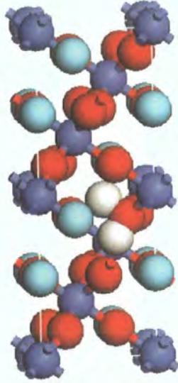
Figure 4.7: Two possible interstitial sites are shown in a  $\text{LaCoO}_3$  “supercell”. The Co ions are represented by the blue spheres, La by the turquoise spheres, O by the red spheres and muons by the white spheres.
