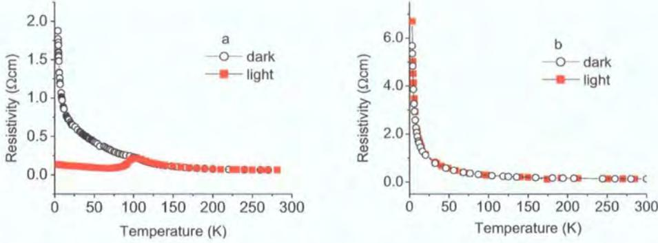
Figure 6.8: Temperature dependent electrical resistivity measurements of  $Cd_{0.85}Mn_{0.15}Te$  doped with In (a) and Al (b) respectively, before and after illumination in an attempt to observe a PPC state.
