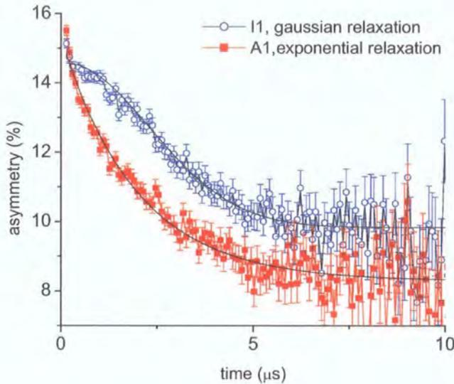
Figure 6.14: The  $\mu SR$  data is shown for both In and Al doped samples prior to illumination, along with their respective fits. The experiments were performed in the zero field configuration at 1.5 K.
