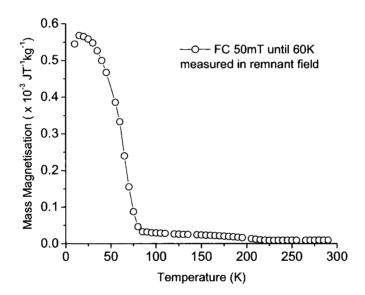
Figure A.12: The temperature dependence of the remnant mass magnetisation of  ${\rm LaCoO_3}$  when field cooled until 60 K and then measured in the remnant field.
