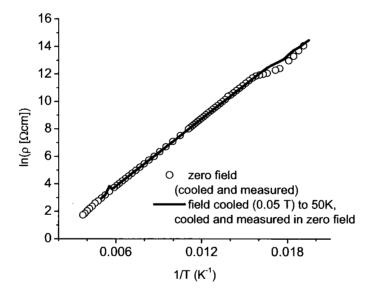
Figure 4.30: Temperature dependence of the zero field resistivity compared directly to when the sample is field cooled. The functional form of the FC data undergos a smaller change in activation energy at 64 K.
