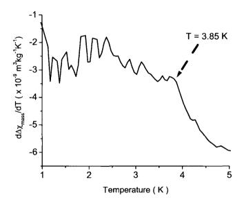
Figure 5.14: Temperature dependent change in derivative of the magnetic susceptibility (ZFC) with respect to temperature for La<sub>0.97</sub>Sr<sub>0.03</sub>CoO<sub>3</sub>.
