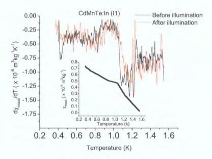
Figure 6.12: Magnetic susceptibility as a function of temperature for  $Cd_{0.85}Mn_{0.15}Te:In$ . The main figure shows the derivative of the moment with respect to the temperature before and after illumination. The inset shows the mass susceptibility before illumination. From [1].
