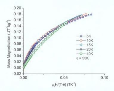
Figure B.4: Mass magnetisation curves for  $La_{0.97}Sr_{0.03}CoO_3$  up to 5 T, demonstrating scaling behavior from 5 K - 20 K.
