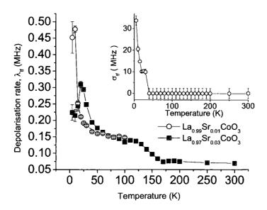
Figure 5.5: Temperature dependence of the depolarisation rates for  $La_{0.97}Sr_{0.03}CoO_3$  and  $La_{0.99}Sr_{0.01}CoO_3$  obtained from the oscillatory component in equation 5.2. The inset demonstrates the temperature dependent gaussian relaxation for  $La_{0.97}Sr_{0.03}CoO_3$ . The lines are a guide to the eye.
