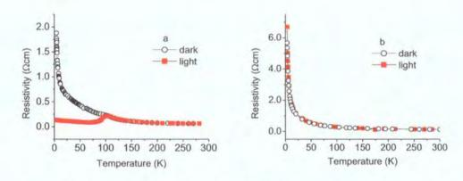
Figure 6.8: Temperature dependent electrical resistivity measurements of  $Cd_{0.85}Mn_{0.15}Te$  doped with In (a) and Al (b) respectively, before and after illumination in an attempt to observe a PPC state.
