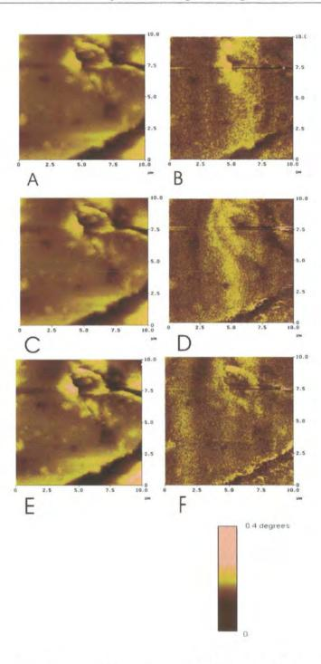
Figure 7.12: AFM images ( A, C, E ) and MFM ( B, D, F ) of PANiCNQ sample  $3b_1$  after the uv induced magnetic transition.
