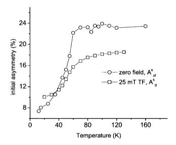
Figure A.11: Temperature dependence of the initial asymmetry parameters for the ZF and 25 mT TF data as defined in A.2 and A.1.
