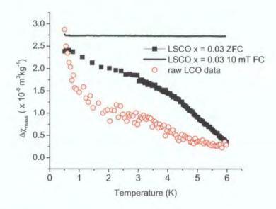
Figure 5.13: Temperature dependent change in magnetic susceptibility of La<sub>0.97</sub>Sr<sub>0.03</sub>CoO<sub>3</sub>, for both FC and ZFC experiments, directly compared to the raw data of LaCoO<sub>3</sub>, from chapter 4.
