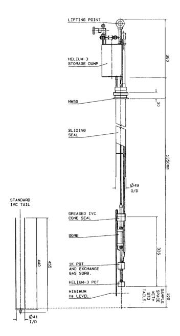
Figure 3.5: A schematic diagram of the Oxford Instruments  $\mathrm{He^3}$  Heliox cryostat, all dimensions are in mm.
