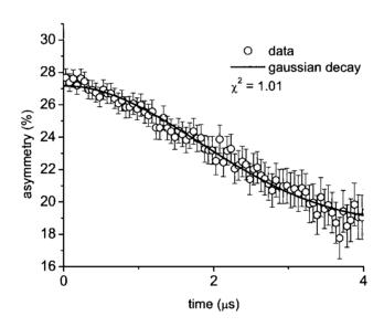
Figure A.6: Time dependence of the fitting function and the data for the ZF data at 100 K, with the gaussian term of equation A.2
