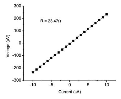
Figure 3.1: A VI plot showing good Ohmic behaviour. This particular sample of  $La_{0.85}Sr_{0.15}CoO_3$  was measured at 14 K, the error bars are within the symbols.
