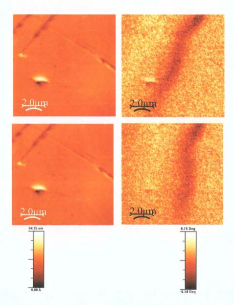
Figure C.4: AFM (on the left) and MFM ( on the right ) images of a sample of PANiCNQ.
