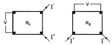
Figure 3.2: The van der Pauw technique; this diagram shows the perimeter current and voltage taps for the resistance configurations to calculate the resistivity.
