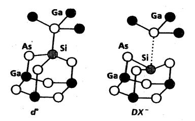
Figure 6.3: Atomic configuration of the shallow donor (d<sup>0</sup>) and the deep DX<sup>-</sup> level in  $Al_xGa_{1-x}As$ :Si, showing the distortion of the lattice around the donor atom Si[12, 13]
