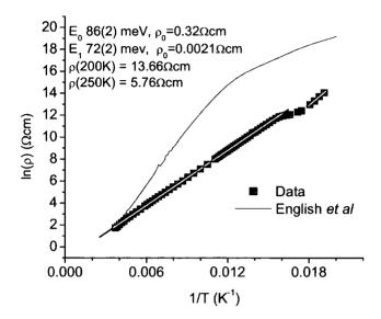
Figure 4.29: Temperature dependence of the zero field resistivity. The functional form of the data is clearly activated with a high temperature activation energy  $E_0$  of 86 meV with a crossover to  $E_1$  of 72 meV at 64 K. Also shown are the resistivity data from English *et al*[29].
