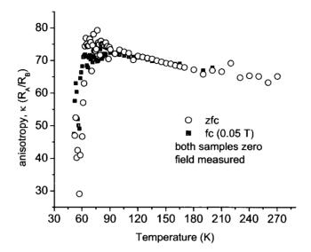
Figure 4.31: Temperature dependence of the anisotropy ratio ( $\kappa$ ) for both the FC and ZFC data, a clear change in the anisotropy ratio is seen in both scenarios below 64 K.
