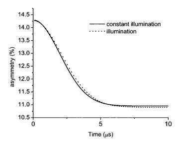
Figure 6.17: The time dependent change in the muon relaxation for  $Cd_{0.85}Mn_{0.15}$ Te:In in the dark and under constant illumination, the change in observed relaxation is very small at 0.9 K.
