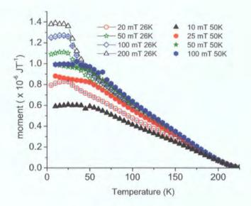
Figure 5.11: Temperature dependence of the remnant magnetic moment of  $La_{0.97}Sr_{0.03}CoO_3$  when field cooled in various field until 26 K (hollow symbols) and 50 K (filled symbols).
