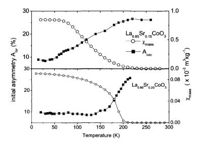
Figure 5.16: Temperature dependence of the initial asymmetry directly compared to the FC mass susceptibility of  $La_{0.85}Sr_{0.15}CoO_3$  and  $La_{0.80}Sr_{0.20}CoO_3$  respectively. The errors are smaller than the symbols.
