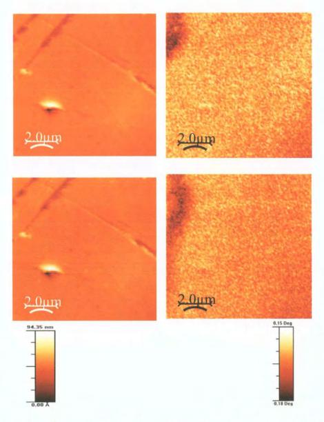
Figure C.2: AFM (on the left) and MFM ( on the right ) images of a sample of PANiCNQ.
