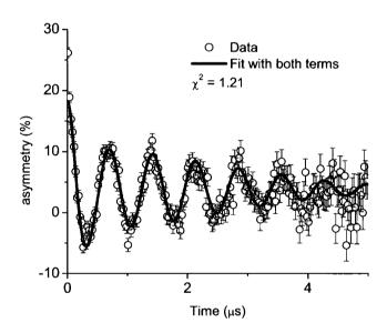
Figure B.3: Time dependence of the fitting function and the data for the TF data at  $20~\mathrm{K}$ , with both terms of equation B.1
