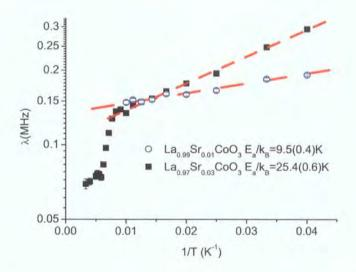
Figure 5.6: Inverse temperature dependence of the depolarisation rates for  $La_{0.97}Sr_{0.03}CoO_3$  and  $La_{0.99}Sr_{0.01}CoO_3$  obtained from the oscillatory component in equation 5.2.
