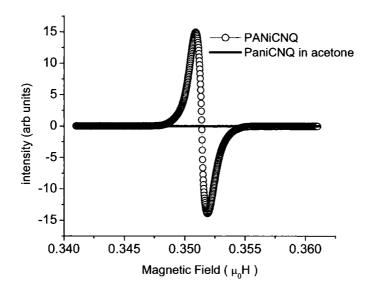
Figure 7.14: ESR signal of sample 3b<sub>1</sub>, before and after dissolving in acetone.
