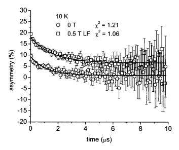
Figure 5.9: Asymmetry comparison of  $La_{0.97}Sr_{0.03}CoO_3$  at 10 K in both the ZF configuration and in an external LF of 0.5 T.
