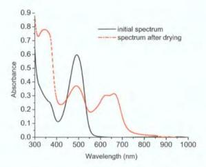
Figure 7.7: Optical absorption of PANiCNQ before and after drying, showing intremolecular charge transfer has occurred.
