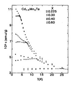
Figure 6.6: Temperature dependent magnetic susceptibility, for varying values of the composition x. Both FC (solid symbols) and ZFC (open symbols) are shown indicating a cusp in the susceptibility indicative of the SG transition. From [21].
