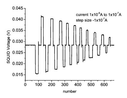
Figure 3.7: The response of the SQUID to a change in current of an electromagnet wrapped around the sample holder. The current was applied in both directions and stepped uniformly down in 10 steps from  $1\mu$ A to  $0.1 \mu$ A.
