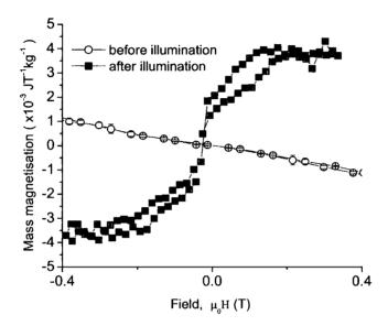
Figure 7.11: The field dependent magnetisation of sample 3b<sub>1</sub> before and after irradiation with uv light.
