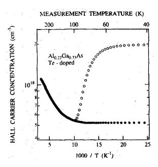
Figure 6.2: The temperature dependent carrier density in Al<sub>0.27</sub>Ga<sub>0.73</sub>As:Te is shown for both dark data (closed symbols) and illuminated data, reproduced from [5]
