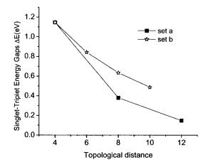
Figure 7.4: The singlet triplet energy gap for biradicals as a function of topological distance for set a and b. From [18].
