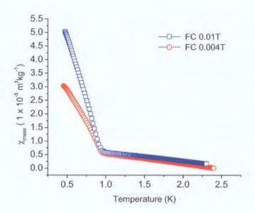
Figure 6.11: The temperature dependent magnetic susceptibility of  ${\rm Cd_{0.86}Mn_{0.14}Te:Al}$  (A1), cooled in an external field of 0.01 T and 0.004T, then measured in a field of 10  $\mu$ T.
