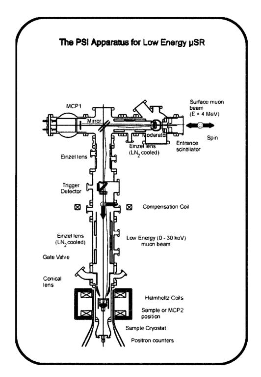
Figure 3.12: The LEM beamline at the PSI. The apparatus enables muons with an incoming energy of  $\sim 4$  MeV to be tuned to have energies between 0.5 and 30 keV[10].
