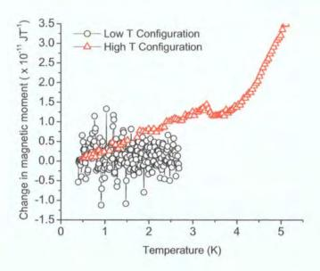
Figure 3.9: Temperature dependent change in the magnetic moment of the background for the temperature regions, 350 mK < T < 2.5 K (low temperature configuration) and 1 K < T < 5 K (high temperature configuration). The measuring field in both cases was 10  $\mu$ T.
