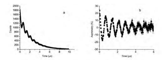
Figure 3.11: Time dependent positron detection for La<sub>0.85</sub>Sr<sub>0.15</sub>CoO<sub>3</sub>. (a) The response of the forward detector to the muon decay in a TF experiment of 0.01 T. (b) A typical asymmetry spectrum denoted by equation 3.3 for the same TF as (a).
