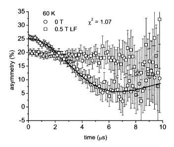
Figure 5.7: Asymmetry comparison of La<sub>0.97</sub>Sr<sub>0.03</sub>CoO<sub>3</sub> at 60 K in both the ZF configuration and in an external LF of 0.5 T.
