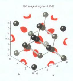
Figure 6.13: The muon implantation site probability distribution as a function of the unit cell  $(\mathring{A})$ , the implanted muons are predicted to sit at an interstitial site, an overlay of the crystal structure is shown for comparison.
