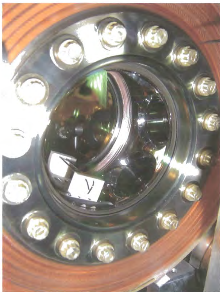
Figure 4.6: Photograph showing the position of the dispensers in the vacuum system. The dispensers are the silver strips in the lower left of the large view-port. The wires over the dispensers are to prevent a direct line of light from the thermal source to the MOT.
