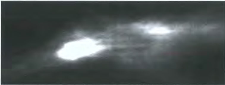
Figure 7.3: Screen captures of images taken during alignment of the \text{CO}_2 laser with the MOT using the anti-trapping technique. The \text{CO}_2 laser can be seen as a dark stripe through the centre of the image.
