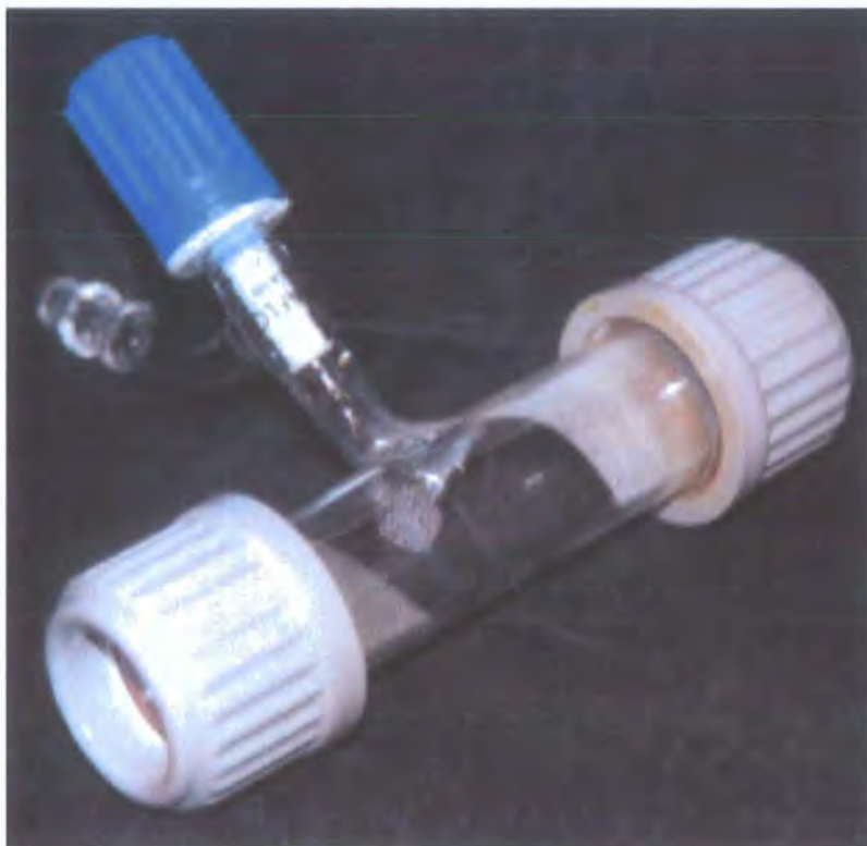
Figure 8.8: The glass cell after use for UV-Vis BPEB measurements, the white substance on the walls of the cell is re-condensed BPEB. The clear parts of the cell indicated where the heater was attached, and prevented the BPEB from condensing.
