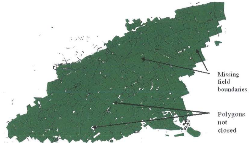
Figure 5.5 Polygon errors from feature code 0030
