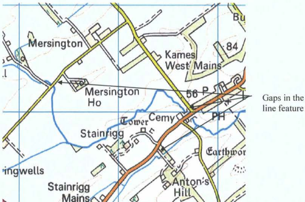
Figure 5.7 Example of errors that carry over to automated digitising
