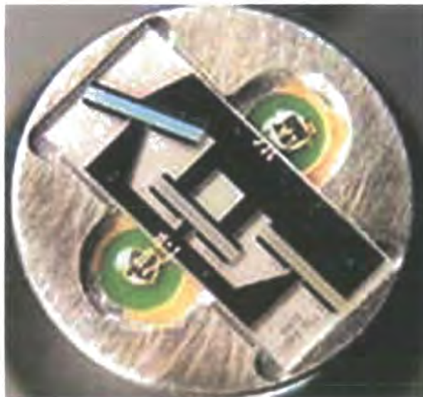
Figure 3-20. Tyre pressure monitoring device using three SAW delay lines (Transense Technologies PLC).
