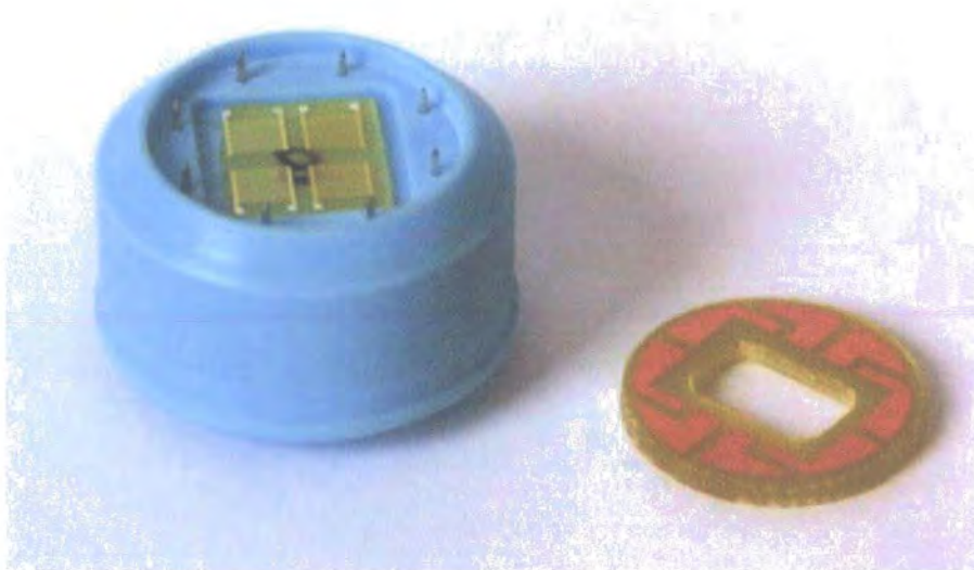
Figure 8-14. Component parts of prototype package. The sensor die is positioned in the case, surrounded by 8 spring-loaded pins. The copper tracks on the PCB allow contact between the pins and contact pads on the die.
