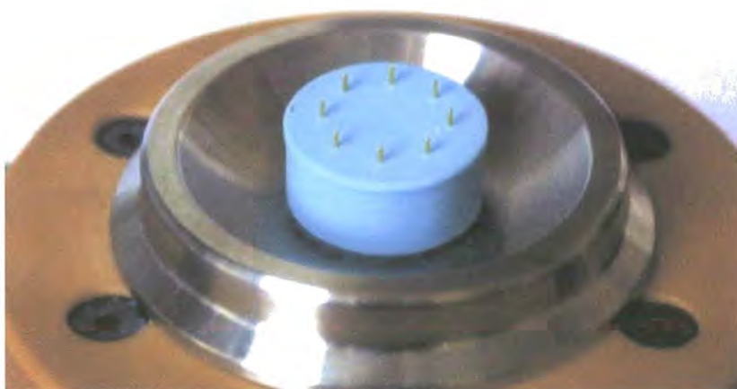
Figure 8-16. Prototype package in sample chamber. The pins would locate in a socket in the lid.
