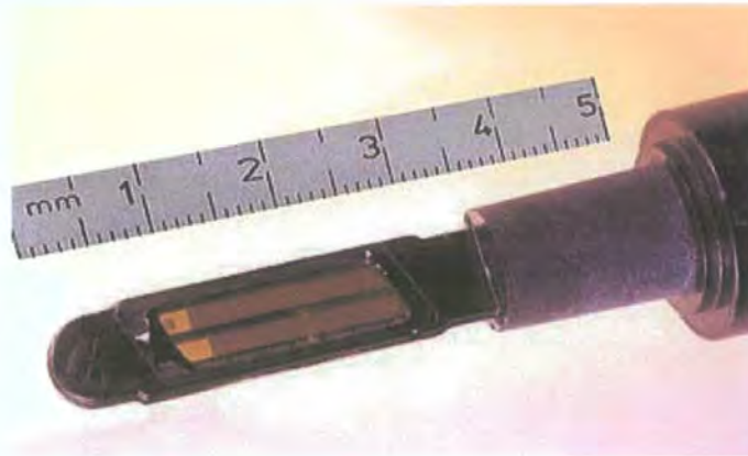
Figure 8-21. Dip-stick viscometer using a SAW device for oil quality measurements [129].
