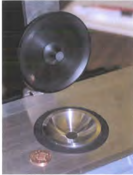
Figure 8-4. Refractometer sample chamber. The stainless steel bowl with the central window region is positioned towards the bottom of the picture, and the lid with the central stub is in the vertical open position. The UK one-penny coin has a diameter of 20 mm for comparison.
