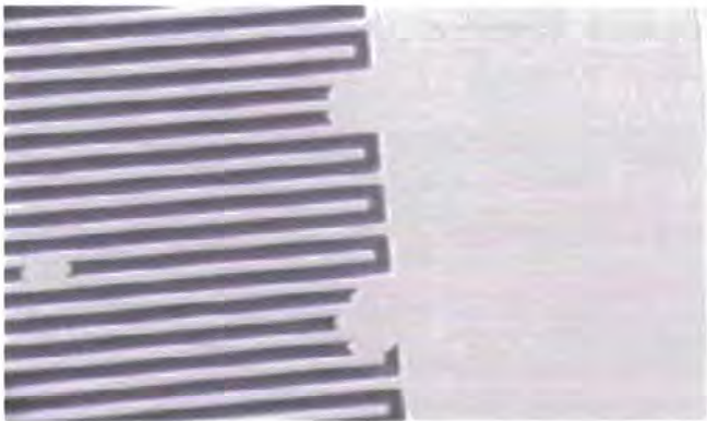
Figure 4-9. Al spots resulting from H 2 bubbles forming during Al etching, causing short-circuits.
