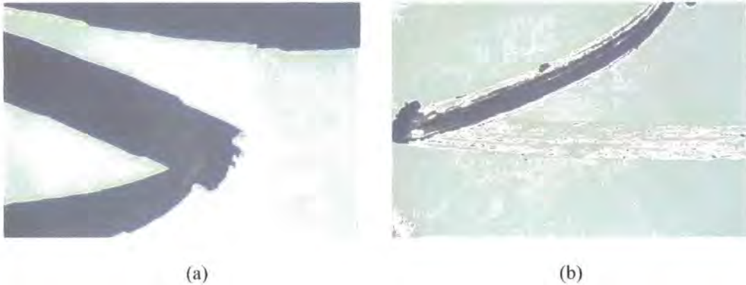
Figure 4-8. (a) Completely removal of the Al on the un-annealed sample and (b) only partial removal due to improved adhesion with annealing.
