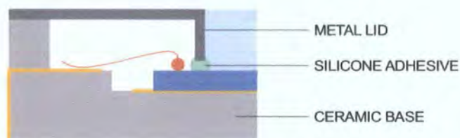
Figure 8-6. Method of sealing electrical contacts using a metal lid and ceramic base. The ceramic package is based on the electrical header illustrated in figure 8-2.
