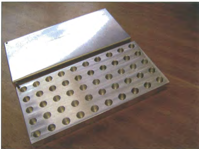
Figure 3.12 Sample block for annealing in vacuum oven
