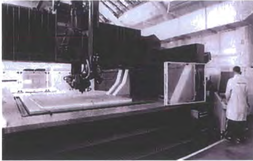
Figure 7.8. An Example Resource: the Desitech Panel Machining Centre.
