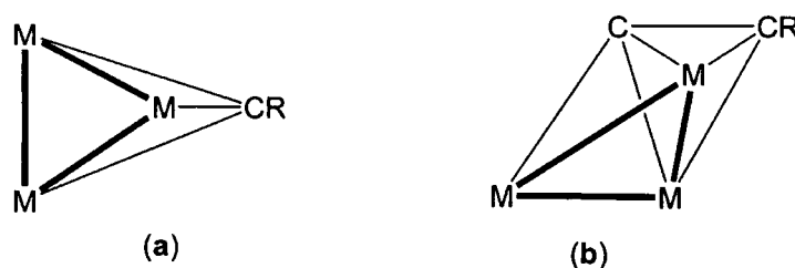
Figure 1.7. The attachment of terminal carbon to the metal atoms by (a) \mu_3\text{-}\eta^1 mode and (b) \mu_3\text{-}\eta^3 .
