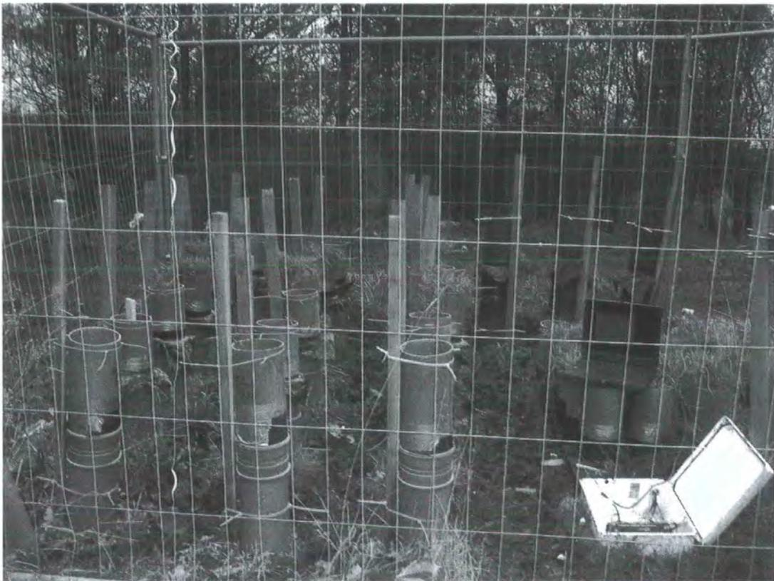
**Photograph 2.2: Field Lysimeter set up at Thornley**
