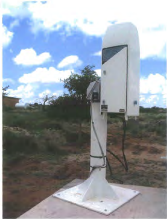
Figure 3.17: The ceilometer used to measure the backscatter of radiation at 905 nm.
