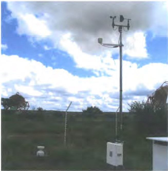
Figure 3.3: The weather station pole on site, which measures the air temperature and pressure, relative humidity, and wind speed at ground level.
