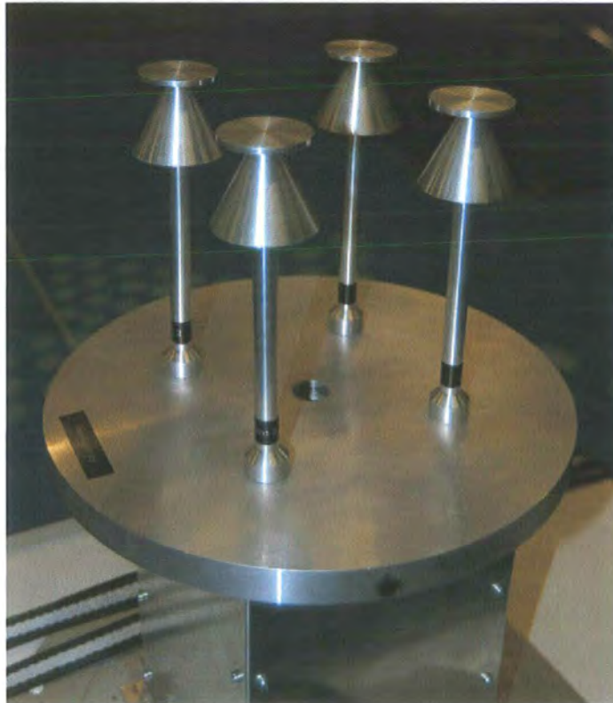
Figure 6.27: Wideband (2-6 GHz) Discone circular array (showing 4 elements) [28].
