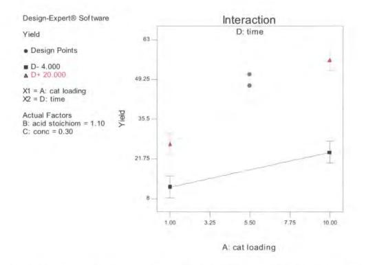
Figure 11. Catalyst loading/time interaction graph for the boric acid catalysed direct amide condensation in toluene.
