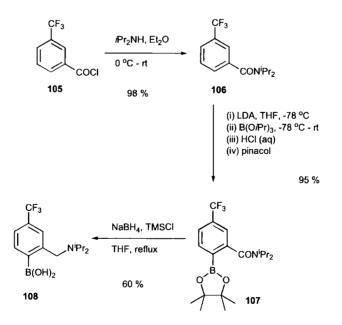
Scheme 7. Synthesis of trifluoromethyl-substituted boronic acid 108.
