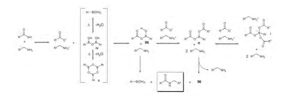
Scheme 5. Proposed mechanism for amide formation catalysed by boric or boronic acids.
