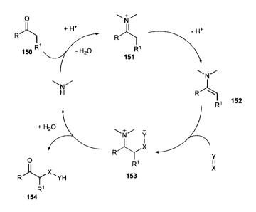
Scheme 12. Proposed mechanism for enamine catalysis.
