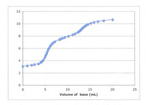
Figure 23. Titration curve for (S)-pyrrolidin-2-yl-methylboronic acid 268a with sodium hydroxide in H<sub>2</sub>O.
