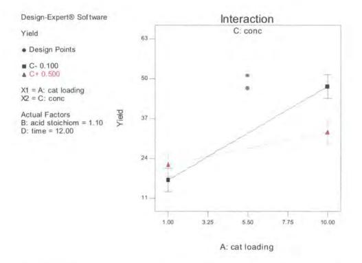
Figure 10. Catalyst loading/concentration interaction graph for the boric acid catalysed direct amide condensation in toluene.
