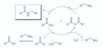
Scheme 4. Proposed mechanism for thermal amide formation.
