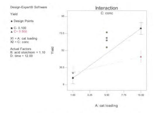
Figure 8. Interaction graph for the direct amide condensation in toluene.
