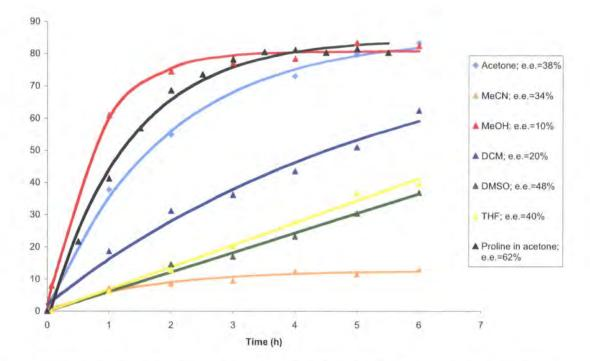
Figure 25. Solvent effects on conversion to aldol adduct (S)-278 vs. time for the reaction between 4-nitrobenzaldehyde and acetone catalysed by (S)-268a
