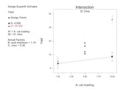
Figure 6. Interaction graph for the direct amide condensation in fluorobenzene.
