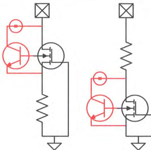
Figure 5.39: Extended source and extended drain ggNMOS schematic
