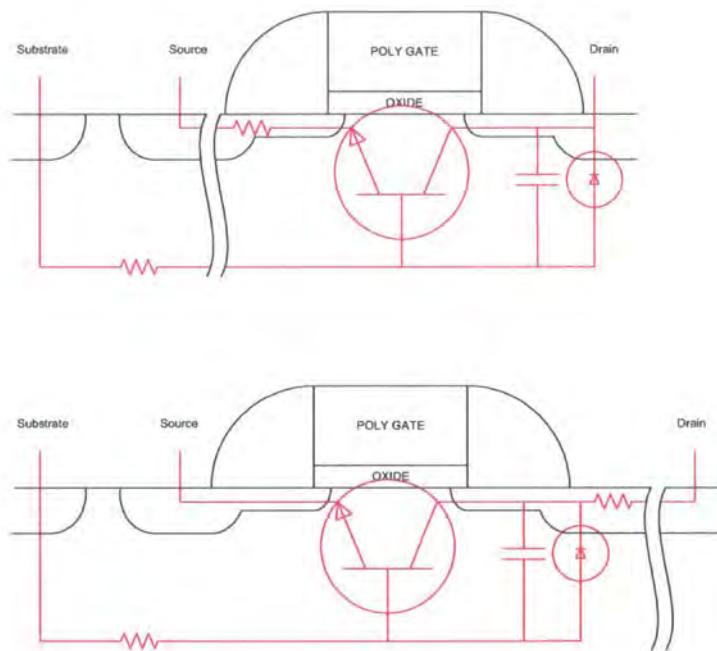
Figure 5.40: Extended source and extended drain ggNMOS layout
