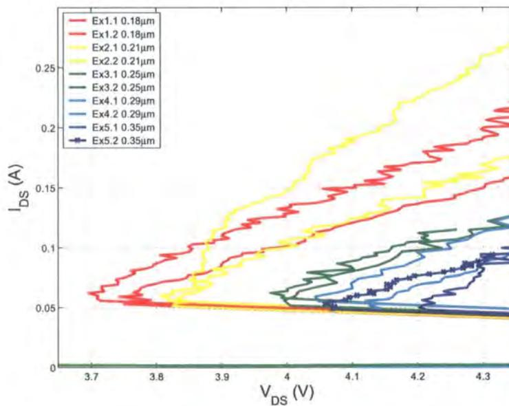
Figure 6.7: Detail of Figure 6.6 showing ggNMOS once triggered
