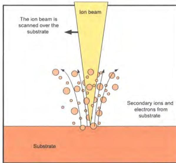
Figure 3.2: The principle of FIB imaging [4]
