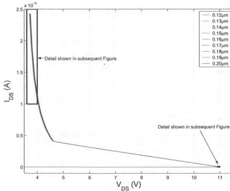
Figure 6.12: IV characteristics of a modified ggNMOS
