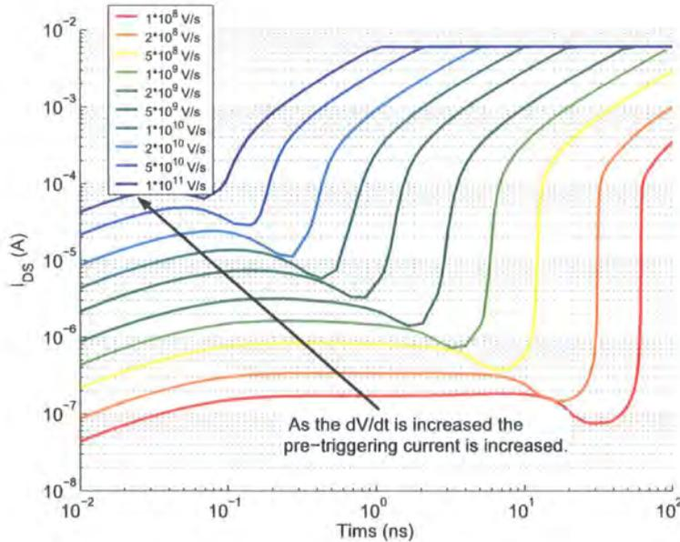
Figure 5.23:  $I_{DS}$  vs Time over a range of applied voltage ramps
