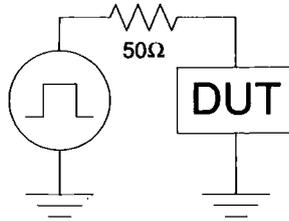
Figure 2.1: The basic concept of a TLP tester
