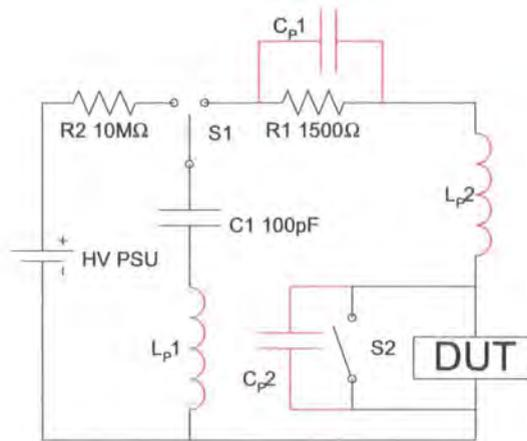
Figure 1.47: HBM ESD test circuit with parasitics
