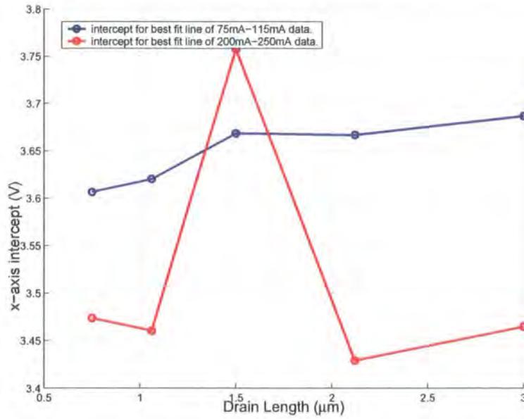
Figure 6.17: The offset voltage of the ggNMOS once the device is triggered over a range of drain lengths
