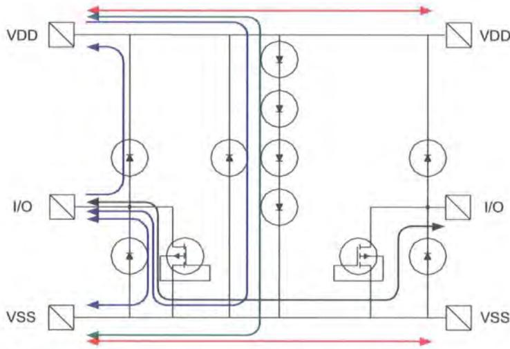
Figure 1.44: Current paths through a chip for all pin discharge combinations
