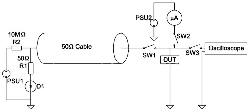
Figure 2.11: TLP tester schematic
