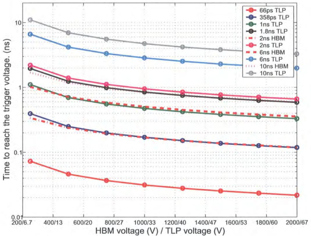
Figure 4.2: The time taken for an HBM or TLP source to reach 6V for a variety of rise times and amplitudes
