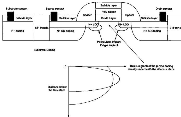
Figure 5.9: The structure of an nMOS transistor
