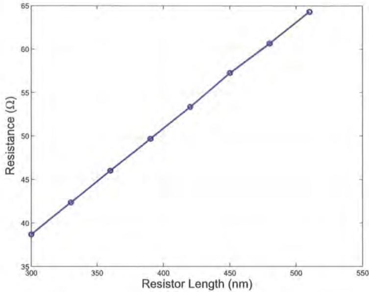
Figure 5.38: Resistance of the n-well resistors vs length
