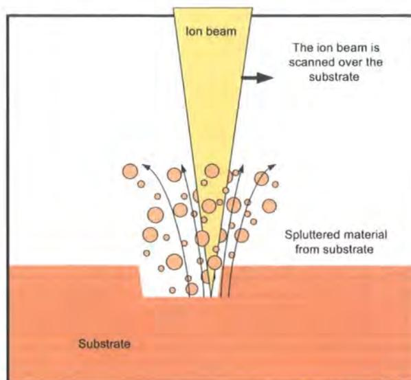
Figure 3.3: The principle of FIB milling [4]
