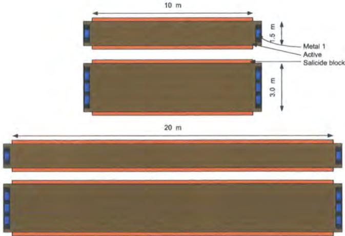
Figure 6.25: Layout of the test resistors
