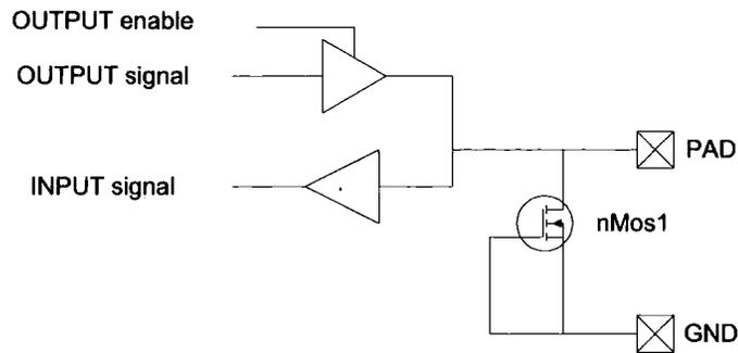
Figure 1.1: An IO circuit with ESD protection
