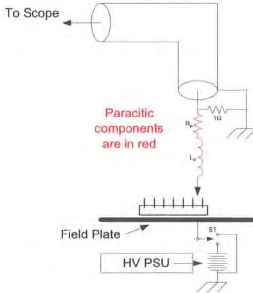
Figure 1.50: CDM ESD test circuit with parasitics
