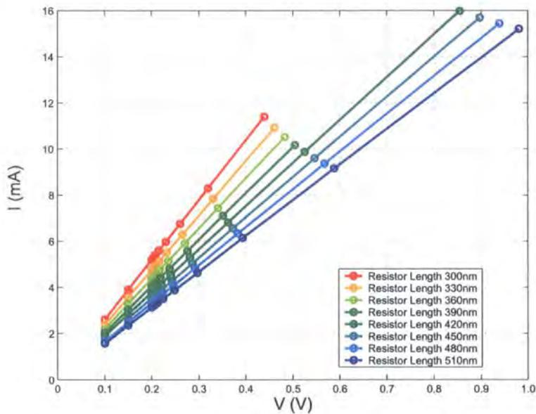
Figure 5.37: IV characteristics of an n-well resistor
