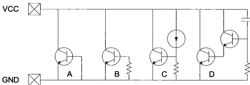
Figure 1.15: Three ESD protection solutions using bipolar transistors
