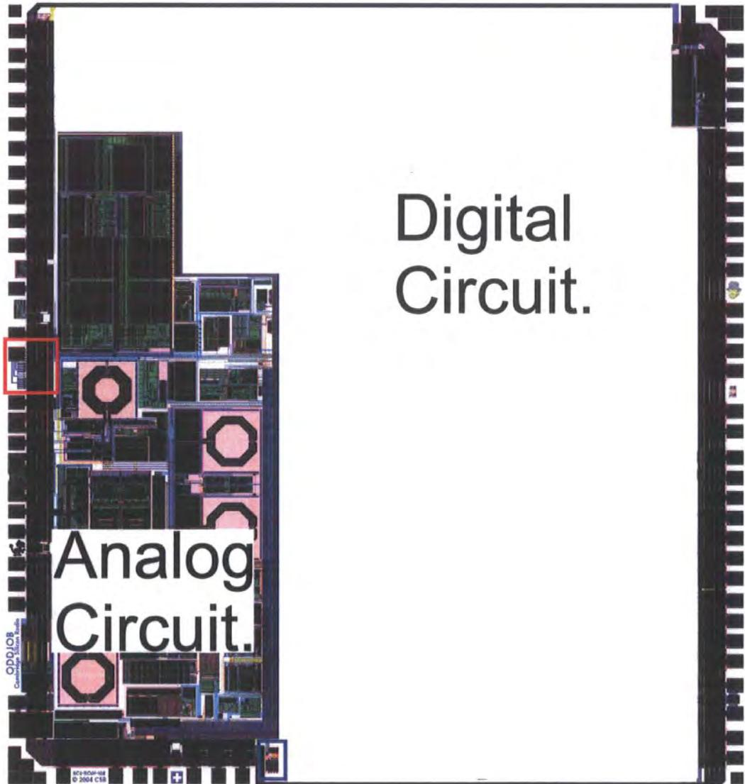
Figure 6.1: Top level layout of the CSR chip
