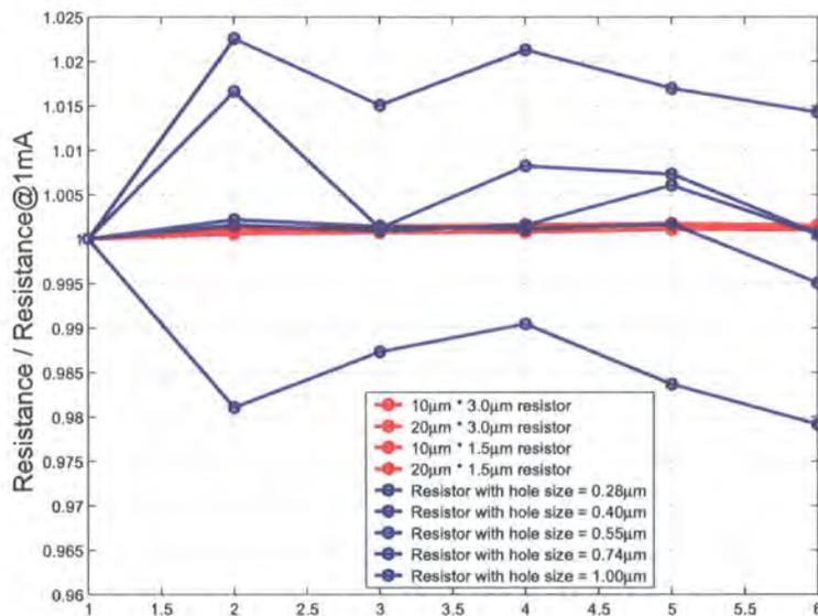
Figure 6.22: Change in measured Resistance vs Current
