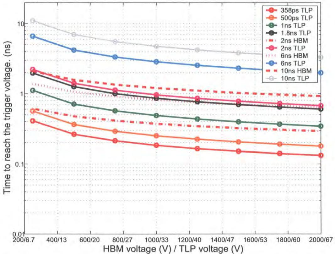
Figure 4.4: The time taken for a ggNMOS  $V_{DS}$  to reach 6V under TLP and HBM test conditions for a variety of rise times and amplitudes
