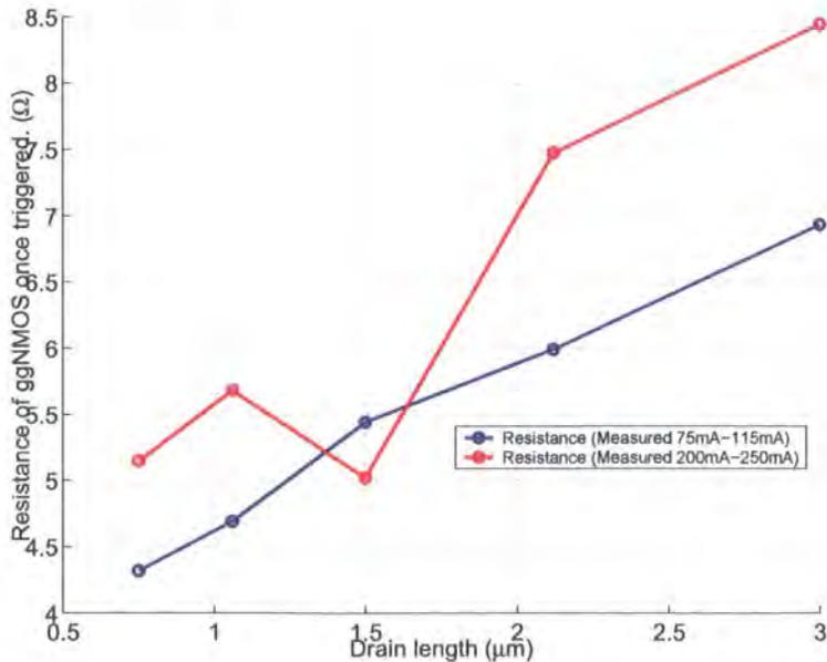
Figure 6.16: The resistance of the ggNMOS once the device is triggered over a range of drain lengths
