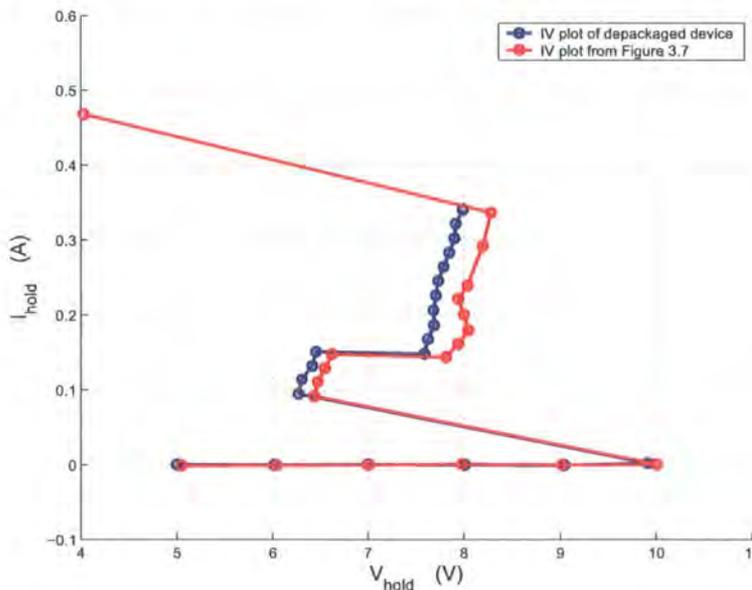
Figure 3.10: IV plot of a depackaged device
