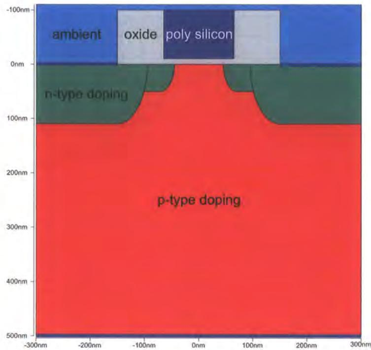
Figure A.1: An un-simulated transistor structure
