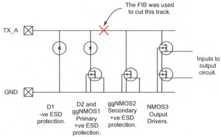
Figure 3.13: The position of the FIB cut to remove ggNMOS2 and the output drivers
