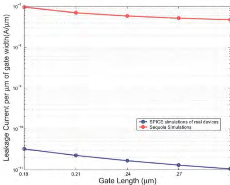
Figure 6.10: Comparison of the leakage current of a ggNMOS calculated using SPICE and Finite Element Simulation
