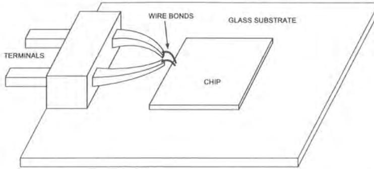
Figure 3.9: Depackaged chip mounted on a glass substrate
