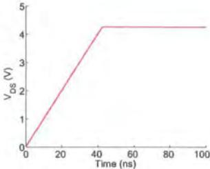
Figure 5.24:  $10^8 \text{V/s}$  voltage ramp with a voltage limit of  $4.25 \text{V}$
