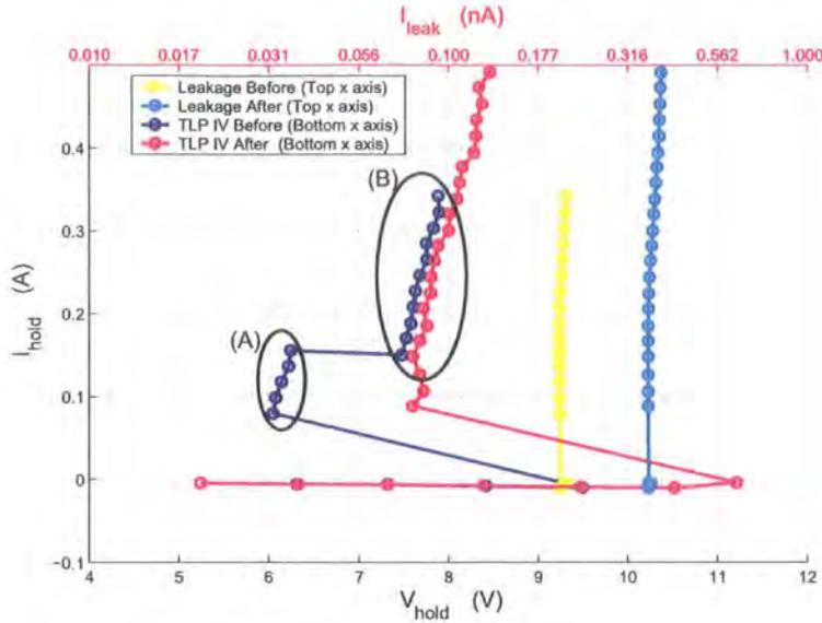
Figure 3.19: TLP IV curve of TX\_A before and after ggNMOS2 and the output drivers were removed (second sample)
