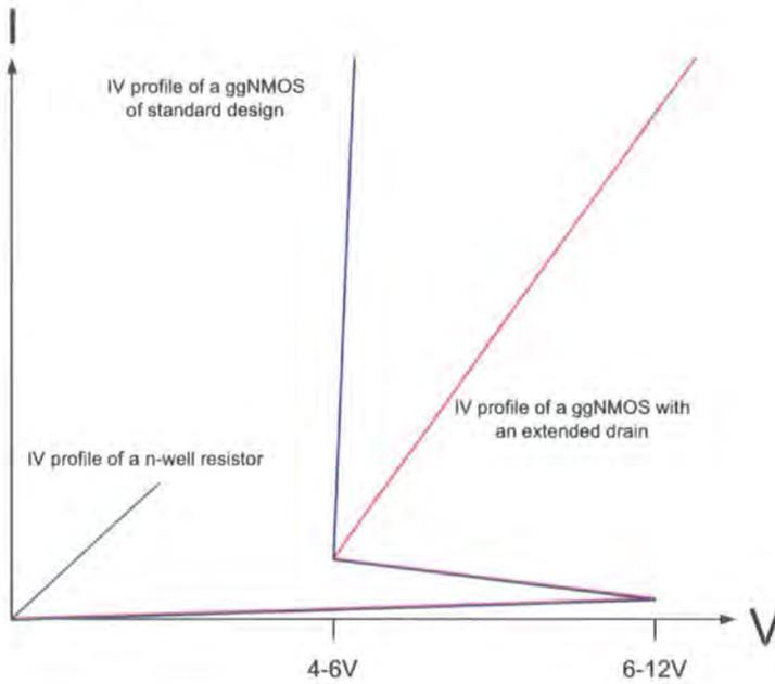
Figure 1.34: The IV profile of an unmodified and modified (drain extended) ggNMOS silicon area consumed by the ggNMOS as well as the parasitic capacitance and alter the triggering voltage of the device whilst maintaining a high  $I_{t2}$ .
