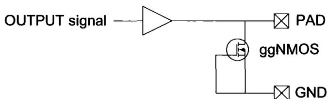
Figure 1.32: Basic ggNMOS design using a standard nMOS
