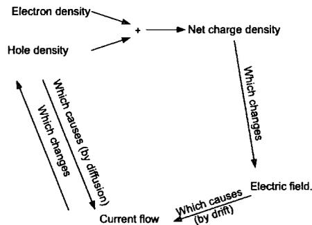
Figure 5.1: The calculations that the Finite Element Simulation software has to satisfy in order for the simulation to converge
