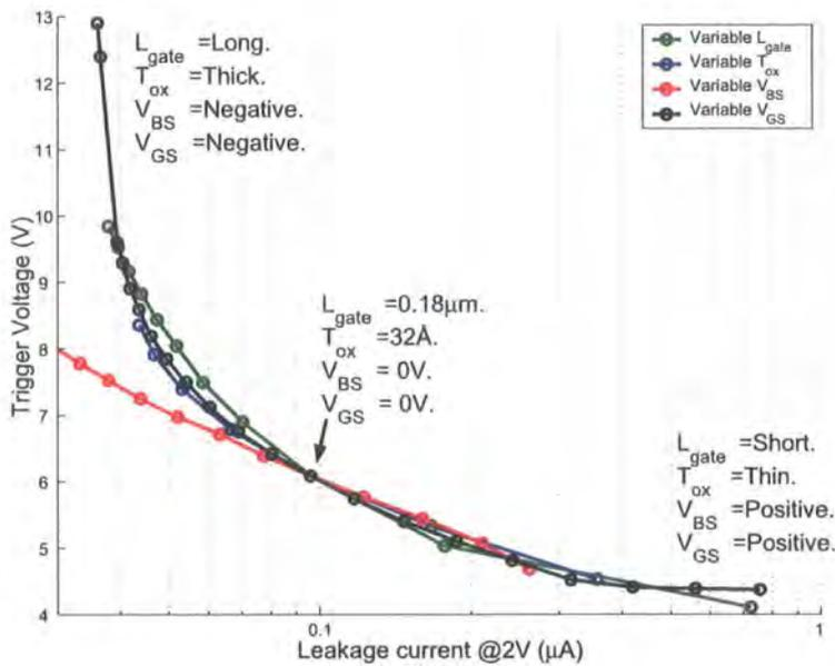
Figure 5.21:  $V_{t1}$  vs  $I_{leak}$  over a range of gate lengths, oxide thicknesses, gate biases and bulk biases
