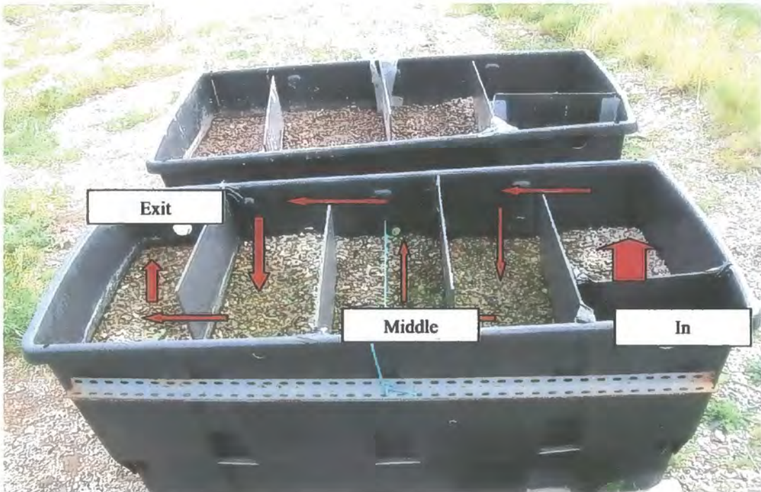
Plate 2.3. Photograph of a spare test tank complete with baffles and gravel showing sample points and direction of flow. These two beds were later used as gravel only test beds.
