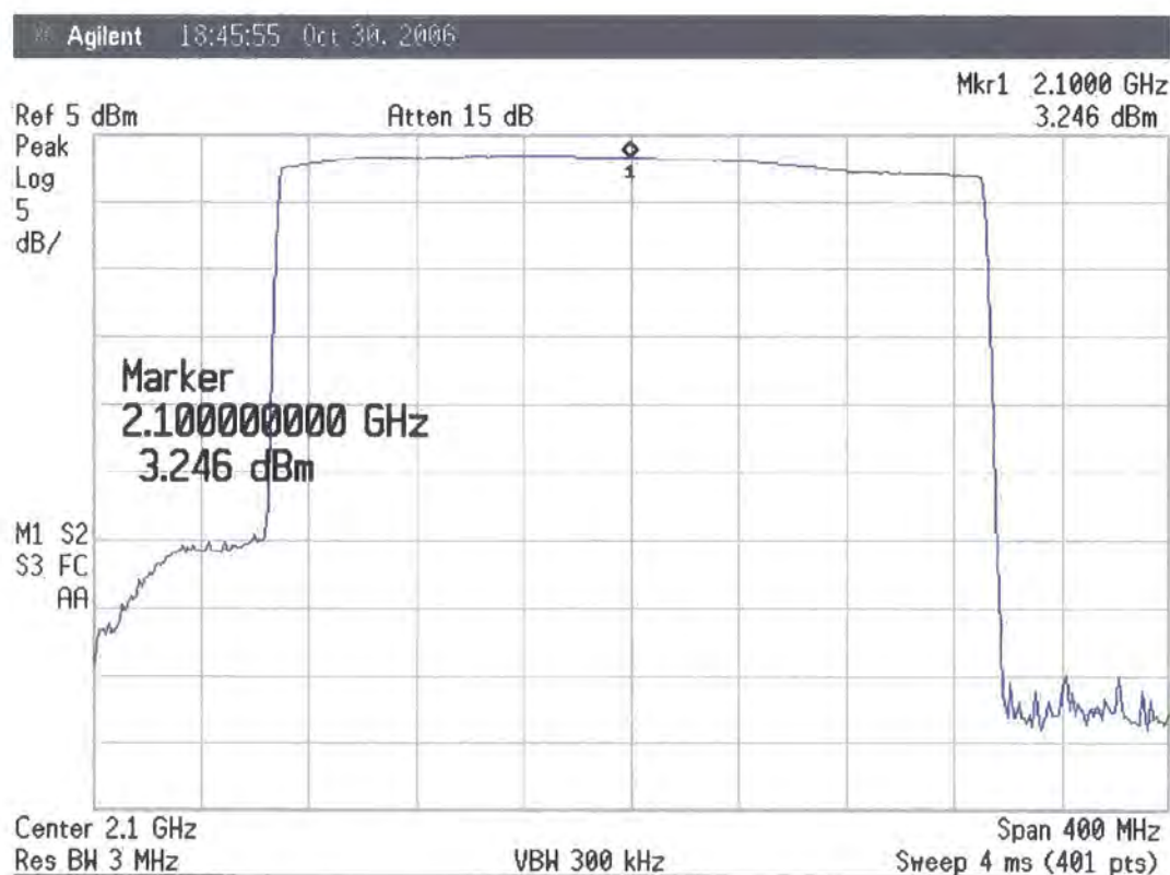
Figure 5.6 2.1 GHz IF flatness for 260 MHz sweep width
