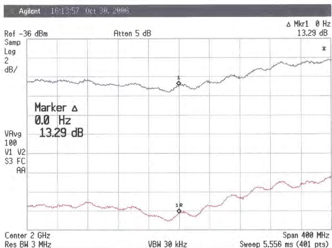
Figure 5.15 “y-factor” measurement of the 3.5 GHz down-converter
