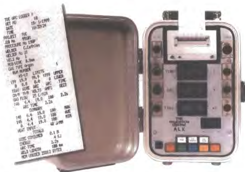
Figure 3.8: PAMS monitoring device and typical sample printout it generates
