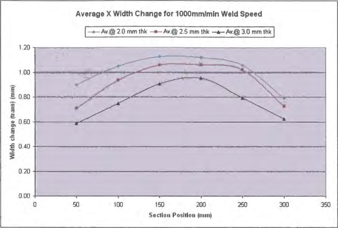
Figure 4.35: Variation of transverse distortion for thickness variation (butt weld)
