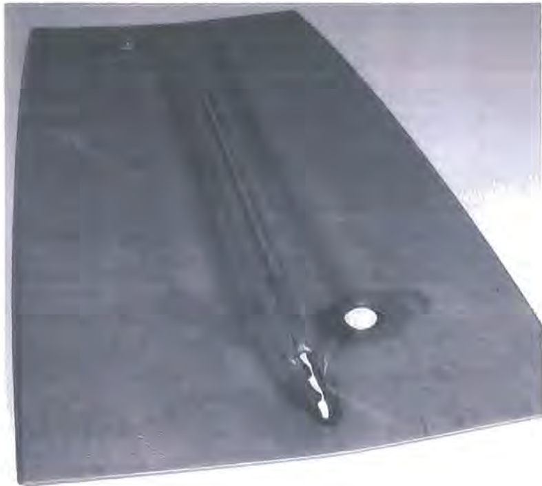
Figure 4.3: Picture of 2.0mm plate showing burn through at end of weld run
