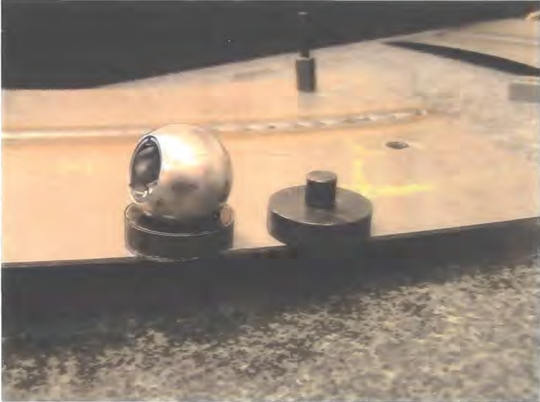
Figure 3.10: Track ball and holders used in scanning process
