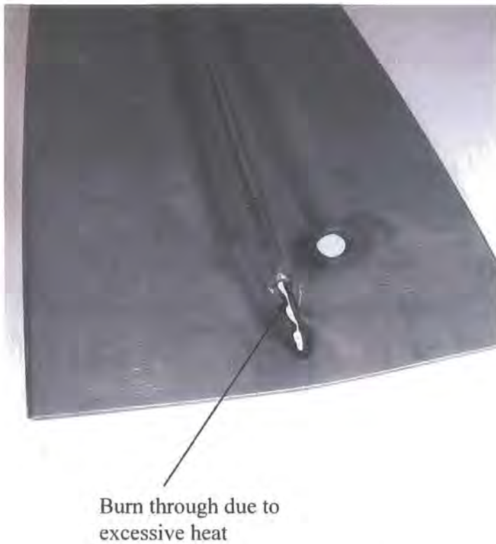
Figure 3.7: Example of burn through due to incorrect weld speed
