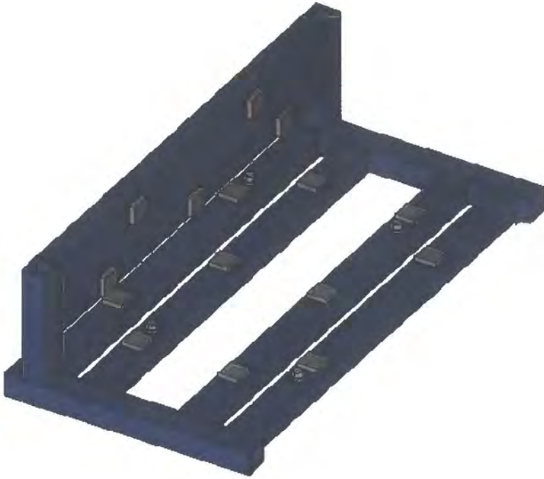
Figure 3.5: Modified final fixture design
