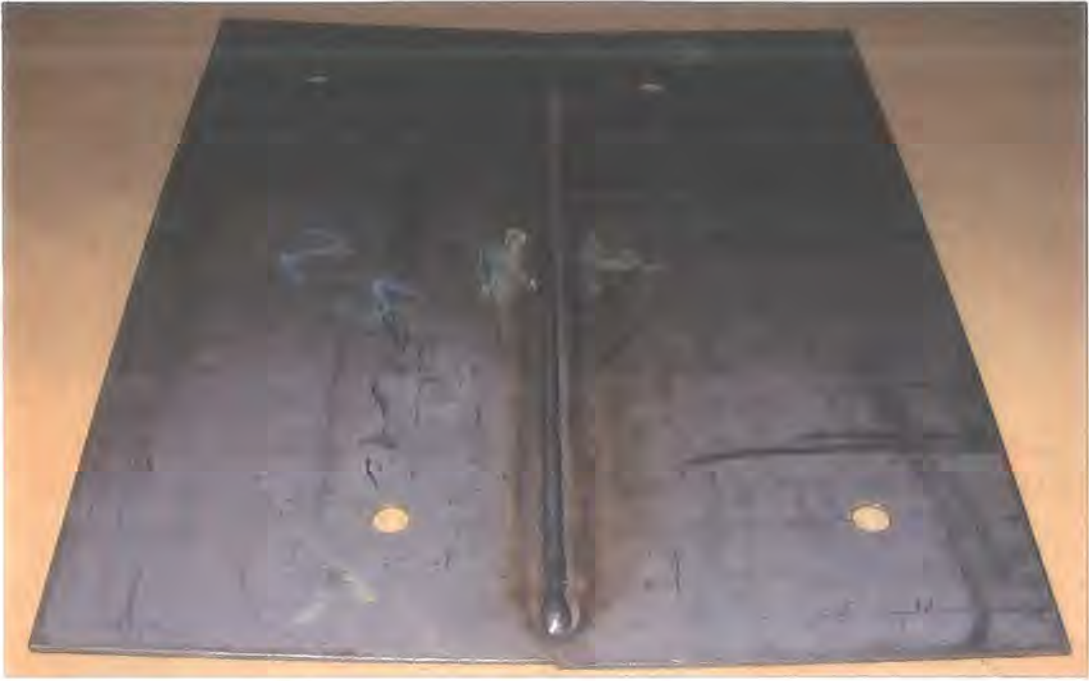
Figure 4.25: Image of a typical welded butt weld sample
