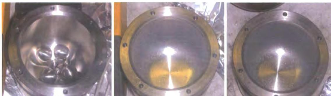
**Figure 5.5** Photographs of 99.8 wt. % titanium pot (inner diameter ~10 cm) used in Fritsch P6 milling: before milling (left) and after 30 mins (centre) and 60 mins (right) of milling  $\text{Nb}_3\text{Sn}$ . For clarity, the 10 mm and 20 mm diameter milling balls are not included in the photos of the pot after milling.
