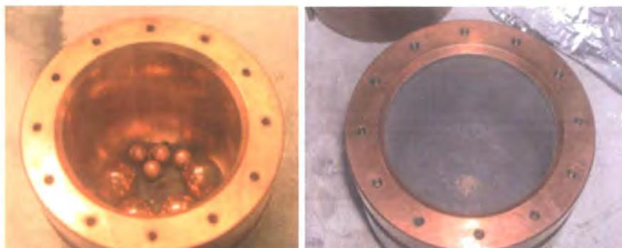
**Figure 5.4** Photographs of 99.95 wt. % copper pot (inner diameter ~10 cm) used in Fritsch P6 milling before milling (left) and after 90 minutes of milling  $\text{Nb}_3\text{Sn}$  (right). In the photo on the left before milling, the loose  $\text{Nb}_3\text{Sn}$  powder can be seen with the clean milling balls of 10 mm and 20 mm diameter. The balls have been taken out of the pot in the photo on the right to show the extent of coating of the pot sides.
