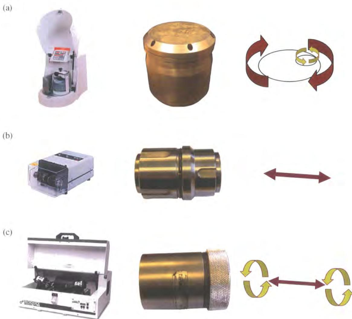
**Figure 3.4** Photographs, milling pots and schematic representation of the milling pot motion for the: (a) Fritsch P6, (b) Retsch MM301 and (c) SPEX 8000D
