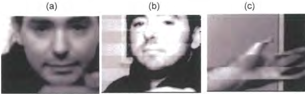
Figure 4.4: Images captured with the successive partial system - (a) shows a normal image of the author taken under natural illumination, whilst (b) shows the striping effects caused by aliasing with the 100Hz mains illumination. Finally (c) shows a tearing effect caused by the motion of a waving hand.
