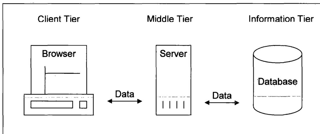
**Figure 1 Three-tier Web based application (From [4])**
