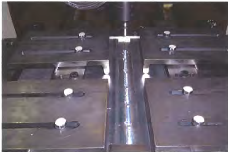
Figure 27 - Clamping Arrangement for Trial 1
