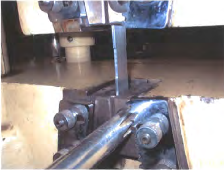
Figure 38 - Testing in Denison Tensile Tester
