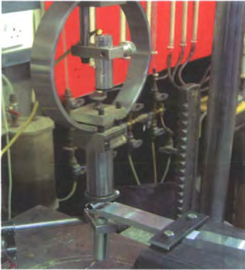
Figure 48 - TRIAL 5 Bending Test Setup
