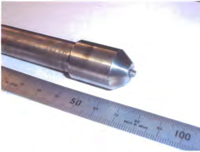
Figure 26 - Screw Type FSW Tool and Holder
