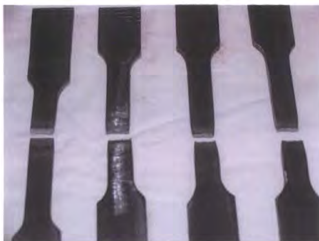
Figure 24 – Steel FSW Tensile Test Specimens
